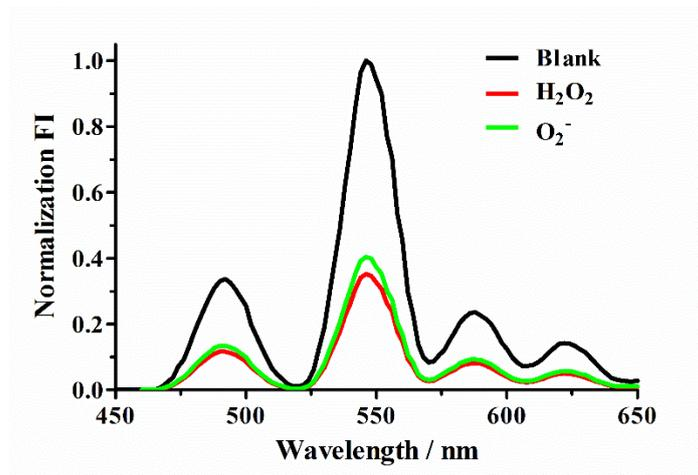
**Figure S6** Luminescence responses of the Tb/GMP/Hg-Cys sensing system to 100  $\mu\text{M}$  ROS including  $\text{H}_2\text{O}_2$  and superoxide free radical ( $\text{O}_2^-$ ).  $\text{O}_2^-$  generated from dissolved  $\text{KO}_2$  (200  $\mu\text{M}$ ) in the dimethyl sulphoxide (DMSO) and the concentration of  $\text{O}_2^-$  was estimated to be the half concentration of  $\text{KO}_2$ .
