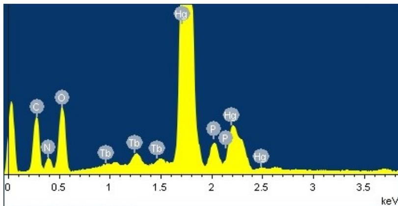
**Figure S2** Energy-dispersive X-ray (EDX) spectra of Tb/GMP/Hg.
