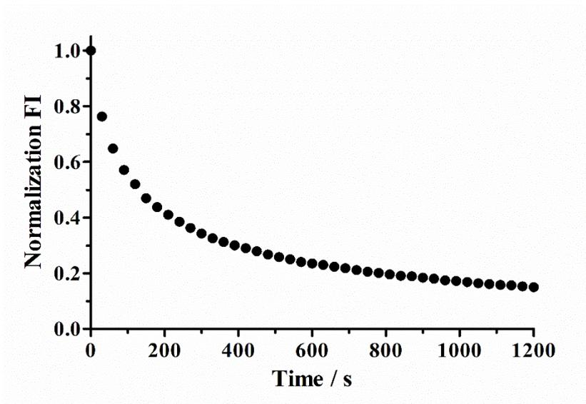
**Figure S5** Kinetics investigation of luminescence response of the Tb/GMP/Hg-Cys sensing system (500  $\mu\text{M}$  Cys used) to 1 mM  $\text{H}_2\text{O}_2$ .
