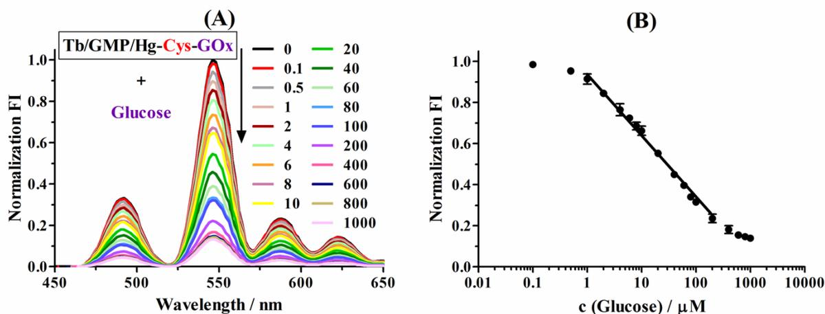
**Figure S8.** The determination of glucose using the Tb/GMP/Hg-Cys-GOx sensing system (500  $\mu\text{M}$  Cys and 0.5  $\mu\text{M}$  GOx used). (A) Luminescence responses of the Tb/GMP/Hg-Cys-GOx sensing system to various glucose concentrations of 0, 0.1, 0.5, 1, 2, 4, 6, 8, 10, 20, 40, 60, 80, 100, 200, 400, 600, 800 and 1000  $\mu\text{M}$ ; (B) Plot of luminescence responses of the Tb/GMP/Hg-Cys-GOx sensing system to various concentrations of glucose indicated.
