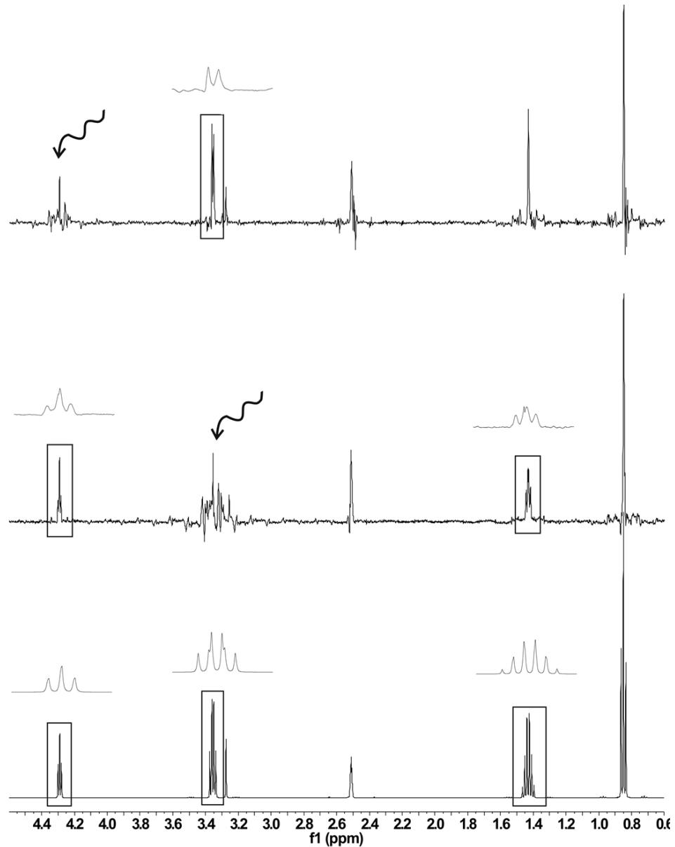
Figure S1: A regular 1D  $^1\text{H}$  spectrum (bottom) and two single scan real-time SERF spectra of a solution of 8 mg n-propanol in 600  $\mu\text{l}$  DMSO- $d_6$ , recorded at 310 K on a Bruker Avance III 500 MHz NMR spectrometer without cryo probe. The selectively refocused signals are indicated by the wavy arrows.
