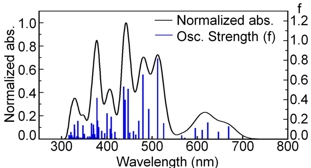
**Figure S21.** Bar graph reporting the oscillator strengths ( $f$ ) as a function of the positions of the electronic transition (blue). The black trace is the same but applying a thickness of  $1000\text{ cm}^{-1}$  to each bar.
