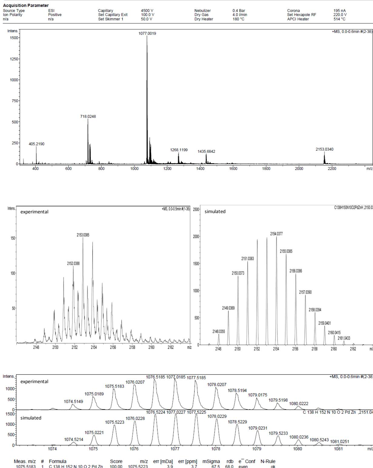
**Figure S5.** Experimental and simulated mass spectra (ESI mass) of **[Fb-Zn]**.
