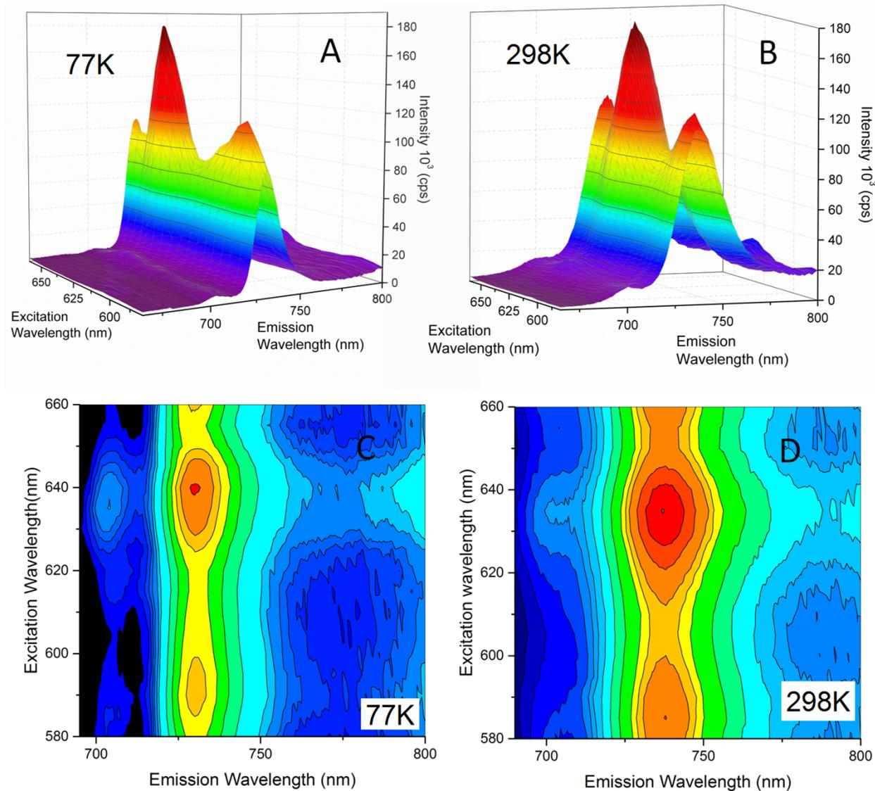
**Figure S24.** 3D (top) and contour maps (bottom) showing the fluorescence spectra of **[Fb-Zn]** in 2-MeTHF at 77 (A, C) and 298 K (B, D).
