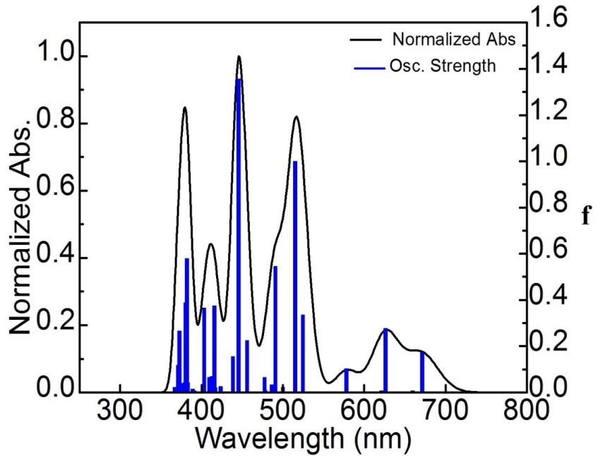
**Figure S22.** Bar graph showing the oscillator strength,  $f$ , as a function of the calculated positions of the electronic transitions (blue) for **[Fb-Fb]**. The black line is the generated spectrum when assigning  $1000\text{ cm}^{-1}$  for each transition.
