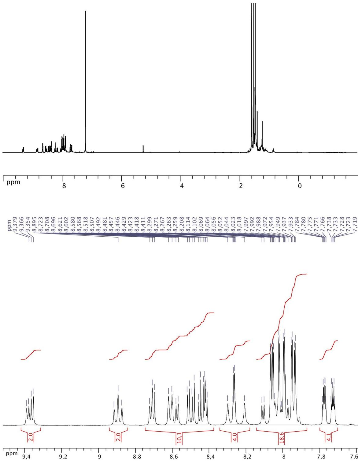
**Figure S1.**  $^1\text{H}$  NMR of **[Fb-Zn]** in  $\text{CDCl}_3$  (bottom: expansion of the aromatic region).
