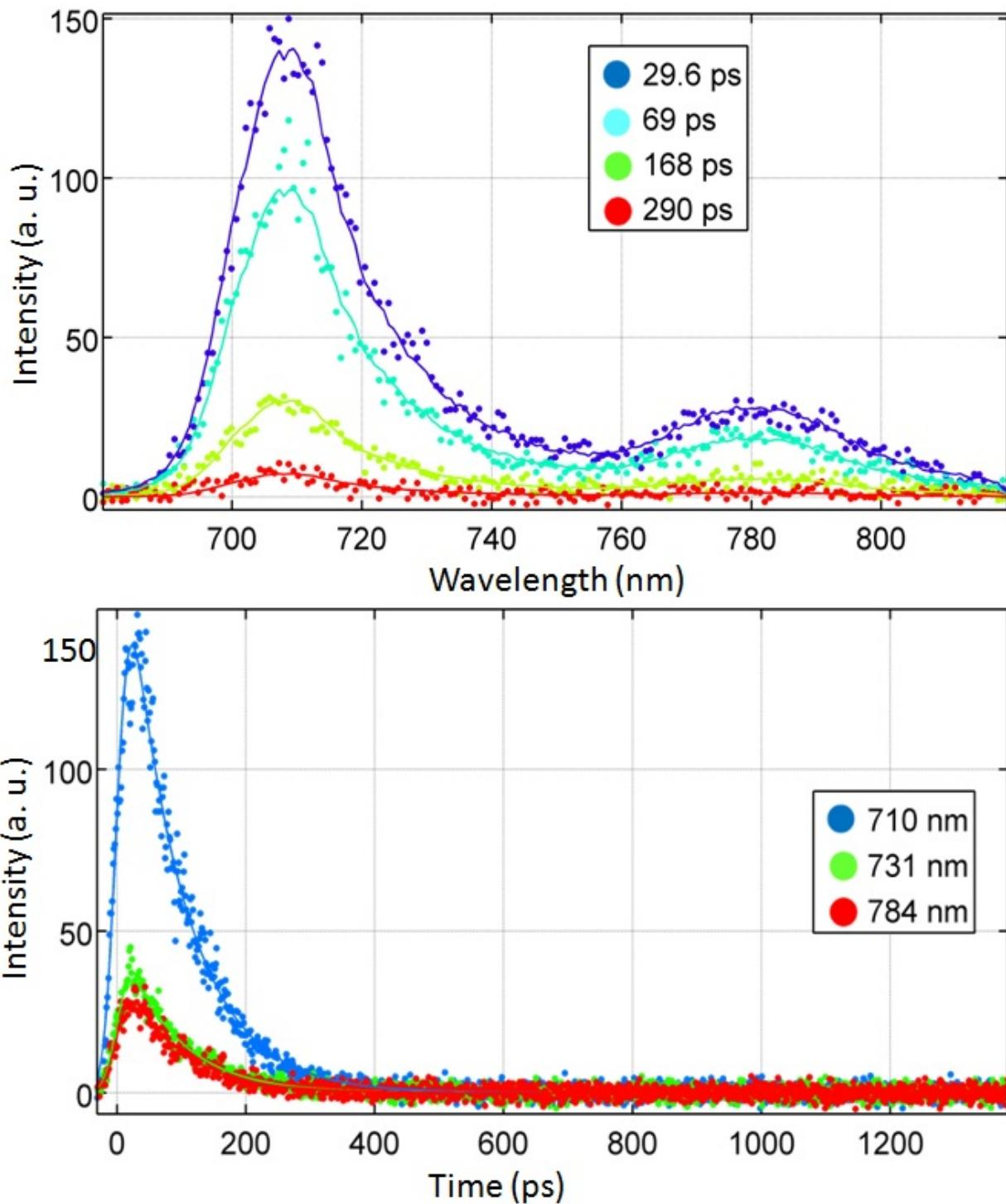
**Figure S12.** Time resolved fluorescence spectra of **[Zn-Zn]** in 2-MeTHF at 77 K using the Streak camera. Top: time-resolved spectra. Bottom: decay traces. The best fits are all monoexponential.
