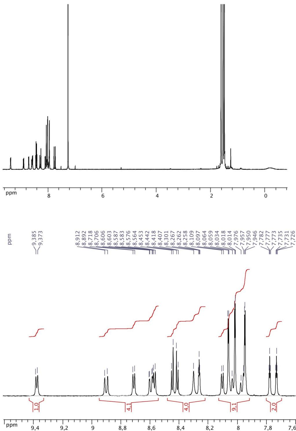
**Figure S8.**  $^1\text{H}$  NMR of [Fb-Fb] in  $\text{CDCl}_3$  (bottom: expansion of the aromatic region).
