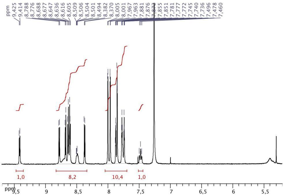
**Figure S7.**  $^1\text{H}$  NMR of **[Zn]** in  $\text{CDCl}_3$  (aromatic part).
