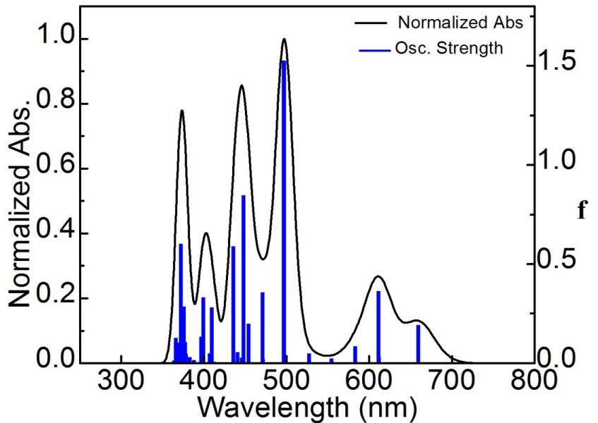
**Figure S23.** Bar graph showing the oscillator strength,  $f$ , as a function of the calculated positions of the electronic transitions (blue) for **[Zn-Zn]**. The black line is the generated spectrum when assigning  $1000\text{ cm}^{-1}$  for each transition.
