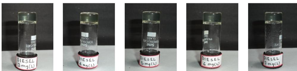
**Figure S28.** Gels from diesel and L-1 at various concentrations of L-1 (a) at 0.3% (w/v) concentration (b) at 0.4% (w/v) concentration (c) at 0.5% (w/v) concentration (d) at 0.6% (w/v) concentration and (e) at 0.7% (w/v) concentration
