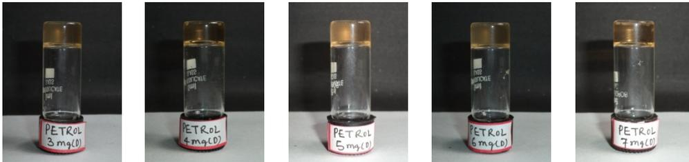
**Figure S25.** Gels from petrol and D-1 at various concentrations of D-1 (a) at 0.3% (w/v) concentration (b) at 0.4% (w/v) concentration (c) at 0.5% (w/v) concentration (d) at 0.6% (w/v) concentration and (e) at 0.7% (w/v) concentration
