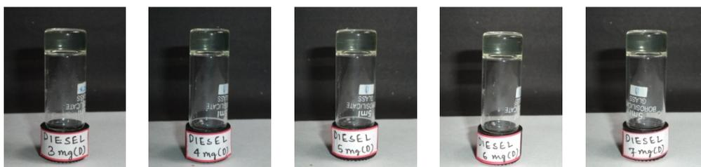
**Figure S27.** Gels from diesel and D-1 at various concentrations of D-1 (a) at 0.3% (w/v) concentration (b) at 0.4% (w/v) concentration (c) at 0.5% (w/v) concentration (d) at 0.6% (w/v) concentration and (e) at 0.7% (w/v) concentration
