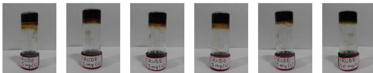
**Figure S30.** Gels from crude oil and L-1 at various concentrations of L-1 (a) at 0.5% (w/v) concentration (b) at 0.6% (w/v) concentration (c) at 0.7% (w/v) concentration (d) at 0.8% (w/v) concentration (e) at 0.9% (w/v) concentration and (f) at 1.0% (w/v) concentration
