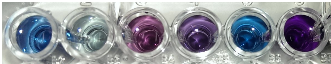
Fig. S1. Photograph of wells containing diluted test samples after acidification with (from left to right) acetic acid, hydrochloric acid, sulfuric acid, phosphoric acid, trichloroacetic acid and nitric acid (acids prepared as aq. 10% w/v solutions and used as described in section 1.3).
