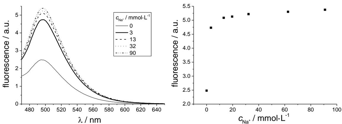
**Figure 15** Emission spectra ( $\lambda_{\text{ex}} = 450 \text{ nm}$ ) of a fiber-optical sensor at different sodium ions concentrations.
