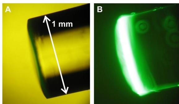
**Figure 11** A: Transmission microscopy picture of the dipped optical fiber and B: Fluorescence microscopic picture with an excitation-filter transmitted light from 445 nm to 450 nm and an emission filter transmitted light between 505 nm to 550 nm.
