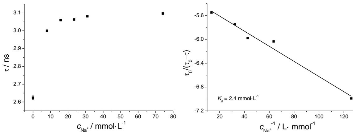
**Figure 16** Calibration of an optode with fiber-optical frequency-domain spectroscopy (FD-S). The used solution contains 10 mM Tris buffer.
