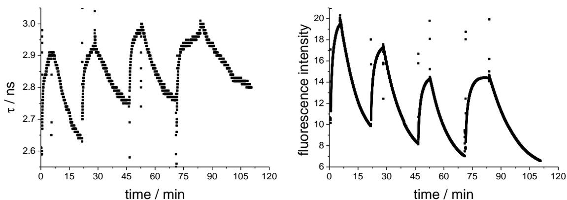
**Figure 17** Response time and signal stability of an optode by periodically switching the concentration of sodium from 0 to 10 mM.
