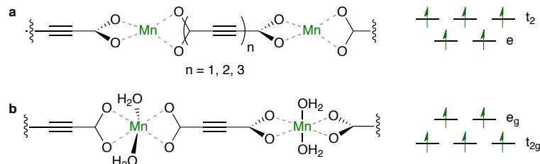
Figure S1: Schematic structures and ligand field splitting for Mn polymers with (a) tetrahedral and (b) octahedral coordination. The associated relaxed structure parameters are given in the tables below.
