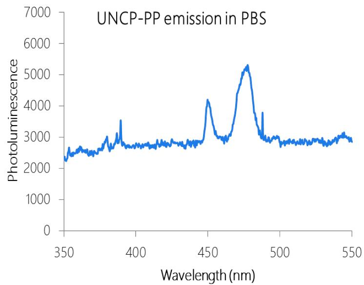
**Figure S-4.** Visible range spectrum of the upconversion emission from a dilute solution of UCNP@PL-PEG nanocarriers in pH 7.4 PBS upon irradiation with 980 nm light at 1.0 W. This shows the characteristic emission peaks at 450 and 475 nm associated with Tm-doped UCNPs.
