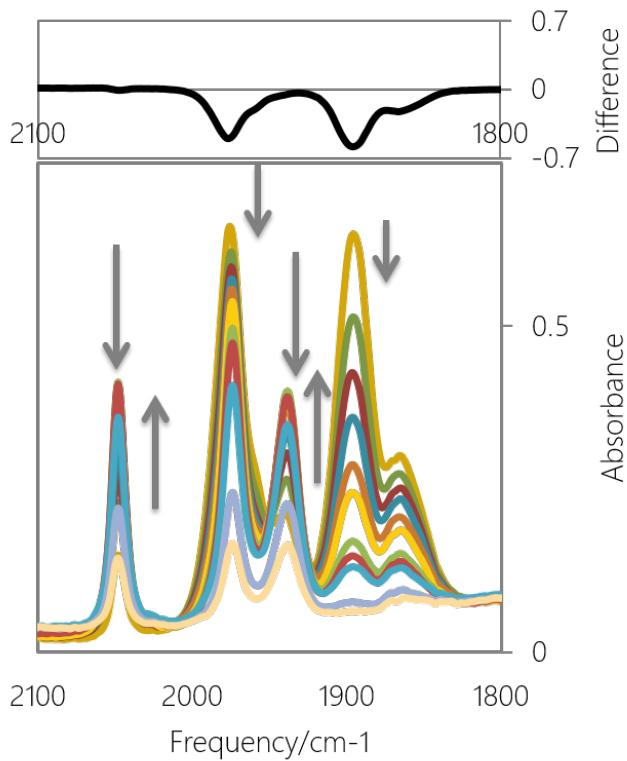
**Figure S-3:** Spectral changes of an aerated DCM solution of **2** in the  $\nu_{\text{CO}}$  region upon irradiation with 470 nm light.
