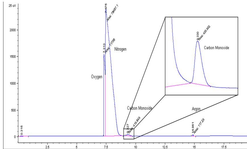
**Figure S-6:** GC trace showing the production of CO in the headspace of a vial containing an aqueous suspension of the photoCORM loaded UCNP@PL-PEG nanocarriers when irradiated with 980 nm light.
