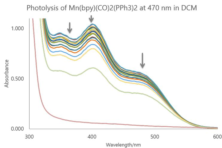
**Figure S-2:** Spectral changes of an aerated DCM solution of **2** in the UV-visible region upon irradiation with 470 nm light.
