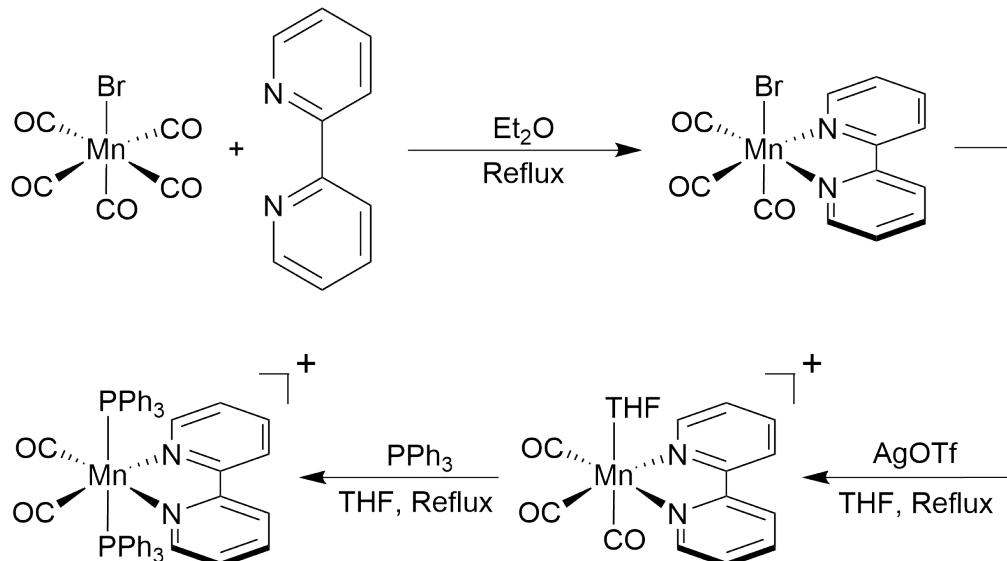
**Scheme S-1.** Synthetic sequence for the preparation of  $\text{Mn}(\text{bpy})(\text{CO})_2(\text{PPh}_3)_2^+$
