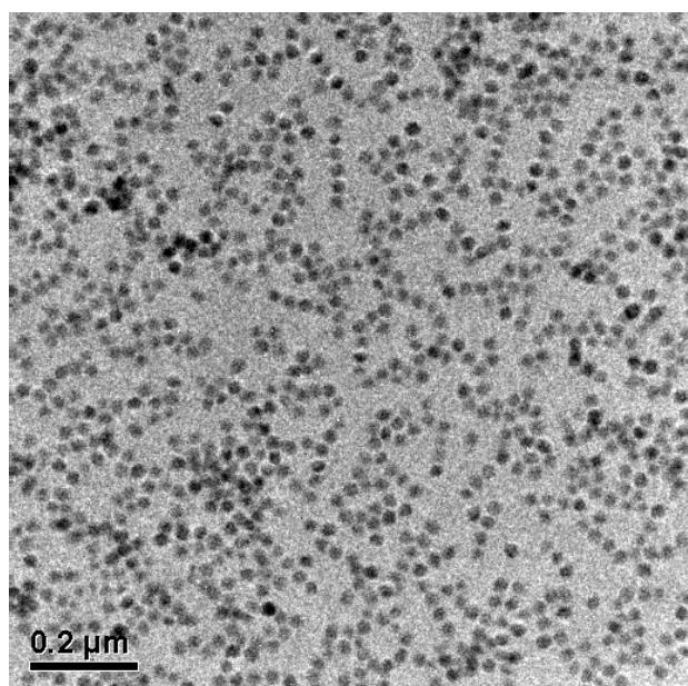
**Figure S-1:** TEM image of  $\text{NaGdF}_4\text{:Tm,Yb}@\text{NaGdF}_4$  UCNPs
