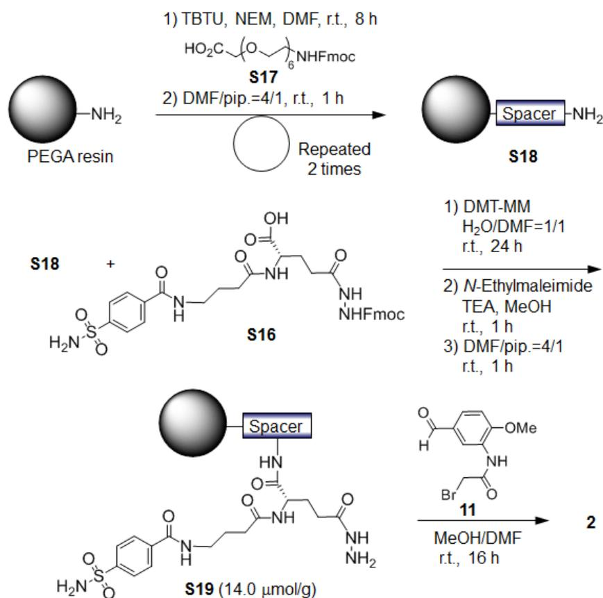
**Scheme S4.** Synthetic scheme of the solid-supported chemical tool **2**. TBTU = *N,N,N',N'*-tetramethyl-*O*-(benzotriazol-1-yl)uronium tetrafluoroborate; NEM = *N*-ethylmorpholine; DMF = *N,N*-dimethylformamide; TFA = trifluoroacetic acid; Fmoc = 9-fluorenylmethyloxycarbonyl.
