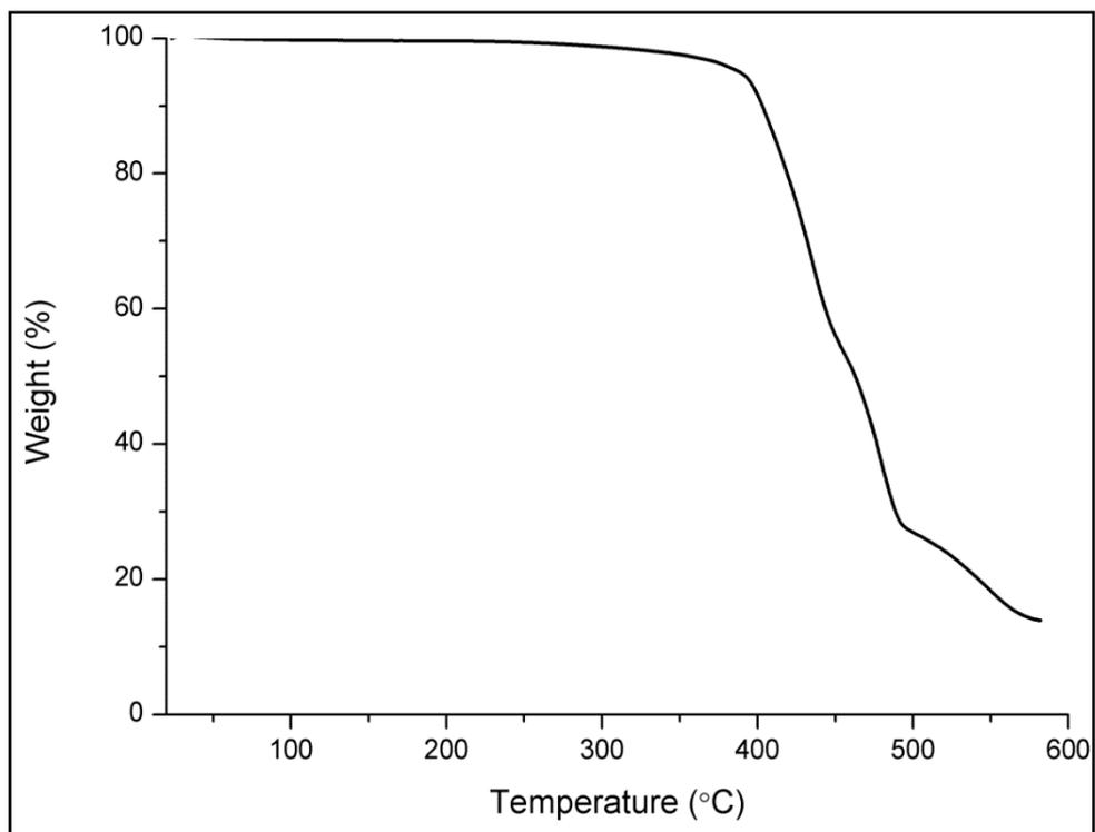
Figure S3: TGA for activated 1.
