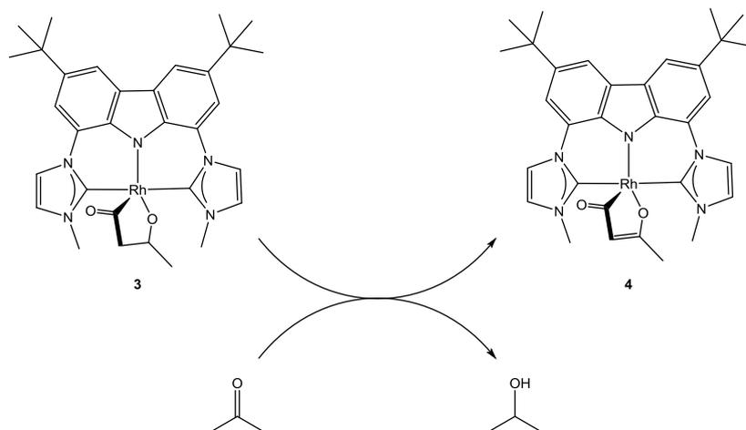
Dehydrogenation of complex 3 to complex 4 is accompanied by hydrogenation of the acetone (which is formed during the catalysis) to isopropanol (Figure 8).
