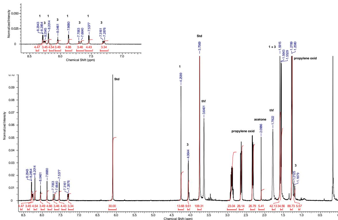
**Figure 13.**  $^1\text{H}$  NMR spectrum after 16 h at room temperature in  $\text{thf-d}_8$  (std = 1,3,5-trimethoxybenzene).
