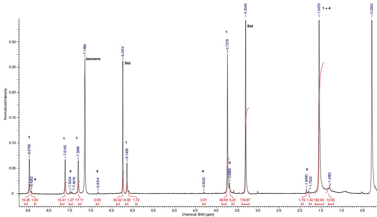
**Figure 16.**  $^1\text{H}$  NMR spectrum after removing all volatiles in vacuo and dissolving the residue again in benzene- $\text{d}_6$  (std = 1,3,5-trimethoxybenzene).
