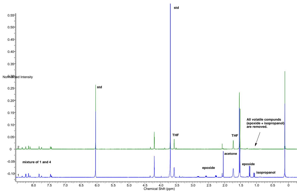
**Figure 8.** After evaporation of all volatile compounds the signal at 1.08 ppm (isopropanol) is missing (std = 1,3,5-trimethoxybenzene).
