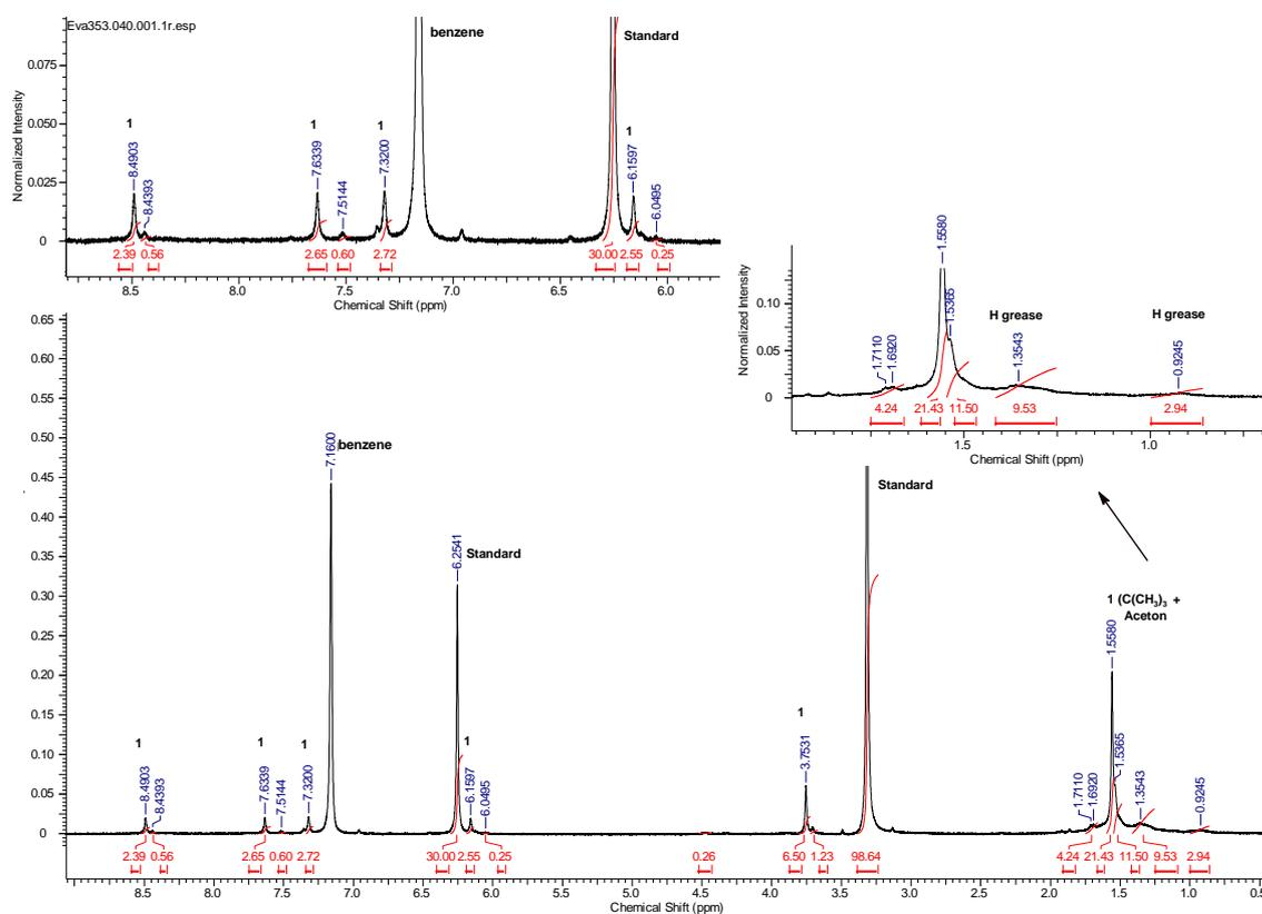
**Figure 11.** The reaction mixture after removing all volatiles and dissolving of the residue in benzene-d<sub>6</sub> (Standard = 1,3,5-trimethoxybenzene).
