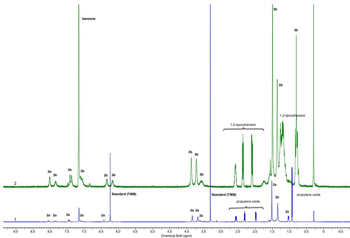
**Figure 1.** Complete conversion of **1a** and propylene oxide (**1**, blue) or 1,2-epoxyhexane (**2**, green) at room temperature to complexes **2a** and **2b**.
