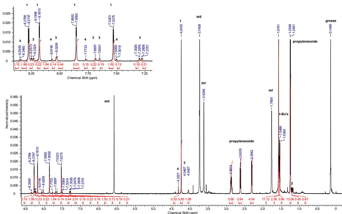
**Figure 4.**  $^1\text{H}$  NMR spectrum recorded directly after the addition of propylene oxide (std = 1,3,5-trimethoxybenzene).
