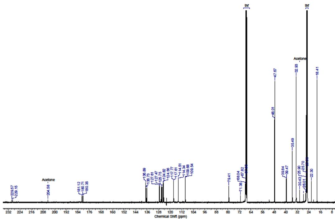
$^{13}\text{C}$ -DEPT-135 NMR spectrum of **3a** in  $\text{thf-d}_8$ :
