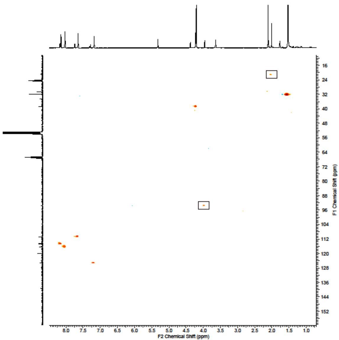
$^1\text{H}$ - $^{13}\text{C}$ -HMBC NMR spectrum of **4a** in  $\text{CD}_2\text{Cl}_2$
