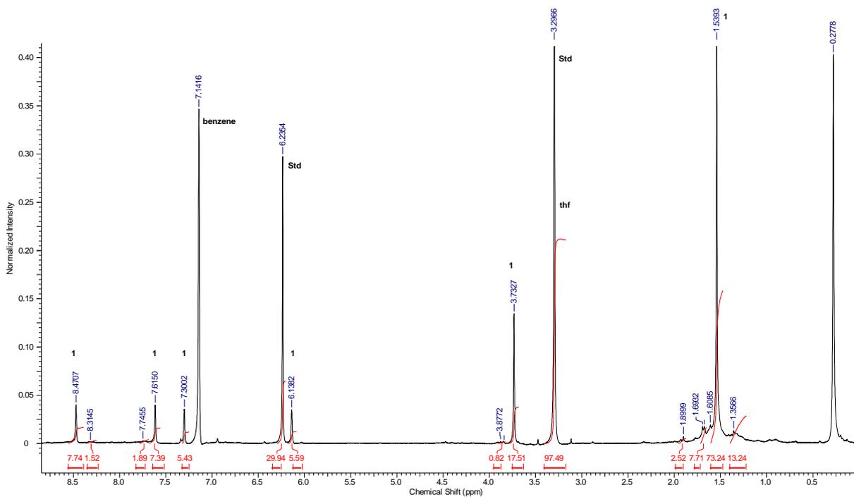
**Figure 14.**  $^1\text{H}$  NMR spectrum after removing all volatiles in vacuo and dissolving the residue in benzene- $\text{d}_6$  (std = 1,3,5-trimethoxybenzene).
