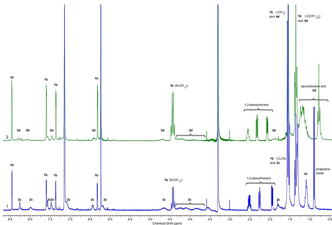
**Figure 2.** Reaction of **1b** with propylene oxide (**1**, blue) and 1,2-epoxyhexane (**2**, green) at room temperature led to the analogue complexes **2c** and **2d**. In this case the conversion of **1b** is incomplete and led to a ratio of **1b:2c = 4:3** or **2d (1b:2d = 8:1)**.
