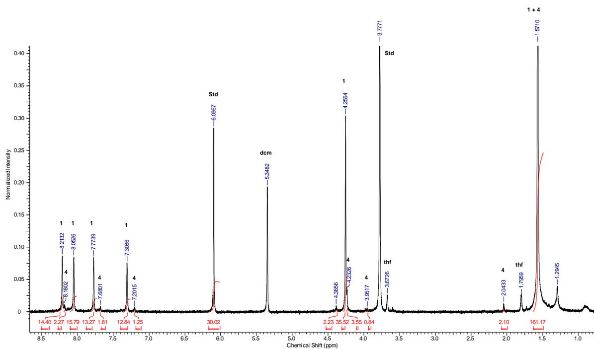
**Figure 17.**  $^1\text{H}$  NMR spectrum after removing benzene- $\text{d}_6$  and dissolving the residue in dichloromethane- $\text{d}_2$  to verify complex **4** by its chemical shift (std = 1,3,5-trimethoxybenzene).
