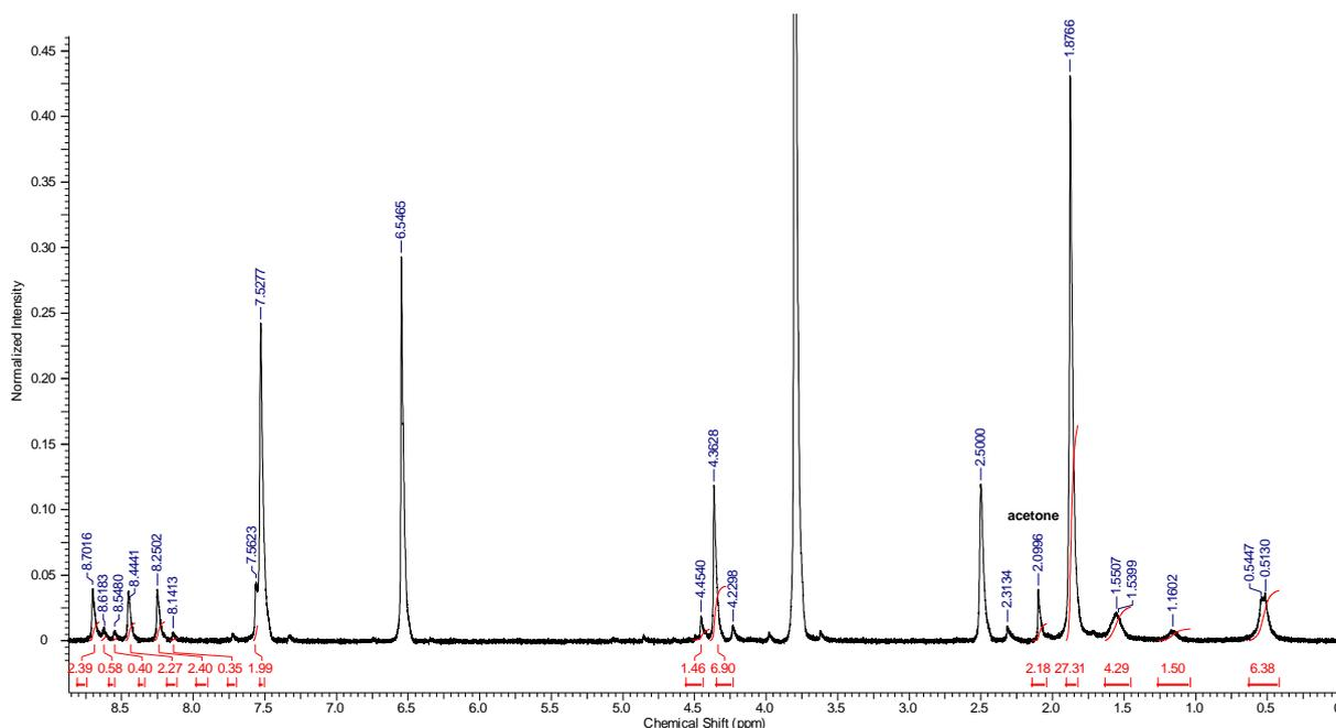
**Figure 12.** Addition of  $\text{dms}\text{-d}_6$  to the solution shifts the acetone signal so that it is not covered by the *t*-Bu signal.
