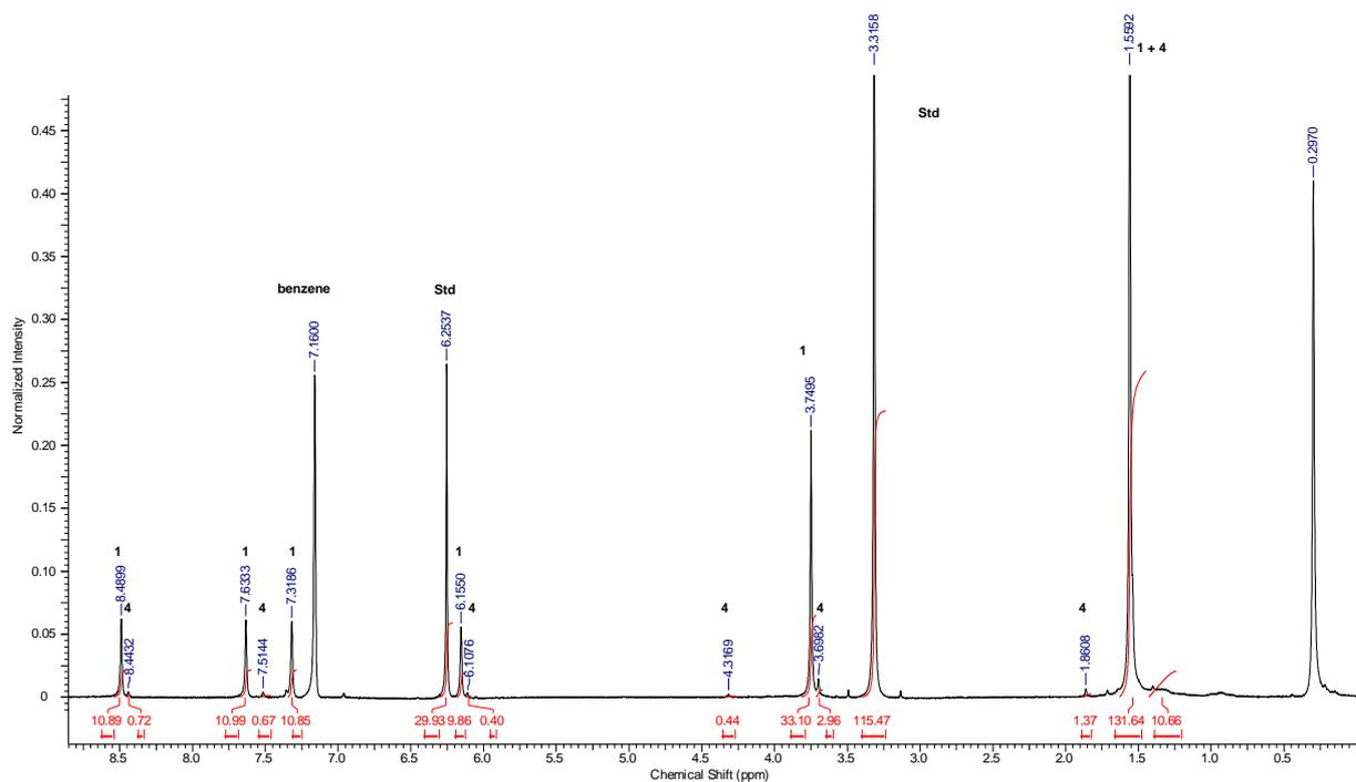
**Figure 15.** After heating the suspension for 1 h at 60 °C, the dehydrogenated rhodium species **4** can be detected in the  $^1\text{H}$  NMR spectrum (std = 1,3,5-trimethoxybenzene).
