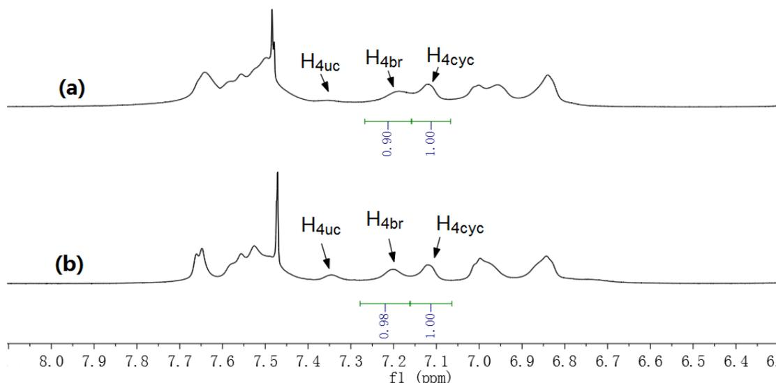
**Figure S7.** Partial  $^1\text{H}$  NMR spectra (400 MHz,  $\text{CDCl}_3\text{-CD}_3\text{CN} = 1/1$ , v/v, 298 K, fixed  $\text{B}_3$  concentration 15mM) of (a) equimolar mixture of  $\text{B}_3$  and  $\text{A}_2$  (b) 1 : 1.5 molar ratio of  $\text{B}_3$  and  $\text{A}_2$ . Peaks of uncomplexed monomers, cyclic oligomers, and the hyperbranched assembly, are designated as uc, cyc, and br, respectively.
