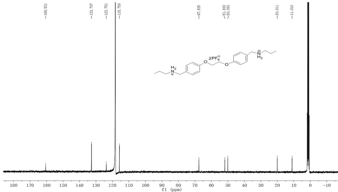
**Figure S15.** <sup>13</sup>C NMR spectrum (75 MHz, CDCl<sub>3</sub>, room temperature) of compound **A<sub>2</sub>**.
