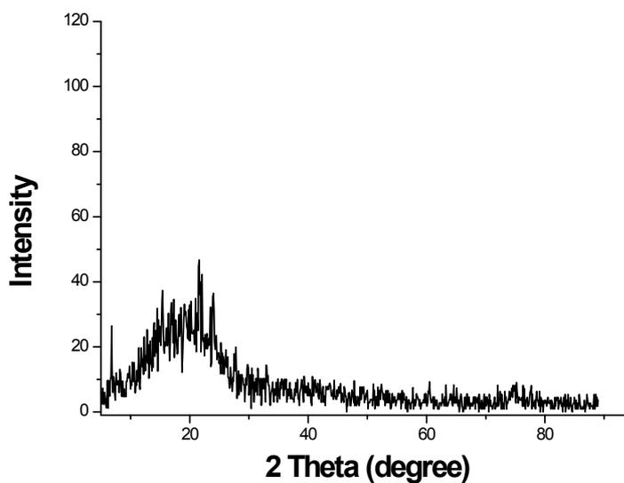
**Figure S4.** XRD analysis of sample obtained from concentrated mixed solution of **B**<sub>3</sub> and **A**<sub>2</sub>.
