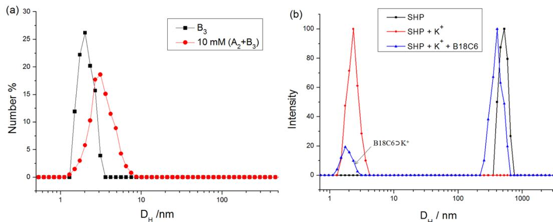
**Figure S6.** (a) Distributions of the hydrodynamic diameter of  $\text{B}_3$  and a mixture of 10 mM  $\text{B}_3$  and 1.5 equiv.  $\text{A}_2$  in chloroform/ acetonitrile (1 : 1, v/v) at 298 K. (b) Size distributions of SHP ( $\text{B}_3=65\text{mM}$ ) in chloroform/ acetonitrile (1 : 1, v/v) at 298 K before and after addition of  $\text{KPF}_6$ , and removal of  $\text{K}^+$ .
