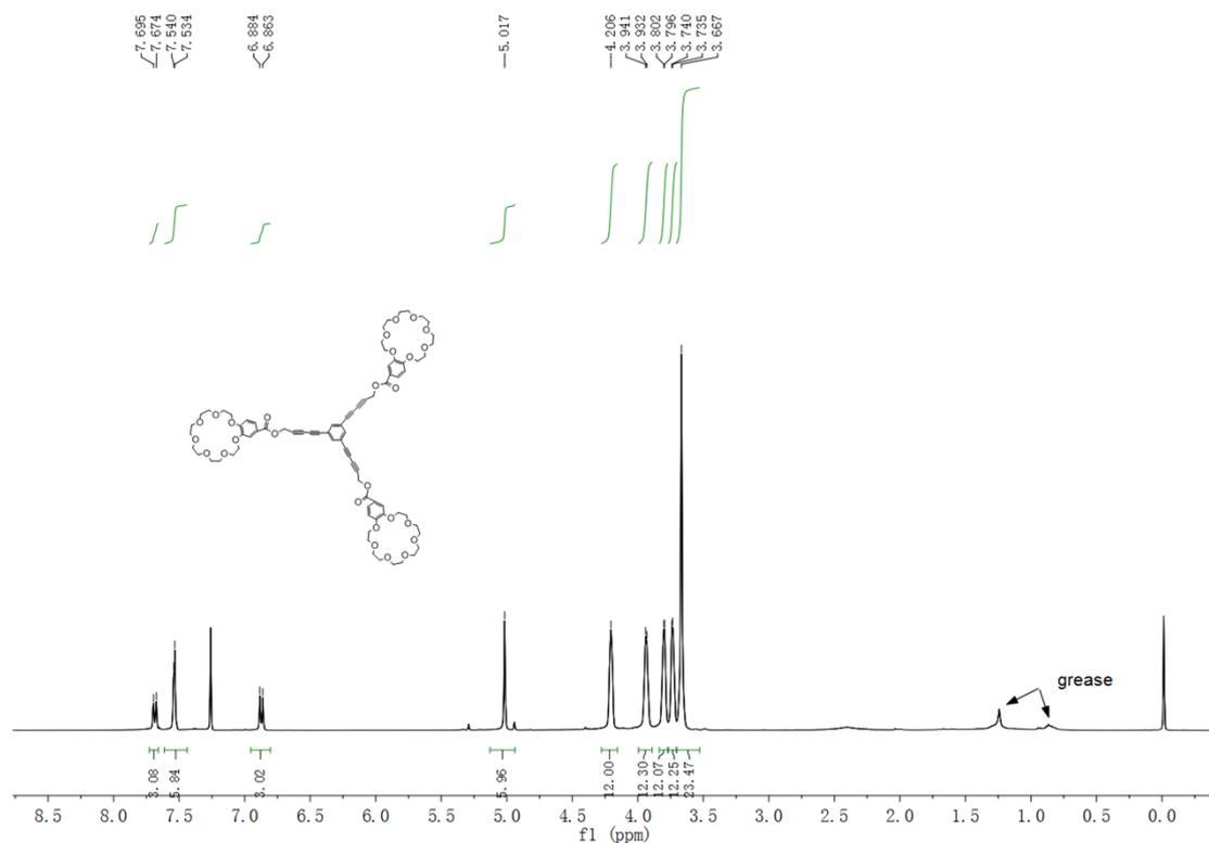
**Figure S11.** <sup>1</sup>H NMR spectrum (400 MHz, CDCl<sub>3</sub>) of compound **B<sub>3</sub>**
