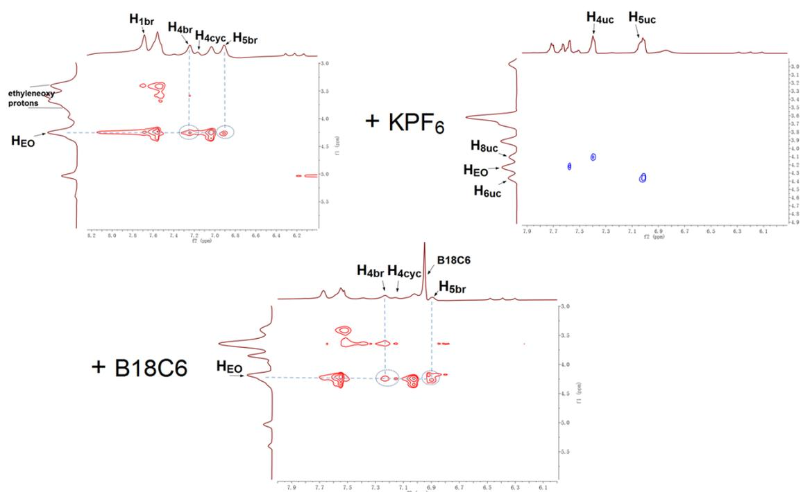
**Figure S5.** Partial NOESY NMR spectra (400 MHz,  $CDCl_3$ – $CD_3CN = 1/1$ , v/v, 298 K) of (a)  $B_3$  (45 mM) with 1.5 equiv.  $A_2$ , (b) after addition of 3 equiv.  $KPF_6$ , and (c) after addition of 3 equiv. B18C6.
