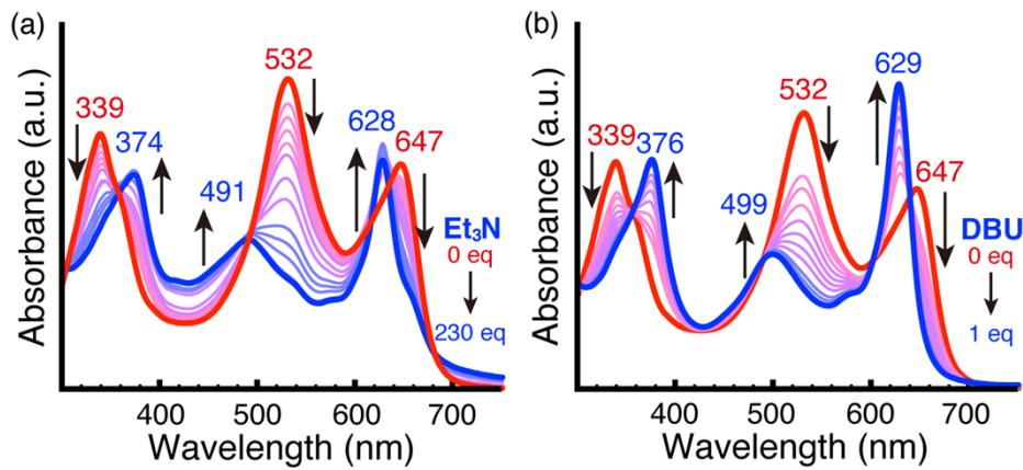
**Figure S5.** Spectral changes of **3** solution by (a) adding Et<sub>3</sub>N (0~230 eq) and (b) adding DBU (~1 eq) in CH<sub>2</sub>Cl<sub>2</sub>.
