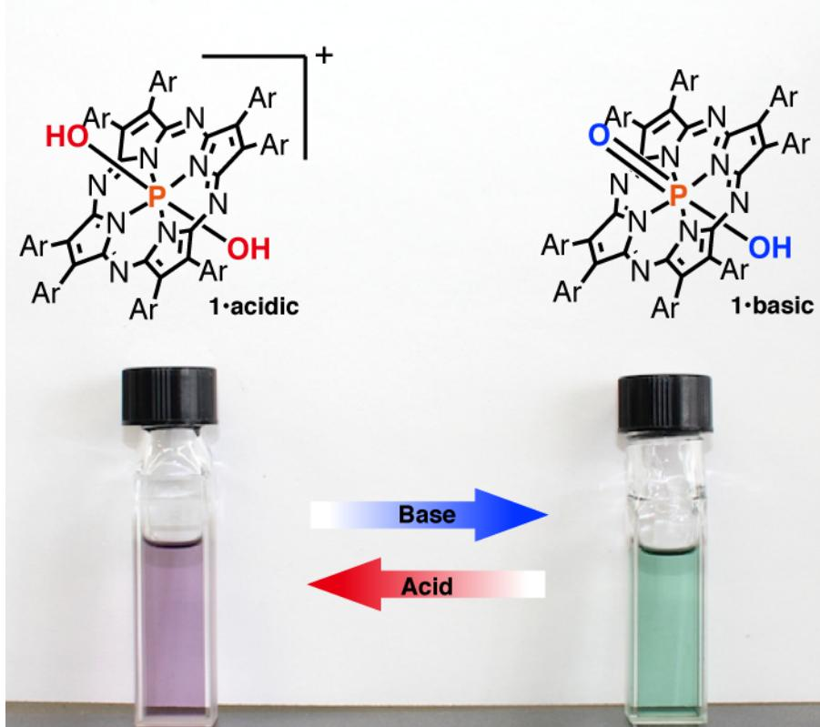
**Figure S3.** Photograph of PTAP **1** solutions under acidic and basic conditions.
