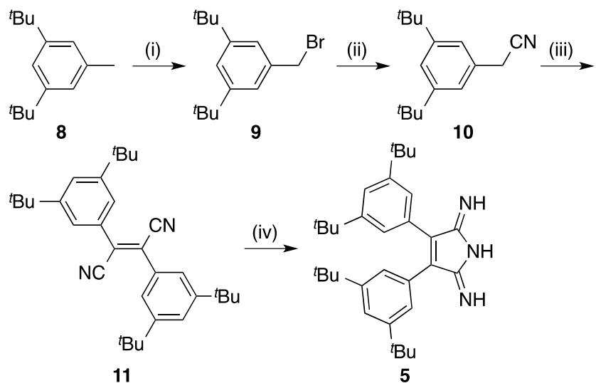
**Scheme S1.** Synthesis of TAP precursor **5**. *Reagents and conditions:* (i) NBS (1 eq), benzoyl peroxide (3 mol%), CCl<sub>4</sub>, reflux, 1 h, 97%; (ii) NaCN (1.2 eq), DMSO, rt, 24 h, 65%; (iii) I<sub>2</sub> (2 eq), MeONa (5 eq), Et<sub>2</sub>O, 0°C, 1 h, 36%; (iv) MeONa (10 mol%), NH<sub>3</sub> (gas), ethylene glycol, 115°C, 6 h, 69%.
