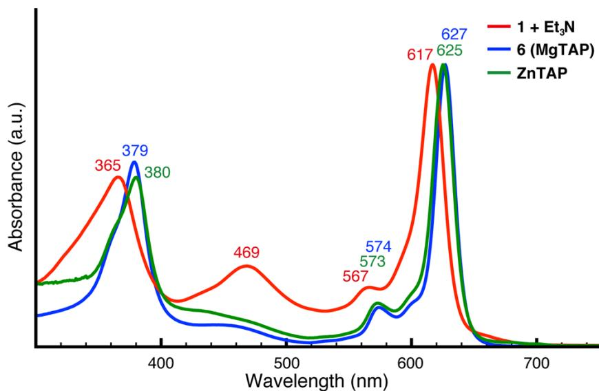
**Figure S4.** UV-vis absorption spectra of **1+Et<sub>3</sub>N** (excess.) (red), **6** (blue), and ZnTAP (green) in toluene.
