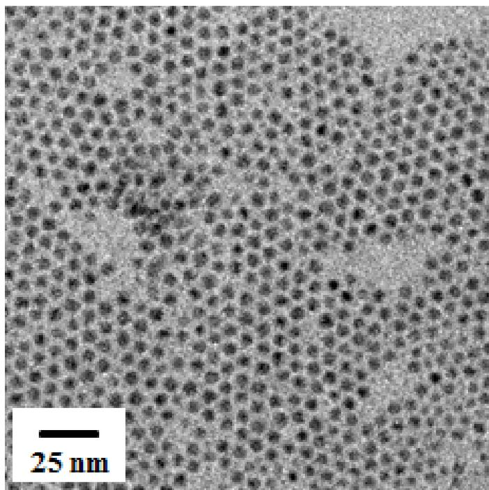
Figure S6. TEM image of Ag-Na<sub>2</sub>Se<sub>2</sub> molar ratio 8 : 1. Nanoparticles size is 6.1 nm and standard deviation is 0.36
