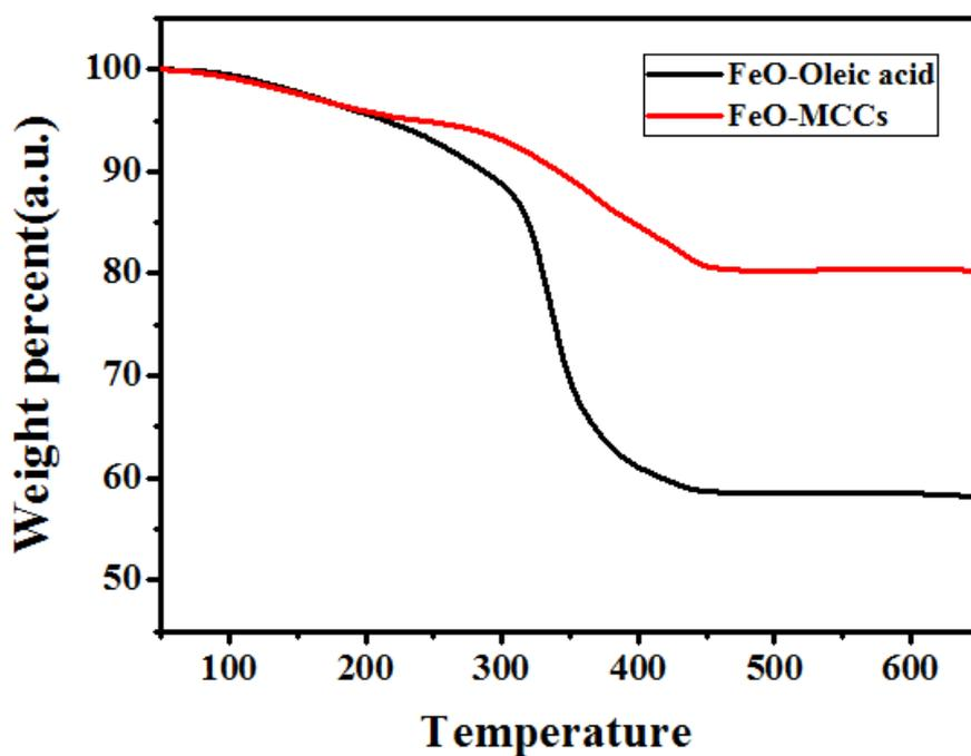
Figure S10. Thermogravimetric analysis of FeO-Oleic acid (black curve, FeO capping with oleic acid) and FeO-MCCs (red curve, FeO- $\text{Na}_2\text{Se}_2$  molar ratio 4 : 1)
