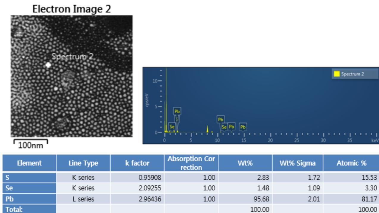
Figure S4. Energy-dispersive X-ray spectroscopy scanning transmission electron microscopy (EDX-STEM) elemental analysis of PbS-Na<sub>2</sub>Se<sub>2</sub> molar ratio 4 : 1.
