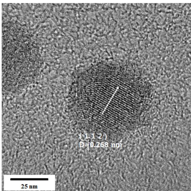
Figure S8. HR-TEM images of Ag-Na<sub>2</sub>Se<sub>2</sub> molar ratio 1 : 4 with the distance between the lattice planes
