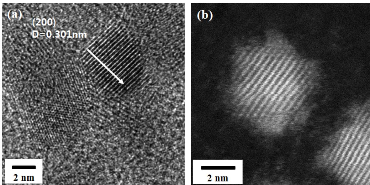
Figure S3. HR-TEM images of (a) with the distance between the lattice planes and HR-STEM image of (b) PbS-Na<sub>2</sub>Se<sub>2</sub> molar ratio 4 : 1.
