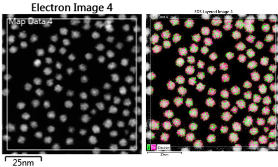
Figure S5. Elemental mapping analysis of PbS-Na<sub>2</sub>Se<sub>2</sub> molar ratio 4 : 1. Selenium color is Pink. Sulfur color is green.
