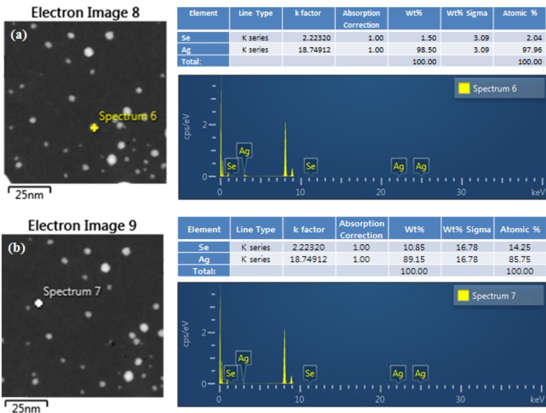
Figure S7. EDX-STEM elemental analysis of Ag-Na<sub>2</sub>Se<sub>2</sub> molar ratio 4 : 1. (a) 5 nm nanoparticle (b) less than 2 nm nanoparticle.
