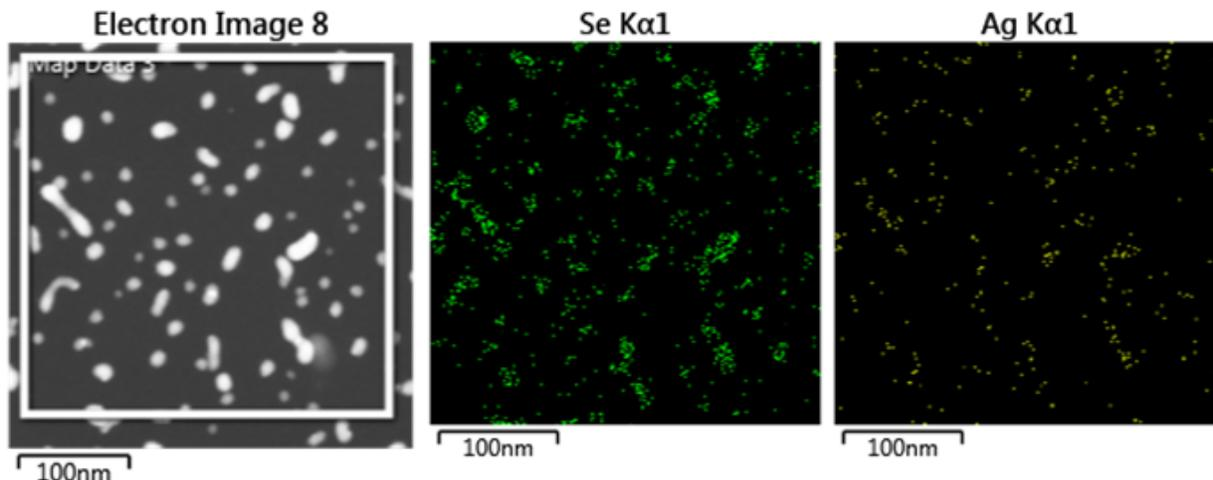
Figure S9. Elemental mapping analysis of Ag- $\text{Na}_2\text{Se}_2$  molar ratio 1 : 4.
