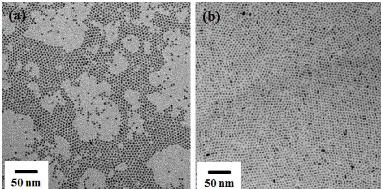
Figure S1. Low magnification Transmission electron microscopy (TEM) images of (a) bare PbS, (b) PbS- $\text{Na}_2\text{Se}_2$  molar ratio 4 : 1.
