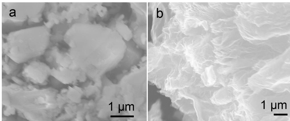
**Figure S3** SEM images of the (a) pristine  $\text{Li}_3\text{VO}_4$  and (b)  $\text{Li}_3\text{VO}_4$ @GNS composite.
