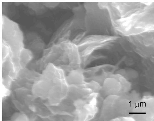
**Figure S7** SEM image of the  $\text{Li}_3\text{VO}_4@\text{GNS}$  composite after 500 cycles at 5C rate. The composite has retained the original morphology as shown in Figure S3b, demonstrating excellent structure stability of this composite materials.
