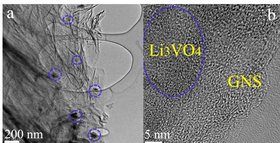
**Figure S4** TEM images of the  $\text{Li}_3\text{VO}_4$ @GNS composite revealing smaller  $\text{Li}_3\text{VO}_4$  particles with size around 10-30 nm.
