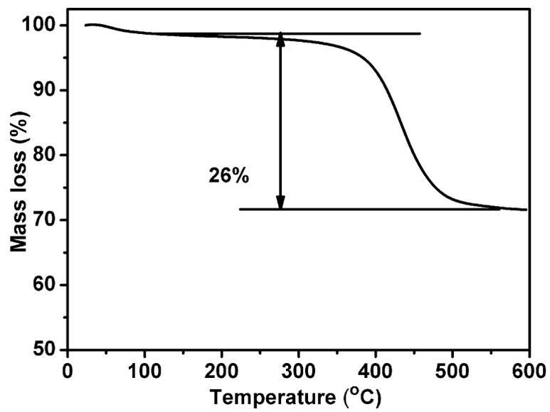
**Figure S2** TGA curves of  $\text{Li}_3\text{VO}_4@\text{GNS}$  in air.
