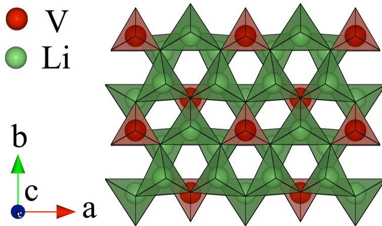
**Figure S1** Schematic structure diagram of  $\text{Li}_3\text{VO}_4$ .
