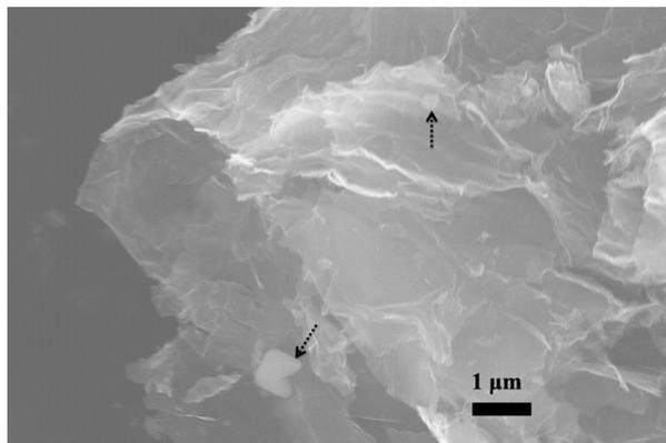
**Figure S5** SEM image of the  $\text{Li}_3\text{VO}_4@\text{GNS}$  composite revealing larger  $\text{Li}_3\text{VO}_4$  particles with size around 500 nm.
