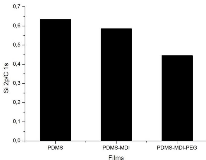
**Figure S-4.** Comparison of the atomic ratio Si(2p)/C(1s) measured by XPS onto the following surfaces: unmodified PDMS (PDMS) , PDMS modified by MDI (PDMS-MDI) and PDMS-MDI-PEG films.
