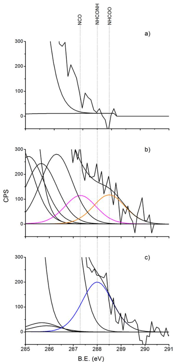
**Figure S-6.** High resolution spectrum obtained by XPS and focused in the O(1s) region between 285 and 295 eV of the following surfaces and compounds analyzed: (a) unmodified PDMS (PDMS), (b) PDMS surface modified by MDI (PDMS-MDI) and (c) PDMS-MDI surface modified with amino and alkyne ended PEG chains (PDMS-MDI-PEG). CPS = count per second.
