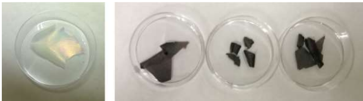
Figure S1. Photographs of unloaded MPC (left image) and the gold nanoparticle-loaded films (right image): MPC-Au-5 (left), MPC-Au-10 (middle) and MPC-Au-100 (right).
