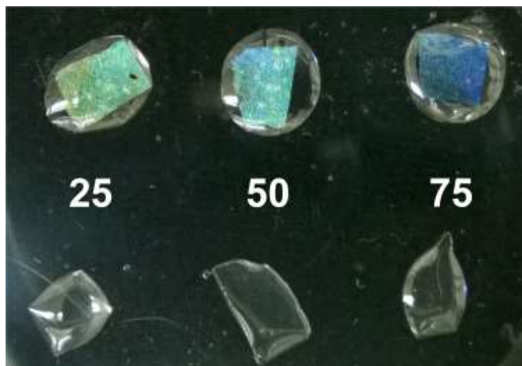
Figure S11. Photographs of MPC-Au-100 (top) and unloaded MPC (bottom) after addition of an aqueous solution of 2-mercaptoethanol ( 25 : 25 vol% 2-mercaptoethanol; 50 : 50 vol% 2-mercaptoethanol; 75 : 75 vol% 2-mercaptoethanol).
