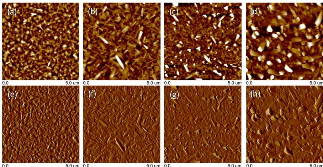
**Fig. S6** The AFM images of the thin film **DAP1** spin coated from  $\text{CHCl}_3$  solution onto ODTs (a: before annealing; b: annealing at  $150\text{ }^\circ\text{C}$ ) and HMDS (c: before annealing; d: annealing at  $150\text{ }^\circ\text{C}$ ) treated substrates. (e-h) are the corresponding phase images.
