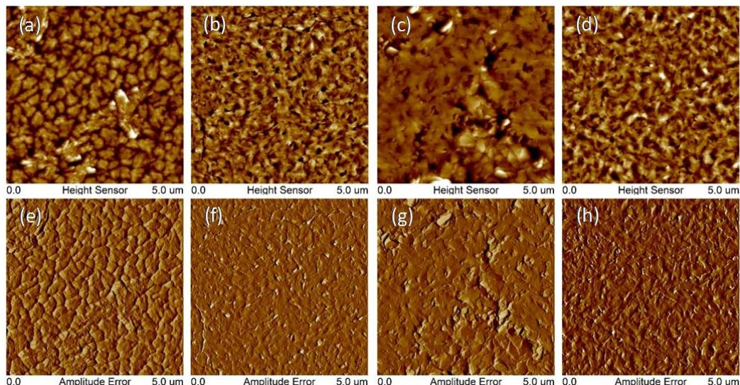
**Fig. S7** The AFM images of thin film **DAP2** spin coated from  $\text{CHCl}_3$  solution on the ODTs-treated substrates annealing at  $120\text{ }^{\circ}\text{C}$  (a),  $150\text{ }^{\circ}\text{C}$  (b), and  $180\text{ }^{\circ}\text{C}$  (c), and on the HMDS -treated substrates annealing at  $150\text{ }^{\circ}\text{C}$  (d). (e-h) are the corresponding phase images.
