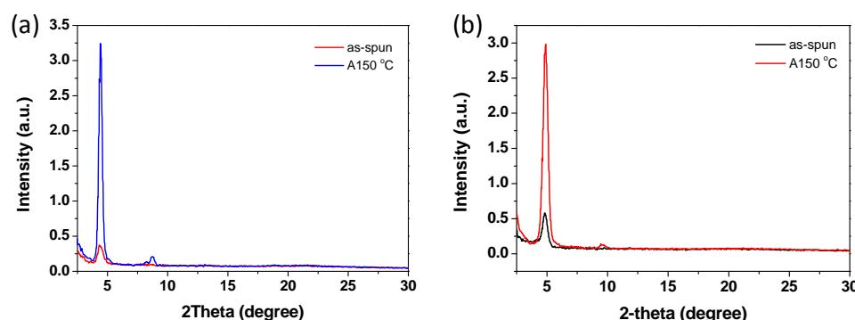
**Fig. S8** XRD patterns of **DAP1** (a) and **DAP2** (b) thin films on ODTs-modified substrates.
