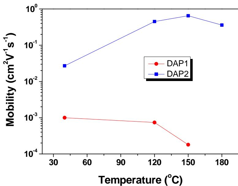
**Fig. S5** The charge carrier mobilities of **DAP1** and **DAP2** with respect to the annealing temperatures.
