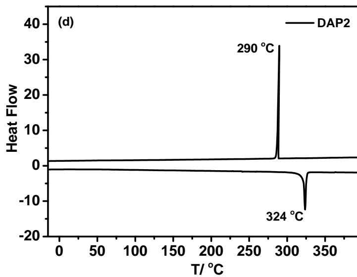
**Fig. S4** Thermogravimetric analysis (TGA) of compounds **DAP1** (a) and **DAP2** (c); Differential scanning calorimetry (DSC) of compounds **DAP1** (b) and **DAP2** (d) in N<sub>2</sub> at a heating rate of 10 °C min<sup>-1</sup>.
