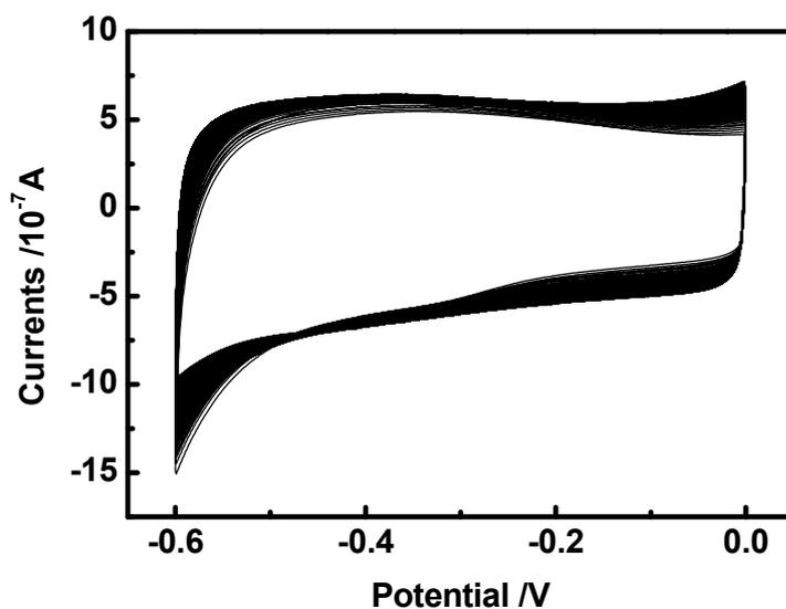
**Figure S5.** Cyclic voltammograms (CV) of Hemin-MHN model with ODT in 25 mM pH 7.0 HEPES containing 1 mM histidine. The scan rate was  $50 \text{ mV}\cdot\text{s}^{-1}$ .
