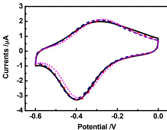
**Figure S8.** CVs of hemin in the Hemin-His model in 25 mM HEPES (pH 7.0) in the absence of EDTA (solid curve), in the presence of 1 mM EDTA for 10 min (dotted curve), 10 h (short dashed curve) and 5 mM EDTA for 10 h (short dotted curve). The concentration of hemin used in (B) is  $50 \text{ }\mu\text{M}$ .
