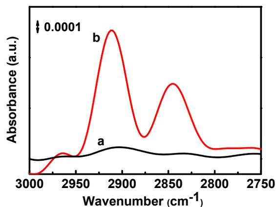
**Figure S1.** SEIRAS spectra of: Hemin-MHN Model in high-wavenumber region before (a) and after (b) ODT attachment.
