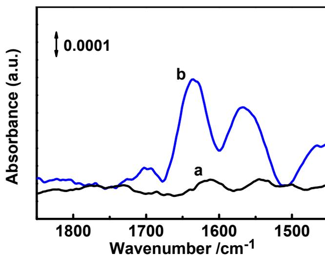
**Figure S2.** SEIRAS spectra of: MHN SAM before (a) and after (b) His assembling. The spectrum of MHN SAM is taken as baseline as shown in curve *a*. Two distinct bands at 1635 cm<sup>-1</sup> and 1567 cm<sup>-1</sup> in curve *b* are characteristics of amide I band and amide II band of the amide bond formed between His and MHN molecules respectively, which clearly indicate the attachment of His molecules on the surface.
