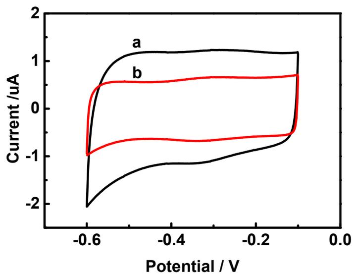
**Figure S6.** CVs of hemin in the Hemin-MHN model (a) without and (b) with 1-hexanethiol in 25 mM pH 7.0 HEPES. The scan rate was  $50 \text{ mV}\cdot\text{s}^{-1}$
