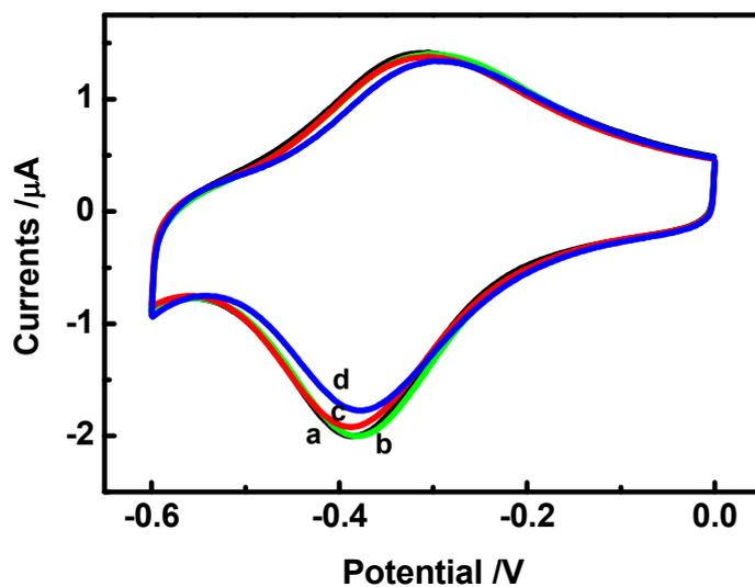
**Figure S9.** CVs of hemin in the Hemin-His model in 25 mM HEPES (pH 7.0) in the absence of His (a), in the presence of 20  $\mu\text{M}$  EDTA for 10 min (b), 10 h (c) and 3 mM His for 3 h (d).
