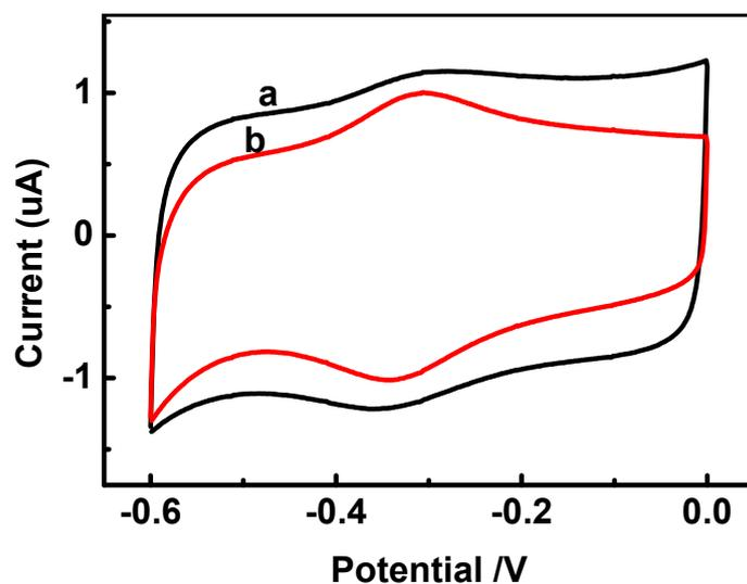
**Figure S7.** CVs of hemin in the Hemin-His model (a) without and (b) with ODT in 25 mM pH 7.0 HEPES. The scan rate was  $50 \text{ mV}\cdot\text{s}^{-1}$
