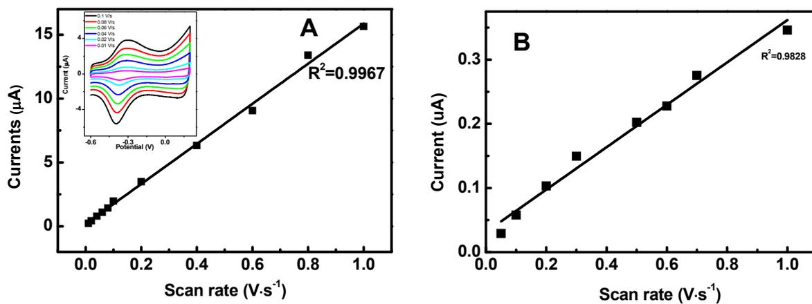
**Figure S3.** Plots of the anodic peak currents of hemin vs. scan rate in 25 mM pH 7.0 HEPES: (A) Hemin-His model and (B) Hemin-MHN model.
