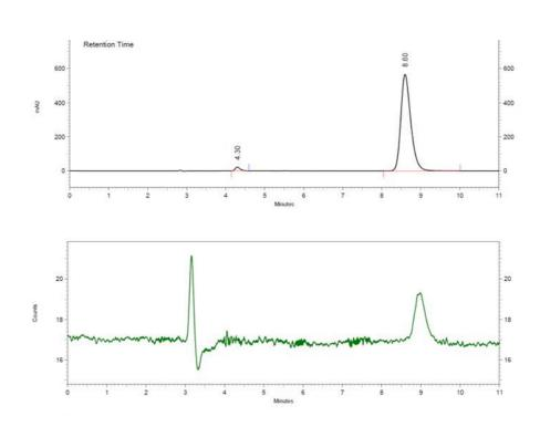
1: 254 nm, 4 nm Results Area % Retention Time Area Capacity factor Relative RT Resolution (USP) 4.30 787161 1.91 0.43 0.00 0.00 8.60 40398803 98.09 1.87 0.00 12.38 Totals 41185964 100.00
