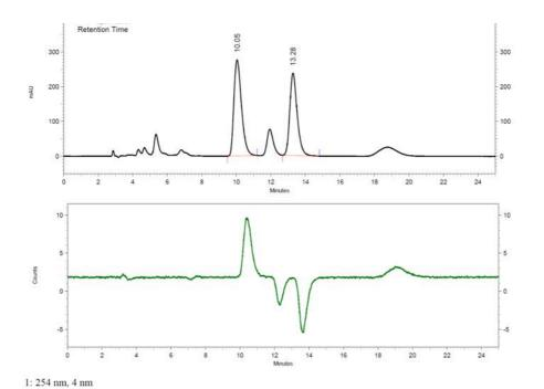
Results Retention Time Area 7637260 Area % 49.88 Capacity factor 2.98 5.25 Resolution (USP) 0.00 Relative RT 1.00 18.76 0.00 5.06 7673122 50.12 Totals 100.00 15310382
