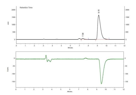
1: 254 nm, 4 nm Results Retention Time Area % Capacity factor Relative RT Resolution (USP) Area 2.95 97.05 7.39 4508861 1.46 1.00 0.00 9.15 2.05 1.40 3.57 148133606
