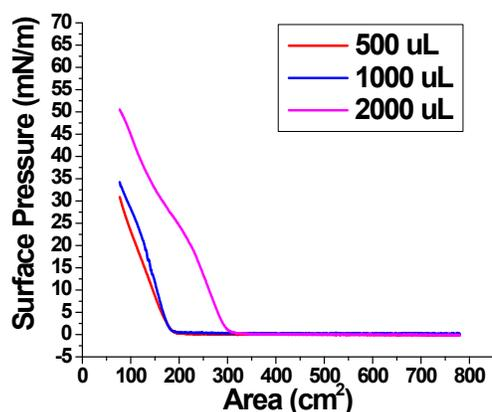
**Fig S3.**  $\pi$ -area isotherm of 500  $\mu\text{L}$ , 1000  $\mu\text{L}$  and 2000  $\mu\text{L}$  GO dispersed in 1:5 water: methanol mixture to a final concentration of 1 mg/mL. 2 mL of sample loading shows a well-define classic  $\pi$ -area isotherm (smooth gas to liquid to solid phase transitions) upon lateral compression.
