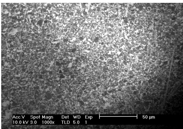
**Fig. S1.** SEM images of GO film deposited by LB. Note that the GO sheets are oriented flat on the surface of the substrate.
