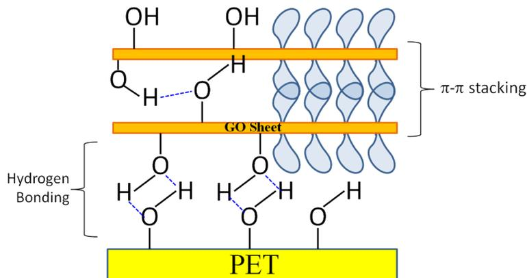
**Fig. S5.** Proposed explanation for the observed stability of GO sheets on PET substrates. The stability may be due to the strong hydrogen bonding of GO to the hydroxy groups of PET film. Secondly, as the number of layers was increased by repeated deposition, the  $\pi$ - $\pi$  stacking of the GO sheets may have contributed to the observed stability.
