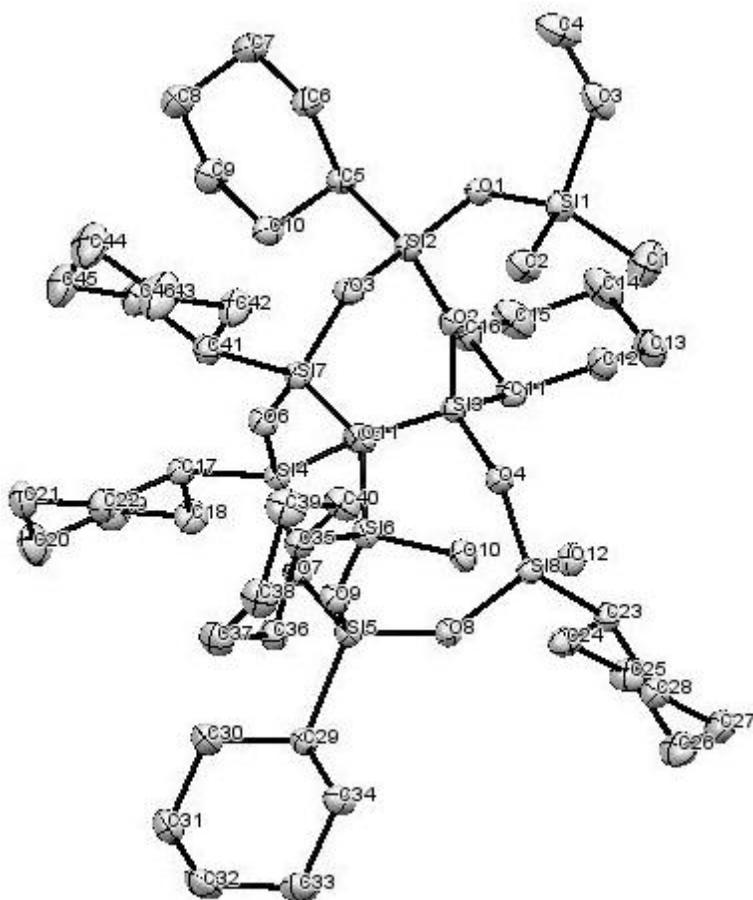
**Figure S2d.** ORTEP of POSS-*c*-hexyl-vinyl-(OH)<sub>2</sub> (2) showing 50% occupancy of the ellipsoid. Protons and minor distorting components atoms not shown for clarity.
