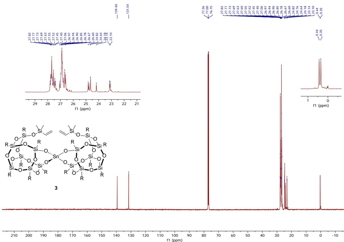
**Figure S4b.**  $^{13}\text{C}$  NMR spectra of **3** in  $\text{CDCl}_3$ . The resonances of the two diastereotopic methyl carbon of  $-\text{SiC}_2\text{H}_3\text{Me}_2$  are at  $\delta$  0.35 and 0.44 ppm.
