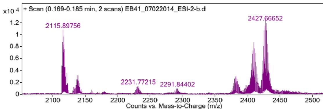
**Figure S4g.** ESI mass spectra of **3** in CDCl<sub>3</sub>. Peak at 2115.9 assigned to the loss of tin, and peak at 2427.7 to (M+3H<sub>2</sub>O+CDCl<sub>3</sub>+Na)<sup>+</sup> (*m/z* calcd for C<sub>93</sub>H<sub>178</sub>O<sub>27</sub>Si<sub>16</sub>SnCl<sub>3</sub>DNa 2426.70 (100%), 2427.70 (98%)).
