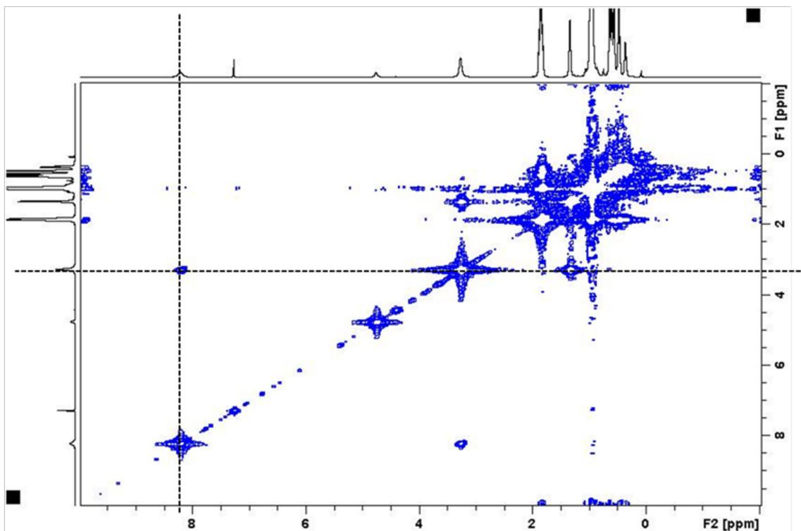
**Figure S1c.** COSY NMR (POSS-iBu<sub>7</sub>-Sn-Me)<sub>2</sub>·Et<sub>2</sub>NH·H<sub>2</sub>O dimer in CDCl<sub>3</sub> confirmed that the peak at  $\delta$  8.19 belong to Et<sub>2</sub>NH<sub>2</sub><sup>+</sup>.
