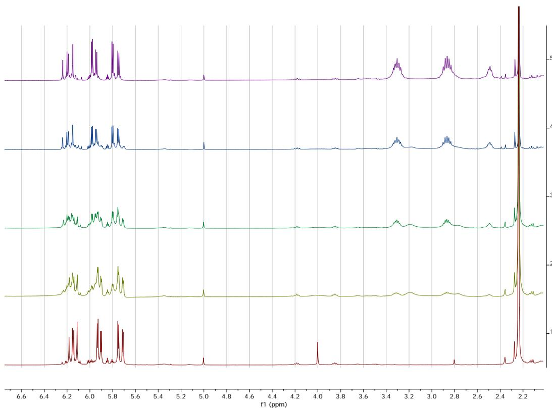
**Figure S6a.** <sup>1</sup>H NMR of **3** after addition of (from bottom to top) 0, 0.5, 1, 1.5 and 2 equivalents of Et<sub>2</sub>NH (the resonances of the vinyl protons of **3** (6.2-5.7 ppm), of the two diastereotopic protons of CH<sub>2</sub> (3.31 and 2.84 ppm) and of the NH (2.49 ppm) of **3**-bound Et<sub>2</sub>NH are shown).
