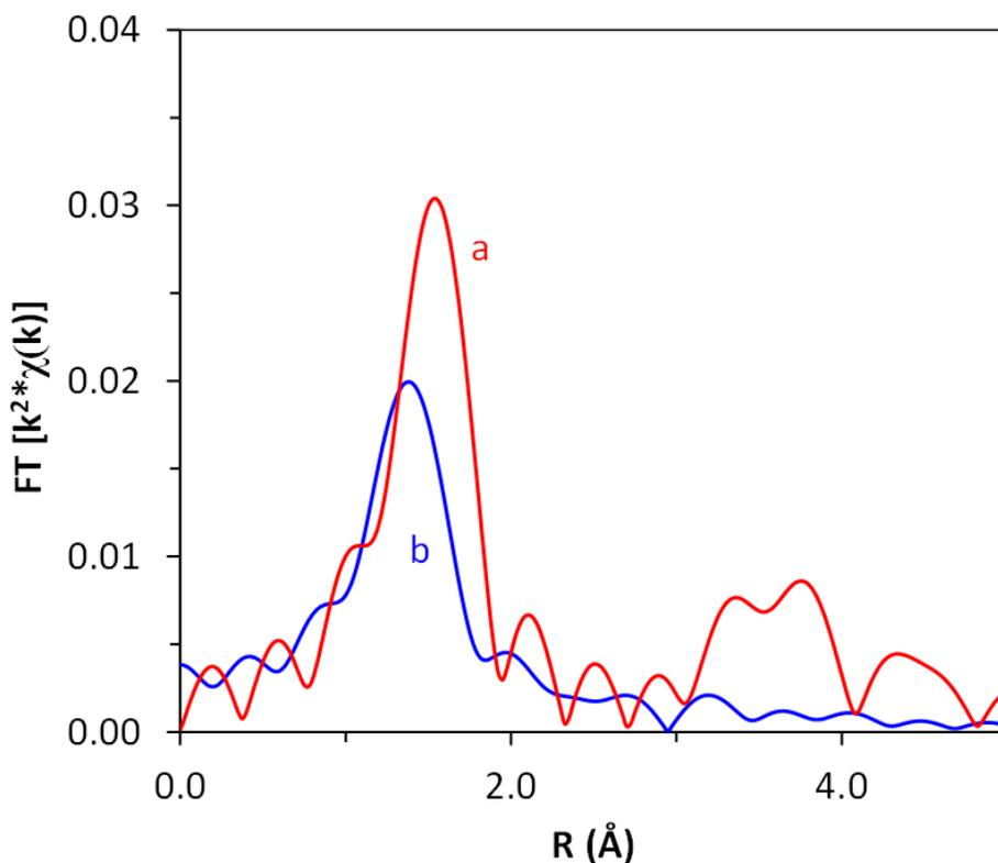
**Figure S5a.** Sn K-edge magnitude of the FT of the EXAFS of (a) SnO<sub>2</sub> and (b) compound **3** in toluene.  $k^2$ :  $\Delta k = 2.7$ - $10.2 \text{ \AA}^{-1}$ .
