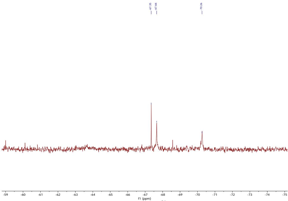
**Figure S8b.** The POSS-region expansion of the  $^{29}\text{Si}$  NMR of **3** after the addition of 32 eq. of  $\text{Et}_3\text{N}$  (all except three signals broadened or disappeared).
