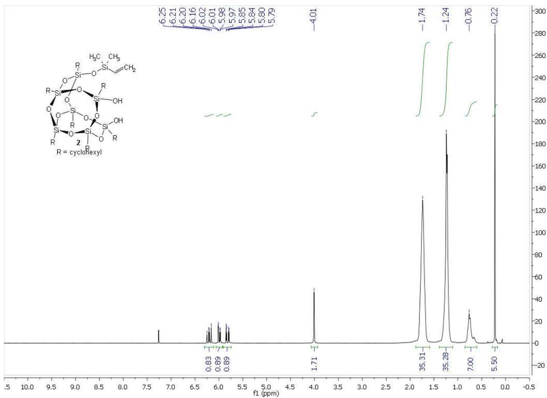
**Figure S2a.** <sup>1</sup>H NMR of compound **2** in CDCl<sub>3</sub>.
