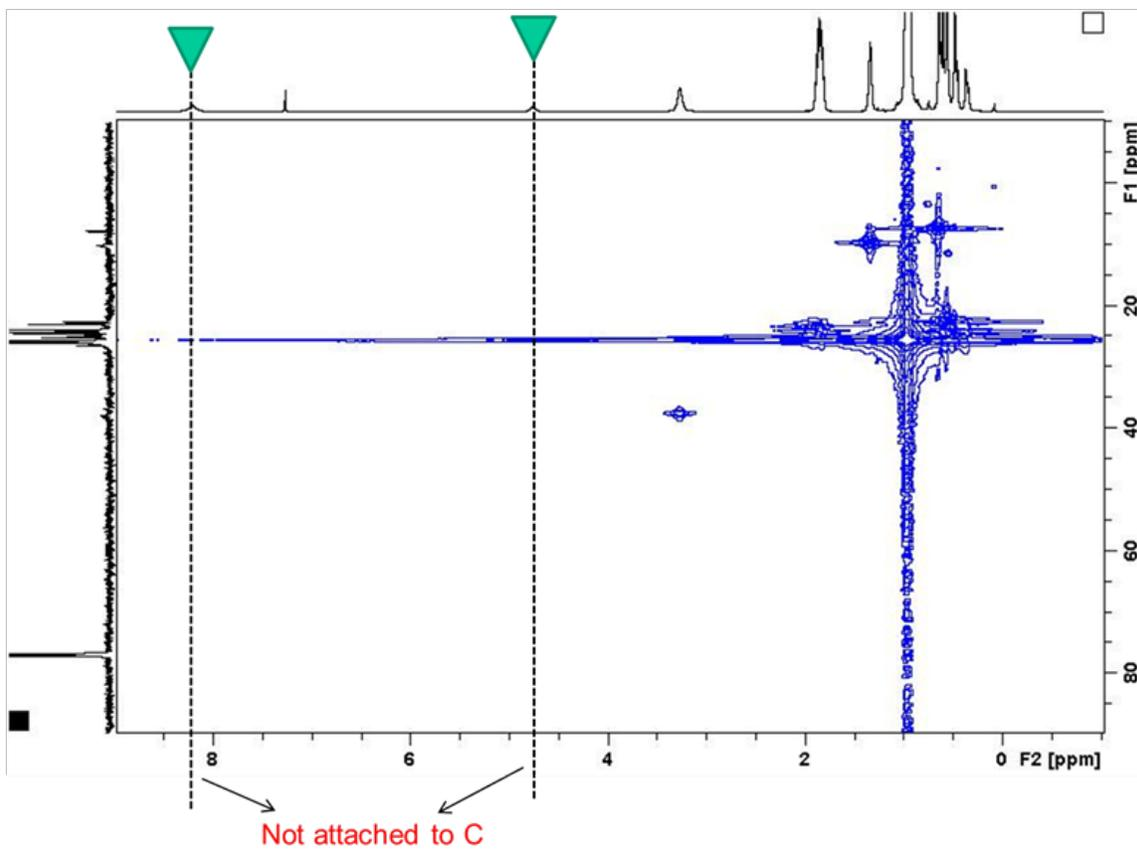
**Figure S1b.**  $^1\text{H}$ - $^{13}\text{C}$  HMQC NMR  $(\text{POSS-iBu}_7\text{-Sn-Me})_2\cdot\text{Et}_2\text{NH}\cdot\text{H}_2\text{O}$  dimer in  $\text{CDCl}_3$  confirmed that the two protons at ppm 8.19 and 4.75 were not attached to carbon.
