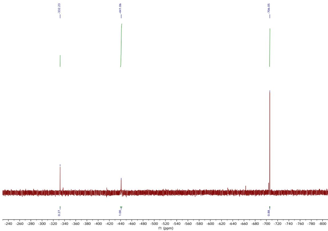
**Figure S6d.**  $^{119}\text{Sn}$  NMR of **3** after addition of 1 equivalent of  $\text{Et}_2\text{NH}$  (-332 ppm is an impurity peak that was present before the addition of  $\text{Et}_2\text{NH}$  and accounted for 12% of the total integrated intensity of the Sn peaks).
