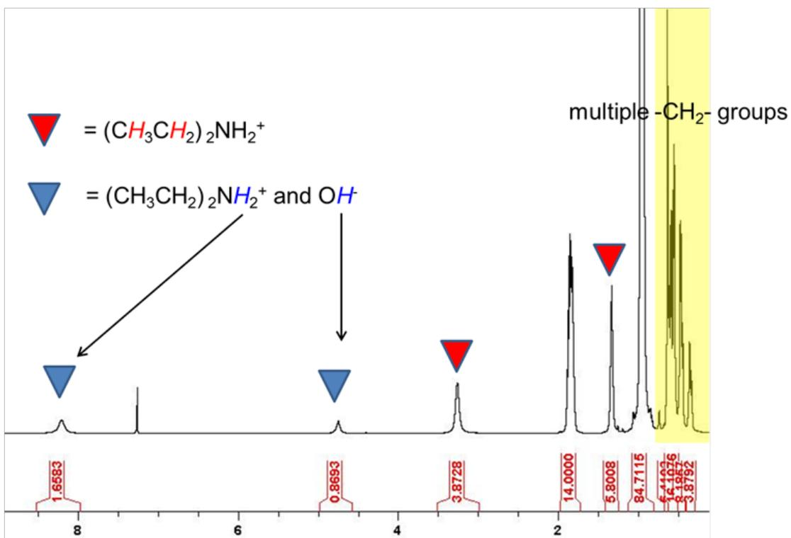
**Figure S1a.**  $^1\text{H}$  NMR  $(\text{POSS-iBu}_7\text{-Sn-Me})_2 \cdot \text{Et}_2\text{NH} \cdot \text{H}_2\text{O}$  dimer in  $\text{CDCl}_3$ .
