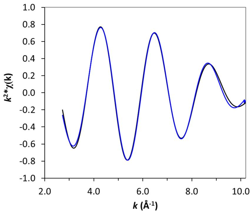
**Figure S5b.** Sn K-edge  $k^2$  weighted isolated first-shell Fourier transform data and fit of the EXAFS of compound **3** fitted using  $\text{SnO}_2$  as the reference. Black: experimental data; blue; fit.  $k^2$ :  $\Delta k = 2.7\text{-}10.2 \text{\AA}^{-1}$ .  $\Delta R = 1.1\text{-}1.8 \text{\AA}$ .
