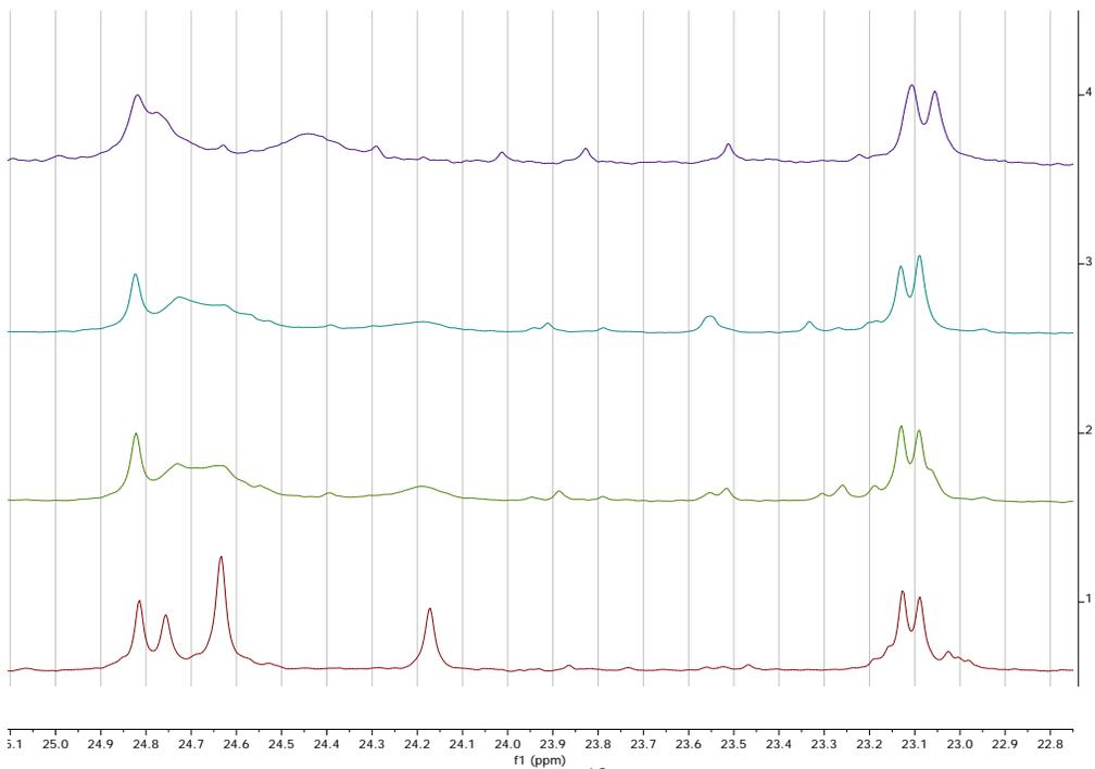
**Figure S8a.** Expanded CH-region of the  $^{13}\text{C}$  NMR of **3** after addition of (from bottom to top) 0, 1, 2, and 32 equivalents of  $\text{Et}_3\text{N}$ .
