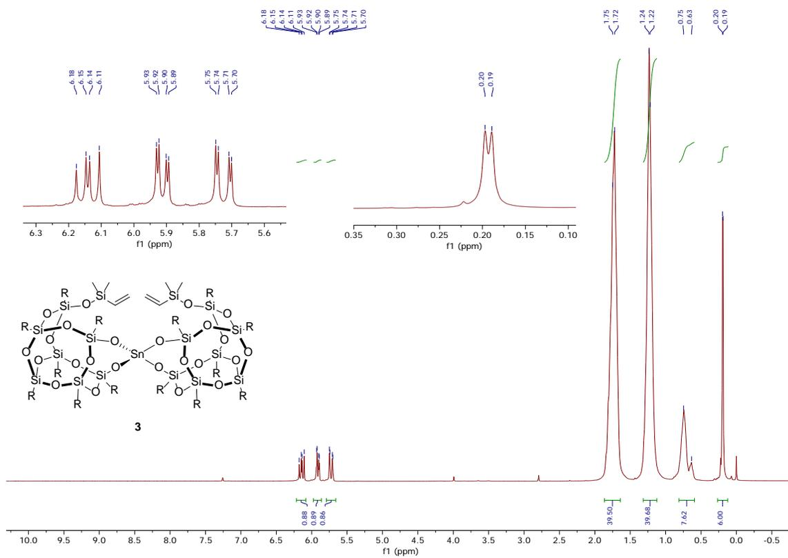
**Figure S4a.**  $^1\text{H}$  NMR spectra of **3** in  $\text{CDCl}_3$ . The resonances of the two diastereotopic methyl carbon of  $-\text{SiC}_2\text{H}_3\text{Me}_2$  are at  $\delta$  0.19 and 0.20 ppm.
