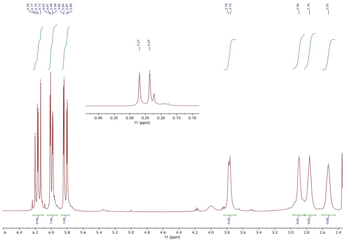
**Figure S7a.** <sup>1</sup>H NMR of **3** after addition of 1 equivalent of ethylenediamine (the signals of the vinyl (6.2-5.8 ppm), methyls (inset) and the two pairs of diastereotopic protons of CH<sub>2</sub>'s and NH<sub>2</sub>'s (3.8-2.4 ppm) of **3**•H<sub>2</sub>NCH<sub>2</sub>CH<sub>2</sub>NH<sub>2</sub> are shown).
