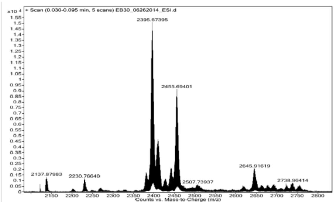
**Figure S4f.** ESI mass spectra of **3** in CH<sub>2</sub>Cl<sub>2</sub>. Peak at 2396 assigned to (M-Sn<sup>4+</sup>+3H<sup>+</sup>-H<sub>2</sub>O+Na<sup>+</sup>+3CH<sub>2</sub>Cl<sub>2</sub>)<sup>+</sup> and 2456 to (M+3H<sub>2</sub>O+2CH<sub>2</sub>Cl<sub>2</sub>)<sup>+</sup>.
