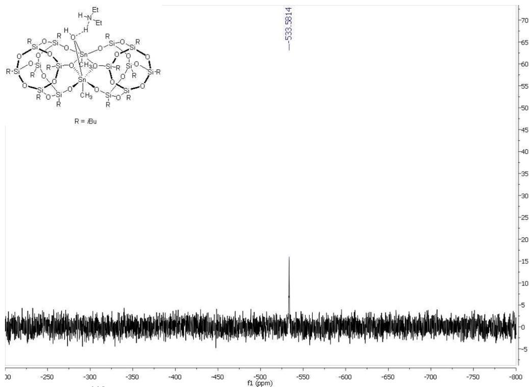
**Figure S1d.**  $^{119}\text{Sn}$  NMR of  $(\text{POSS-iBu}_7\text{-Sn-Me})_2 \cdot \text{Et}_2\text{NH} \cdot \text{H}_2\text{O}$  dimer.
