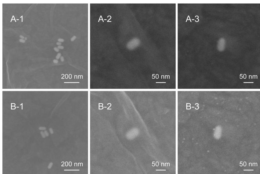
**Fig. S5.** Scanning electron microscope images of gold nanorods covered by (A) graphene oxide and (B) electrochemically reduced graphene oxide.
