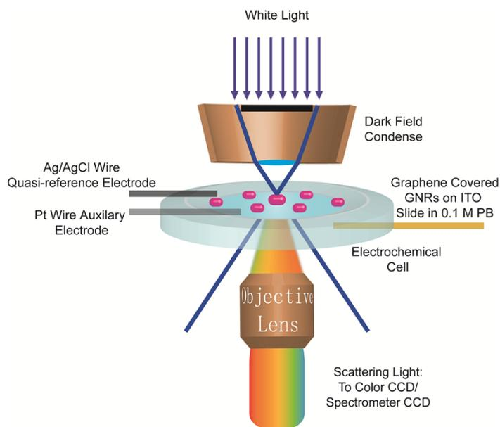
**Fig. S1.** Experimental configuration of the dark-field microscopy and plasmon resonance Rayleigh scattering spectroscopy, and the setup of the electrochemical cell.
