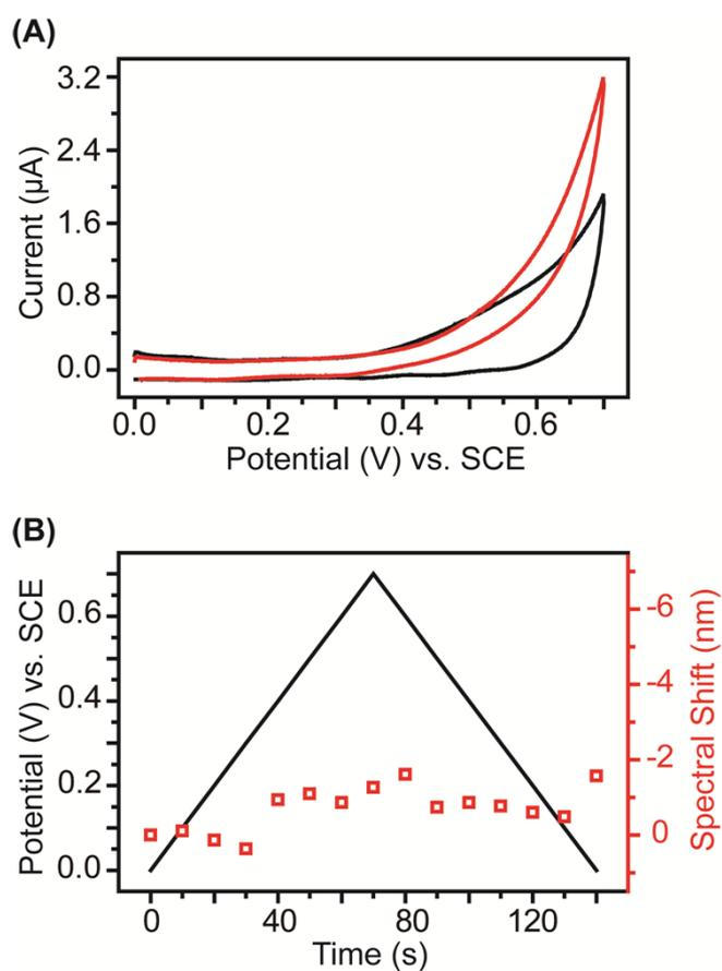
**Fig. S6.** Plasmonic shift of single gold nanorod synchronized with voltammetry on GNRs/APTES/ITO electrode. (A) Cyclic voltammograms recorded at 10 mV/s in the absence (black line) and presence (red line) of 3.0 mM NADH. (B) Faradaic current (black line) and spectral shift (red triangle) as a function of applied potential and time.
