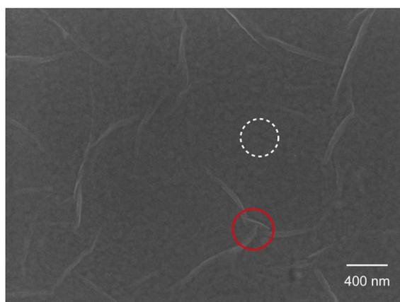
**Fig. S8.** Scanning electron microscope images of silanized ITO covered by graphene oxide. Red and white circles show nanoscale difference of the graphene oxide film.
