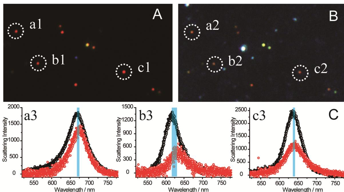
**Fig. S4.** Typical dark field microscopy images (A-B) and plasmon resonance Rayleigh scattering spectra (C) of single GNRs before and after the modification of graphene oxide. a1-c1: DFM of single GNRs on silanized ITO. a2-c2: DFM of GO covered single GNRs on silanized ITO. a3-c3: PRRS of bare (black) and GO covered (red) GNRs.
