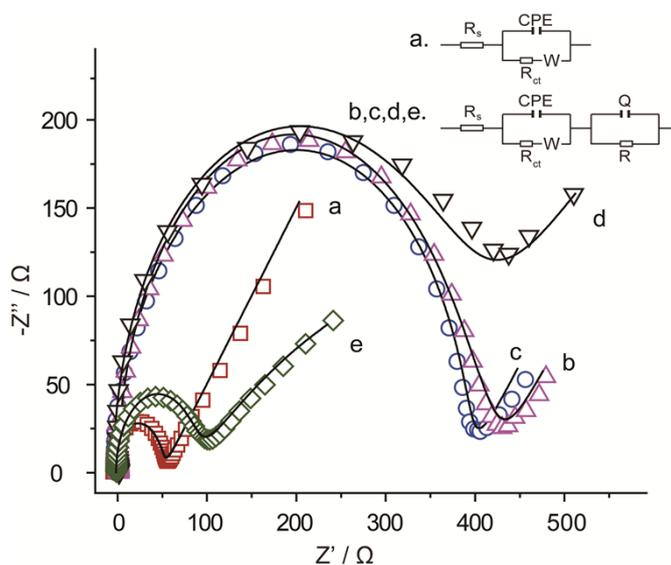
**Fig. S2.** Electrochemical impedance plots in the presence of 5 mM  $\text{Fe}(\text{CN})_6^{3-}$  and 5 mM  $\text{Fe}(\text{CN})_6^{4-}$  containing 0.1 M KCl on ITO electrodes: (a) bare ITO, (b) APTES/ITO, (c) GNRs/APTES/ITO, (d) GO/GNRs/APTES/ITO and (e) erGO/GNRs/APTES/ITO electrodes.
