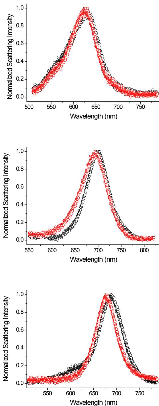
**Fig. S7.** The PRRS spectra of single GNRs overcoated with  $10 \mu\text{g}/\text{cm}^2$  GO (black) or erGO (red). The erGO were formed by scanning the GO covered GNRs/ITO from 0 to -0.8 V for 100 cycles, in phosphate buffer solution.
