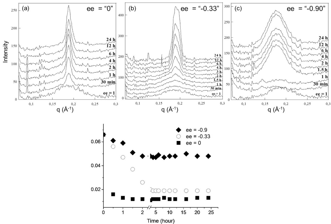
SAXS intensities as a function of time for  $ee = "0"$ ,  $"-0.33"$ ,  $"-0.9"$ , and FWHM of the SAXS peak at  $q \sim 0.185 \text{ \AA}^{-1}$  with  $ee$  from 1 to 0, 1 to  $-0.33$ , 1 to  $-0.60$  and 1 to  $-0.90$
