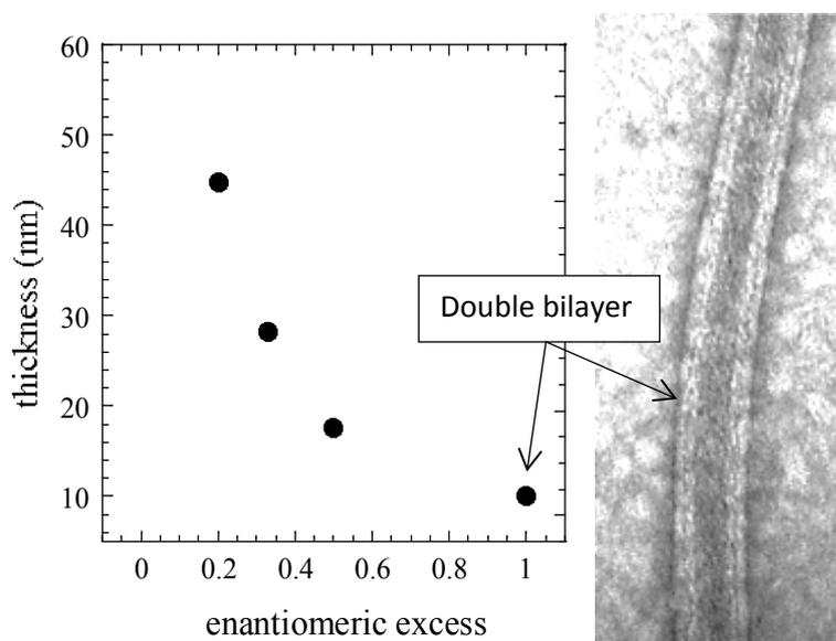
The membrane thickness (number of bilayers  $\sim$  thickness/5 nm) of chiral fiber of 16-2-16 tartrate increase with decreasing ee. The TEM image shows the tubules (ee=1) formed with double bilayers
