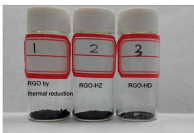
**Fig. S1** Digital image of RGO prepared by thermal reduction<sup>8</sup> (1) and RGO by hydrazine reduction (denoted as RGO-Hz) according to literature<sup>9,10</sup> (2) and RGO-HD (3) with same weight (20mg).
