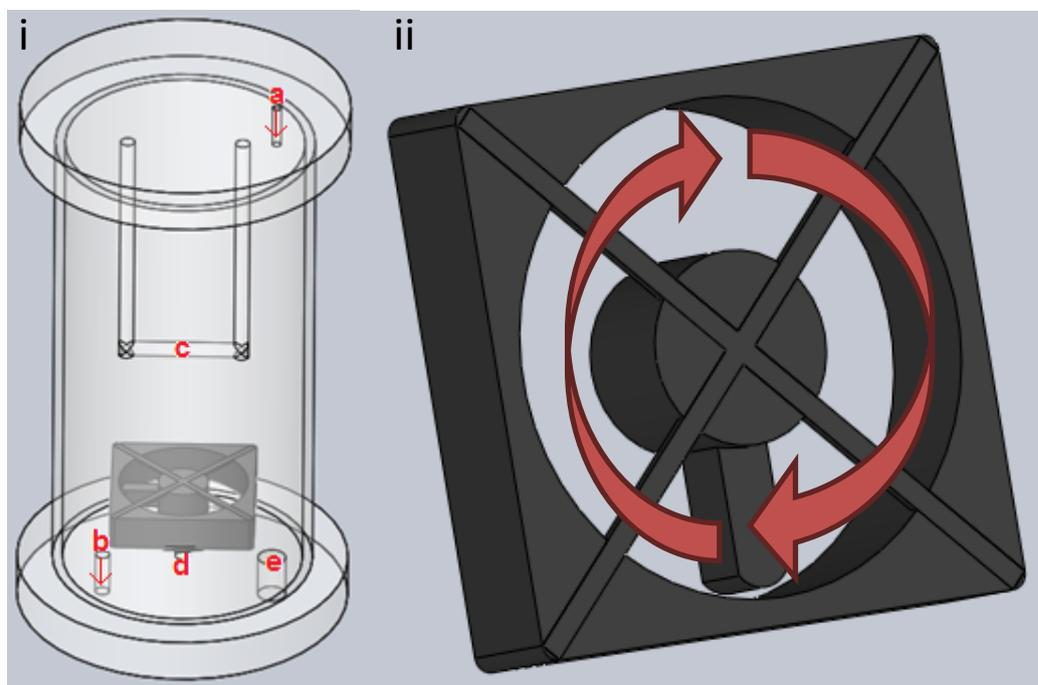
FIG. S1. i) Schematic of plasma reactor setup with additional DC power input and off-centre weighted motor for inducing shaking motion a) monomer inlet b) monomer outlet c) RF cathode d) RF anode with attached motor e) DC power in port. ii) Schematic of shaking motor.
