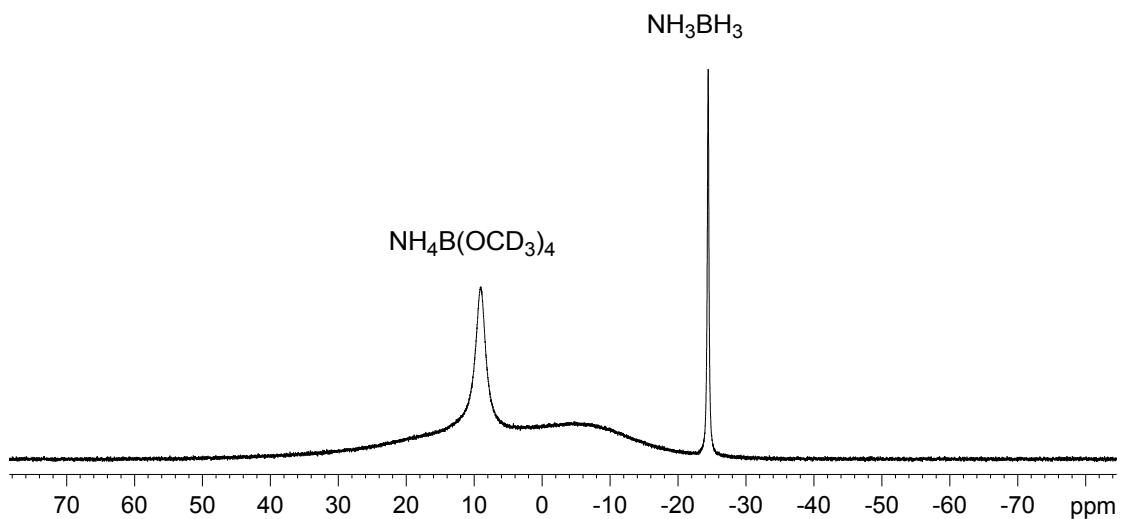
$^{11}\text{B}$  NMR during the progress of reaction (~50% conversion) showing  $\text{NH}_4\text{B}(\text{OCD}_3)_4$  and reacting  $\text{NH}_3\text{BH}_3$ .
