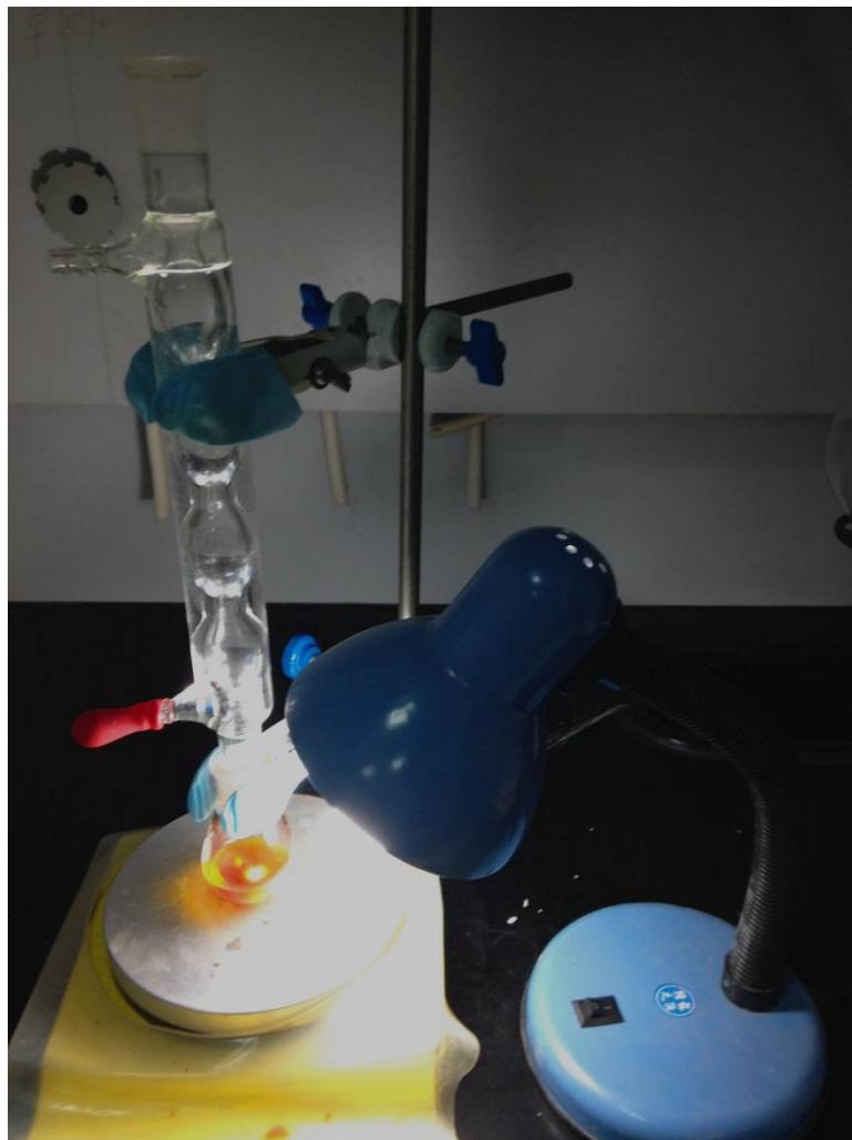
Figure S2. A picture for the setup of visible light induced reaction.
