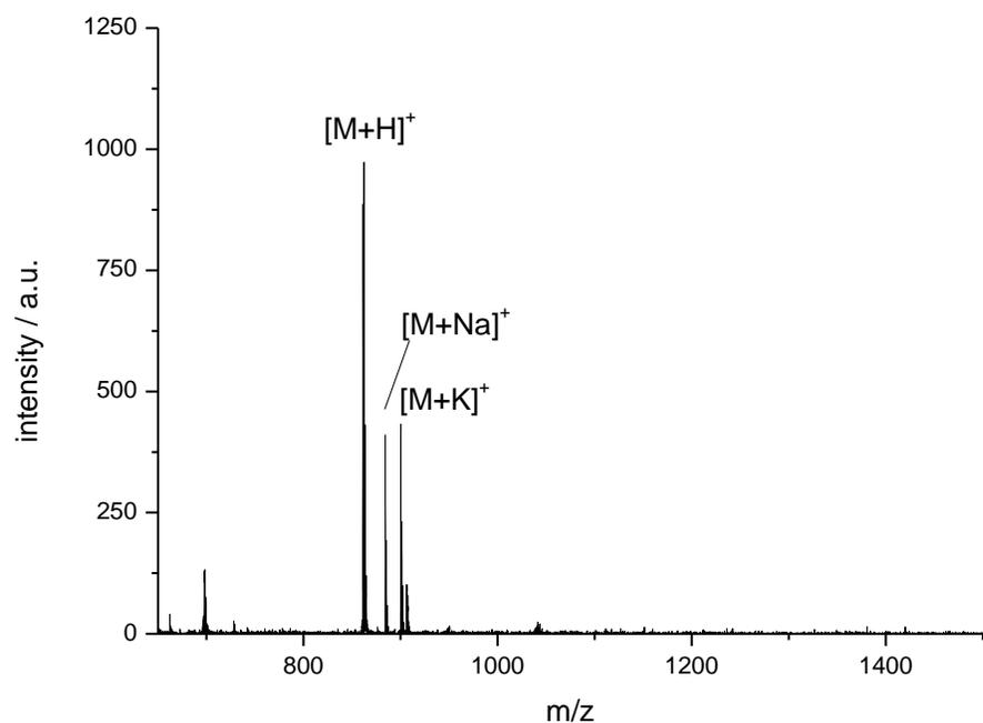
**Fig. S7** MALDI mass spectrum of **5** (matrix: DCTB in chloroform, positive mode).
