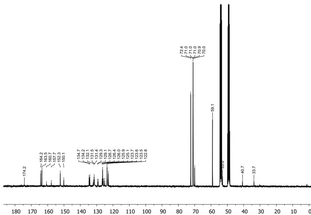
**Fig. S10**  $^{13}\text{C}$  NMR spectrum of **6** (CD<sub>2</sub>Cl<sub>2</sub>/MeOD 5:1, 101 MHz, 300 K).
