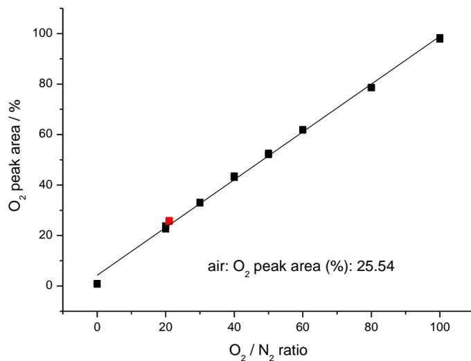
**Fig. S19** Gas chromatography calibration curve for different oxygen/nitrogen mixtures (red square marks the natural composition of air).
