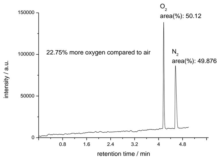
**Fig. S20** Exemplary gas chromatogram measured via injection of 500  $\mu$ L of the gas head space after the water oxidation using **6** a catalyst at a concentration of 96  $\mu$ M.
