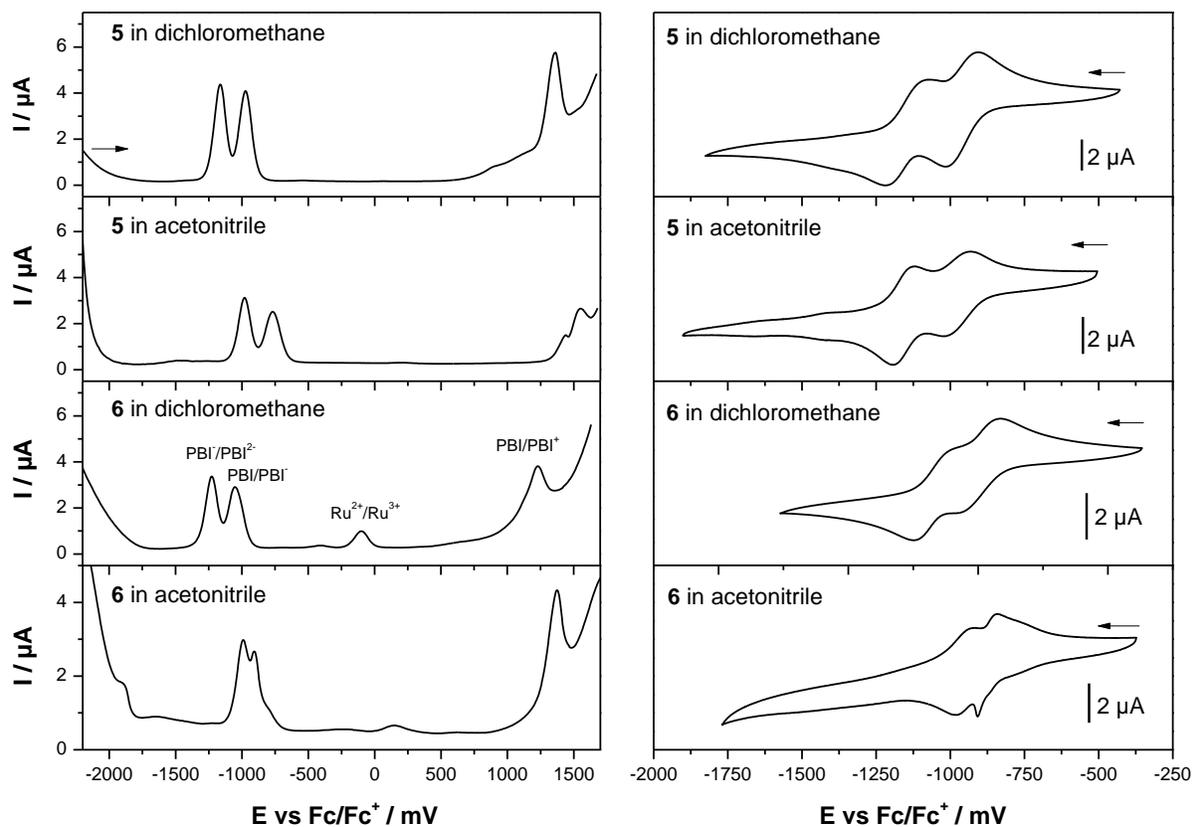
**Fig. S15** Left: Differential pulse voltammograms of **5** and **6** in dichloromethane and acetonitrile, respectively. Right: Cyclic voltammograms for **5** and **6** in dichloromethane and acetonitrile, respectively. The concentration of **5** and **6** for all measurements was  $2 \times 10^{-4}$  M and the scan rate 100 mV/s. TBAHFP was used in all cases as supporting electrolyte at a concentration of 0.1 M.
