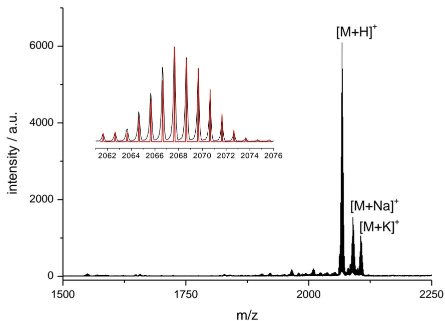
**Fig. S12** HR-ESI mass spectrum of **6** measured from chloroform/acetonitrile (positive mode). The inset shows the isotopic distribution of the  $[M+H]^+$  peak (black = measured, red = calculated).
