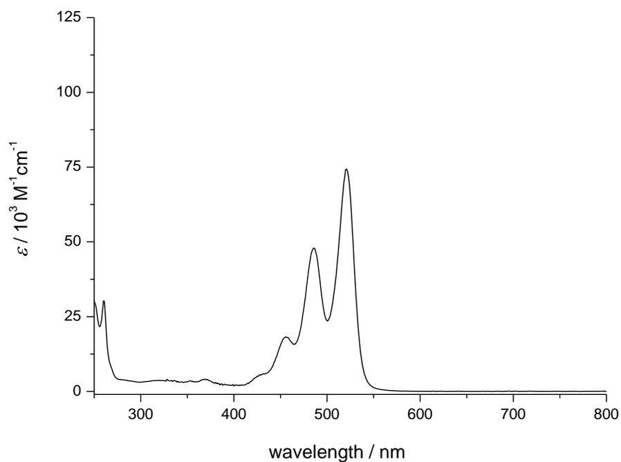
**Fig. S13** UV/vis absorption spectrum of **5** in acetonitrile at a concentration of  $10^{-5}$  M.
