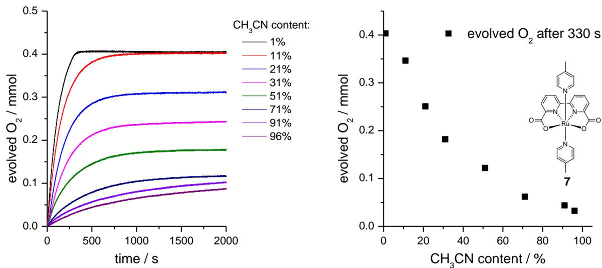
**Fig. S18** Catalytic activity of reference **7** ( $c = 75.5 \mu\text{M}$ ) depending on the acetonitrile content in the reaction mixture. With increased acetonitrile content the oxygen evolution is significantly slowed down. The catalyst solution (400  $\mu\text{L}$ , acetonitrile/water (pH 7) 1:9) was injected into a reaction vial filled with 1 g (1.82 mmol) CAN dissolved in 3 mL of the corresponding acetonitrile/water (pH 1) mixture.
