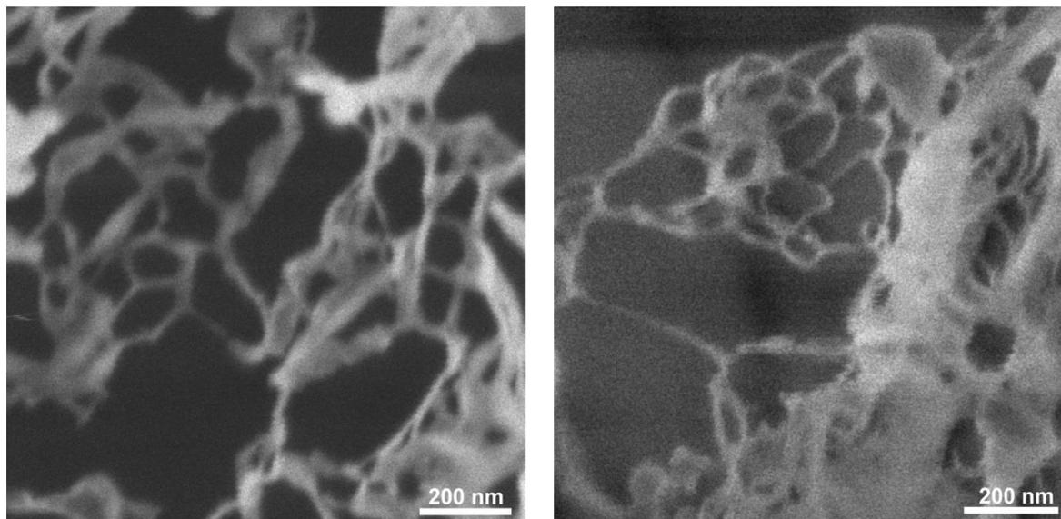
**Fig. S17** Cryo-SEM images of a solution of **6** in an acetonitrile/water 1:1 mixture ( $c = 10^{-5}$  M).
