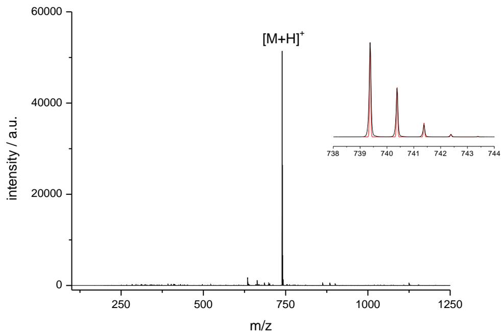
**Fig. S4** HR-ESI mass spectrum of **2** measured from chloroform/acetonitrile (positive mode). The inset shows the isotopic distribution of the  $[M+H]^+$  peak (black = measured, red = calculated).
