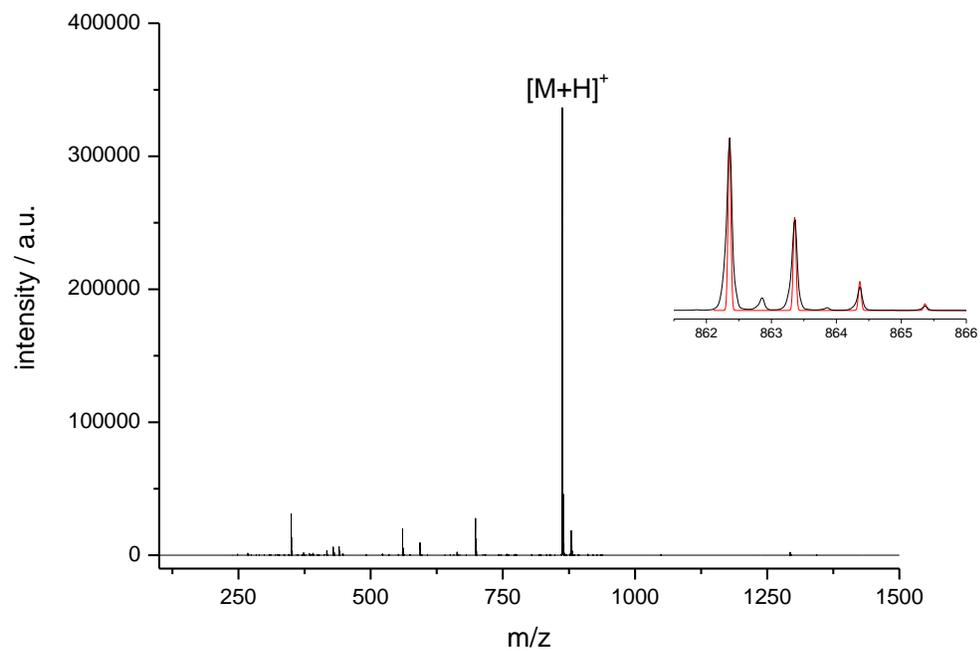
**Fig. S8** HR-ESI mass spectrum of **5** measured from chloroform/acetonitrile (positive mode). The inset shows the isotopic distribution of the  $[M+H]^+$  peak (black = measured, red = calculated).
