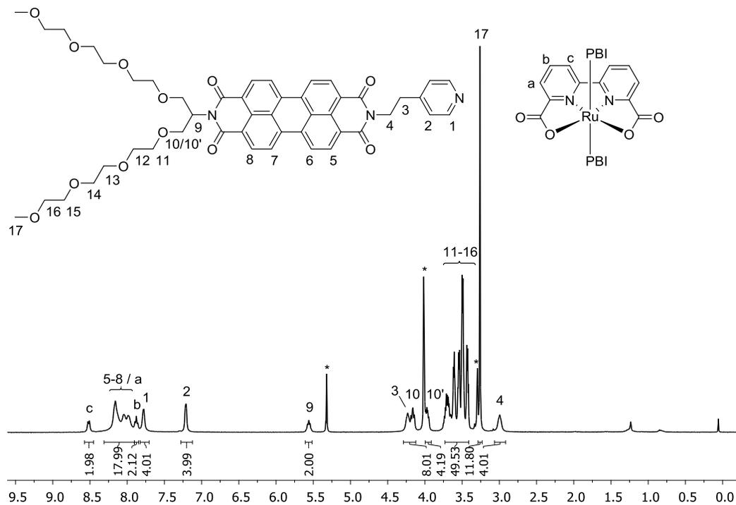
**Fig. S9**  $^1\text{H}$  NMR spectrum of **6** (CD<sub>2</sub>Cl<sub>2</sub>/MeOD 5:1, 400 MHz, 300 K). Peaks labelled with \* derive from the solvent.
