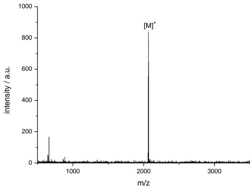
**Fig. S11** MALDI mass spectrum of **6** (matrix: DCTB in chloroform, positive mode).
