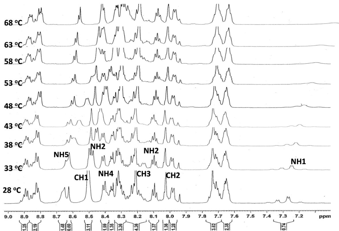
**Figure S14.** Variable temperature  $^1\text{H}$  NMR spectra of **Pentapeptide 5** in  $d_6$ -DMSO showing temperature dependence of amide-NH/triazole-CH chemical shift.
