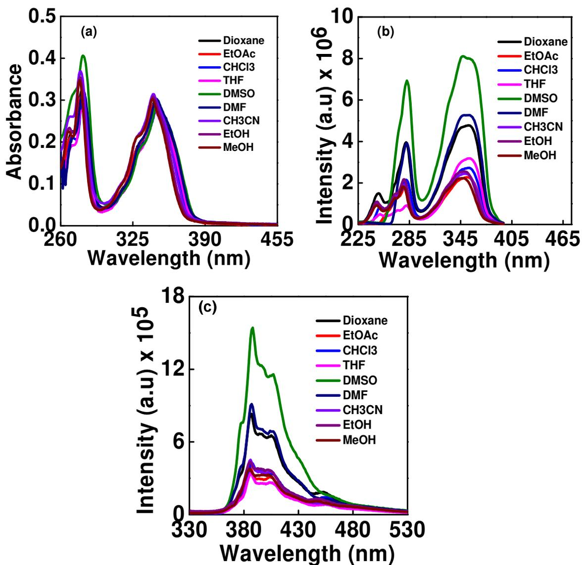
**Figure S27.** UV-Visible (a), excitation (b), and fluorescence emission spectra (c) of **Dipeptide 40** [Boc<sup>TPy</sup>Ala<sup>Do</sup>-Leu-CO<sub>2</sub>Me; Considered as the only Acceptor Chromophore in FRET study] in different solvents [10 μM, r.t.;  $\lambda_{\text{ex}} = \lambda_{\text{max}} \approx 345$  nm in each solvent].
