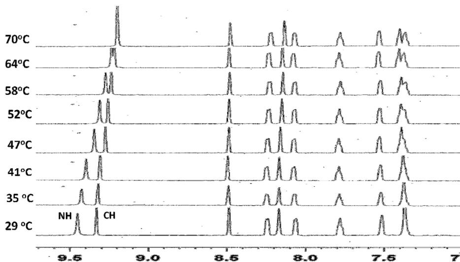
**Figure S8.** Variable Temperature  $^1\text{H}$  NMR spectra of **2**,  $\text{ArTAA}$  in  $d_6$ -DMSO showing temperature dependence of amide-NH/triazole-CH chemical shift.
