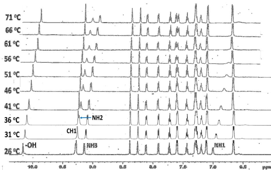
Figure S12. Variable temperature  $^1\text{H}$  NMR spectra of **Tripeptide 4** in  $\text{d}_6\text{-DMSO}$  showing temperature dependence of amide-NH/triazole-CH chemical shift.
