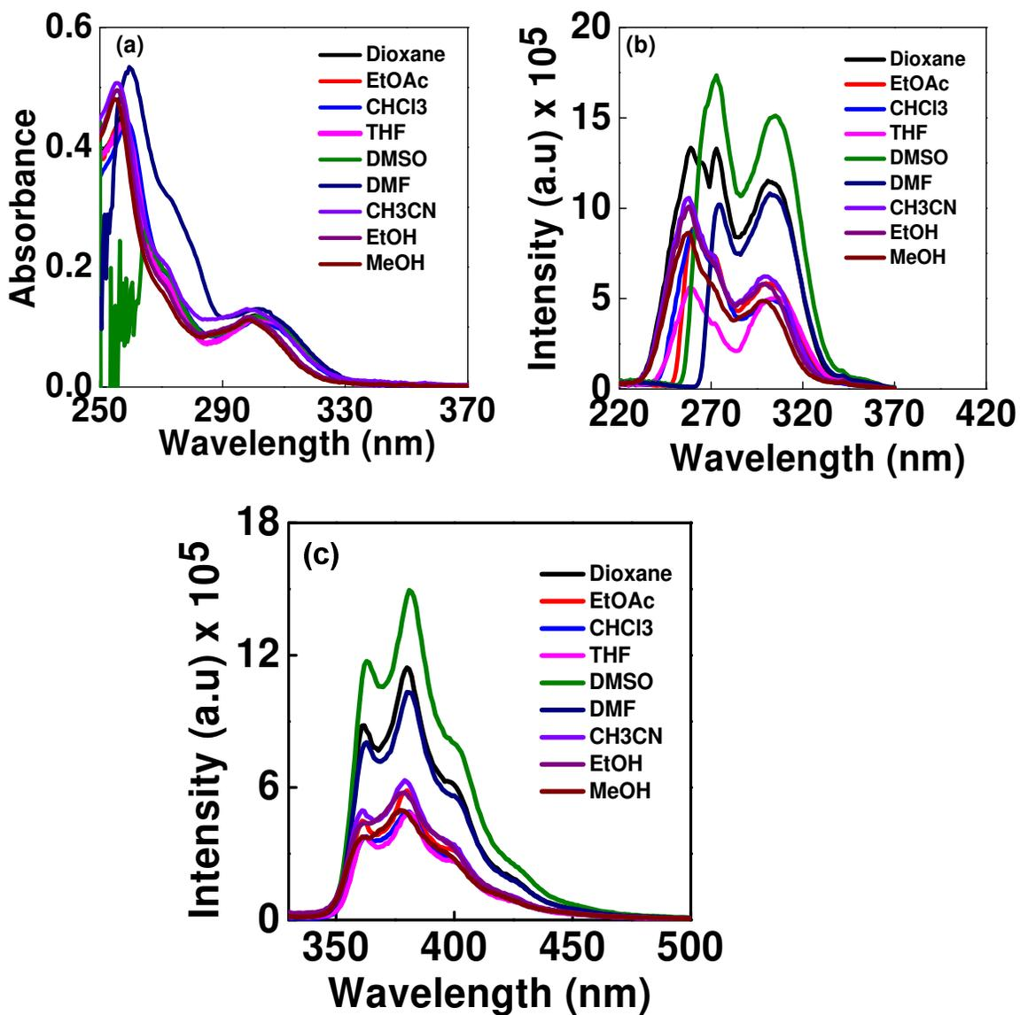
**Figure S26.** UV-Visible (a), excitation (b), and fluorescence emission spectra (c) of **Dipeptide 34** [BocLeU-<sup>T</sup>PhenAla-CO(NMe)OMe; Considered as the only Donor Chromophore in FRET study] in different solvents [10  $\mu$ M, r.t.;  $\lambda_{\text{ex}} = \lambda_{\text{max}} \approx 300$  nm in each solvent].
