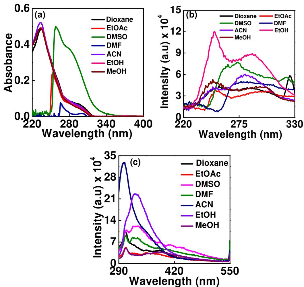
**Figure S25.** UV-Visible (a), excitation (b), and fluorescence emission spectra (c) of the **Aromatic Amino Acid Scaffold 2** [ $\text{BocNH-ArTAA-CO}_2\text{H}$ ] in different solvents [ $10 \mu\text{M}$ , r.t.;  $\lambda_{\text{ex}} = \lambda_{\text{max}} \approx 280 \text{ nm}$  in each solvent].
