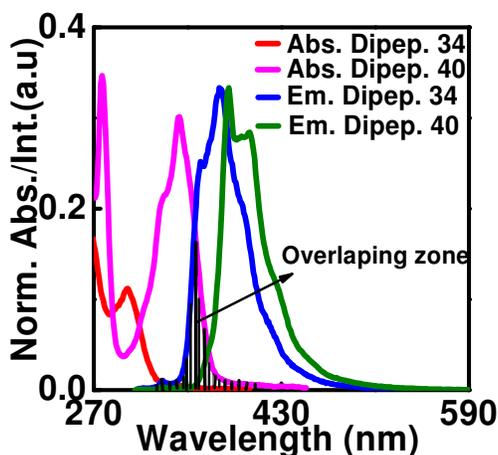
**Figure S29.** (a) Overlapping of emission spectra of **Dipeptide containing fluorescent amino acid**  $^{\text{TPhen}}\text{Ala}^{\text{Do}}$  (**34**) (act as a FRET donor) and the absorption spectra of **Dipeptide containing fluorescent amino acid**  $^{\text{TPy}}\text{Ala}^{\text{Do}}$  (**40**) (act as a FRET acceptor) (10  $\mu\text{M}$  each, r.t.;  $\lambda_{\text{ex}} = 300$  nm in  $\text{CH}_3\text{OH}$ ).
