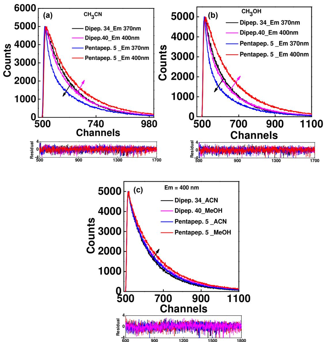
**Figure S31.** Time resolved fluorescence and corresponding residual spectra of **Dipeptide 34, 40** and **pentapeptide 5** using (a) 293 LED in acetonitrile (b) 293 LED in methanol and (c) 343 LED in both the solvent (1ns = 10 chan.).
