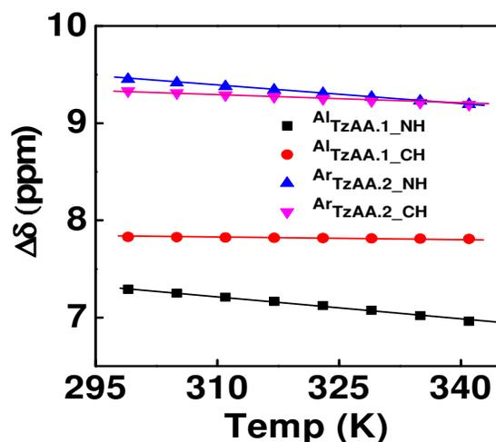
**Figure S6.** Temperature dependence of amide-NH/triazole-CH chemical shift of 1,  $^{\text{Al}}\text{TzAA}$  and 2,  $^{\text{Ar}}\text{TAA}$ .
