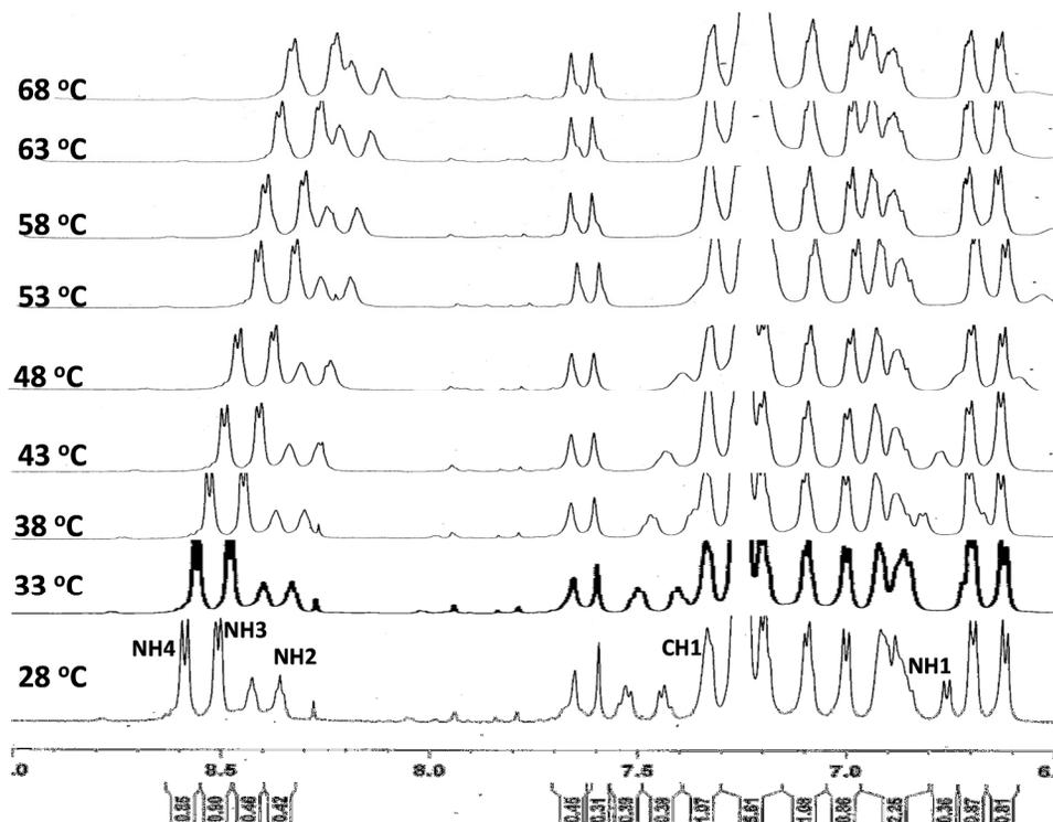
**Figure S10.** Variable temperature  $^1\text{H}$  NMR spectra of **tetrapeptide 4** in  $d_6$ -DMSO showing temperature dependence of amide-NH/triazole-CH chemical shift.
