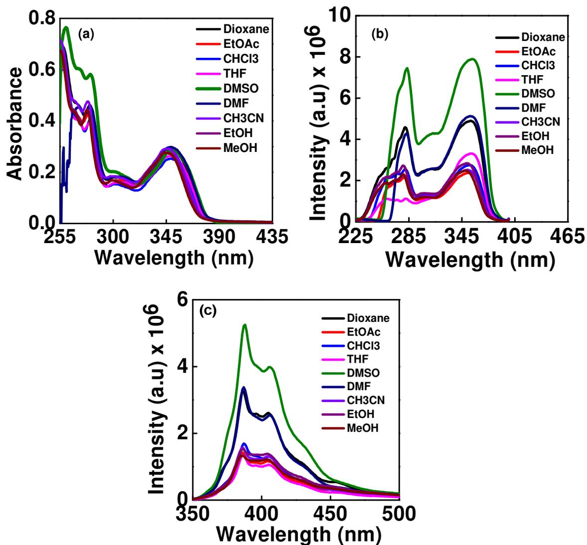
**Figure S28.** UV-Visible (a), excitation (b), and fluorescence emission spectra (c) of Fluorescent Pentapeptide 5 [Boc<sup>TPy</sup>Ala<sup>Do</sup>-Leu-<sup>Al</sup>TAA-Leu-<sup>TPhen</sup>Ala<sup>Do</sup>-CO<sub>2</sub>Me] in different solvents [10  $\mu$ M, r.t.;  $\lambda_{\text{ex}} = \lambda_{\text{max}} \approx 300$  and 345 nm in each solvent].
