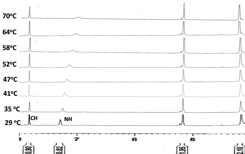
**Figure S7.** Variable temperature  $^1\text{H}$  NMR spectra of **1**,  $\text{ArTAA}$  in  $d_6$ -DMSO showing temperature dependence of amide-NH/triazole-CH chemical shift.
