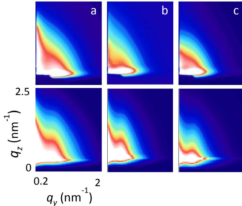
**Fig. S5** GISAXS data (first row) and simulated GISAXS patterns (second row) of the IGZO film annealed at 300°C (a), 380°C (b), and 450°C (c).
