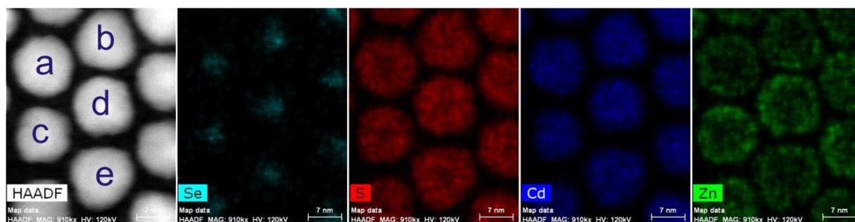
**Fig. S1** CdSe/CdS/ZnS core/multishell QDs at initial state. Marked QDs were used for elemental quantification.
