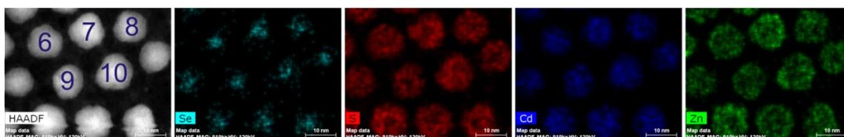
**Fig. S4** QDs at heated state ( $\text{Cd}_x\text{Zn}_{1-x}\text{Se}/\text{Cd}_y\text{Zn}_{1-y}\text{S}$  core/shell QDs). Marked QDs were used for elemental quantification.
