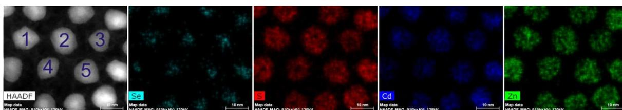
**Fig. S3** QDs at heated state ( $\text{Cd}_x\text{Zn}_{1-x}\text{Se}/\text{Cd}_y\text{Zn}_{1-y}\text{S}$  core/shell QDs). Marked QDs were used for elemental quantification.
