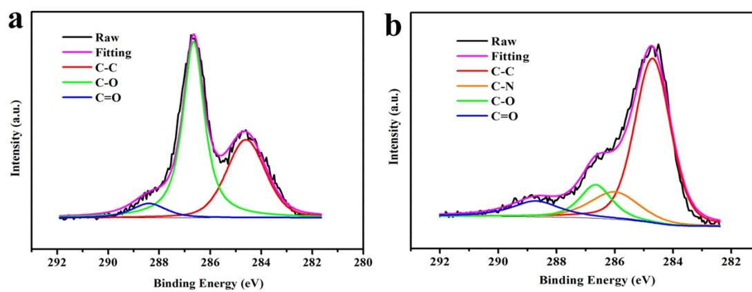
Fig. S5 C1s XPS spectra of GO (a) and SnO<sub>2</sub>/N-doped graphene composite (b).
