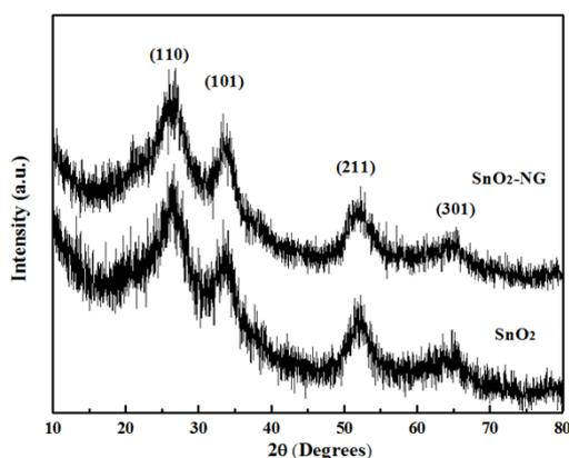
Fig. S1 XRD patterns of  $\text{SnO}_2$  nanocrystals and  $\text{SnO}_2/\text{N}$ -doped graphene composite.
