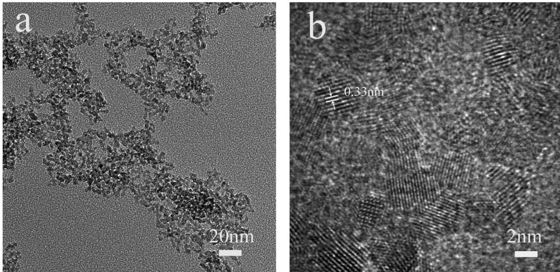
**Fig. S2** TEM (a) and HRTEM (b) images of SnO<sub>2</sub> nanocrystals.
