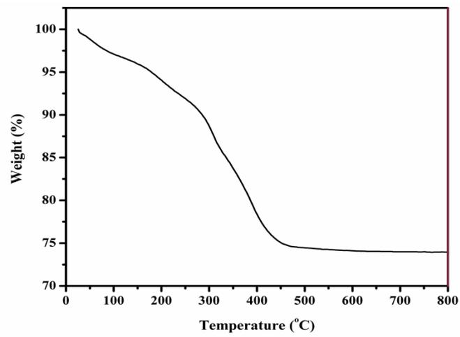
**Fig. S3** TGA curve of SnO<sub>2</sub>/N-doped graphene composite.
