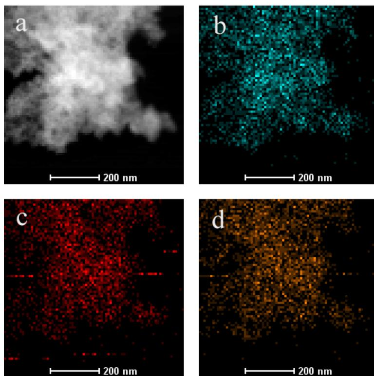
Fig. S4 STEM image (a), Sn (b), C (c) and N (d) elemental mappings of SnO<sub>2</sub>/N-doped graphene composite.
