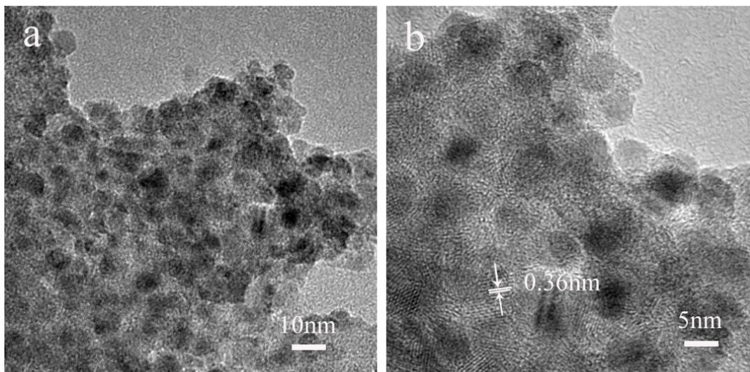
**Fig. S6 TEM (a) and HRTEM (b) images of SnO<sub>2</sub>/N-doped graphene composite electrode after 1C cycling.**
