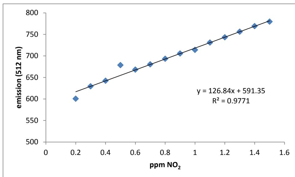
Figure S-8. Emission at 512 nm of **2**+NO<sub>2</sub> (1.0 x 10<sup>-5</sup>M in acetonitrile) *versus* increasing amounts of NO<sub>2</sub> at room temperature.
