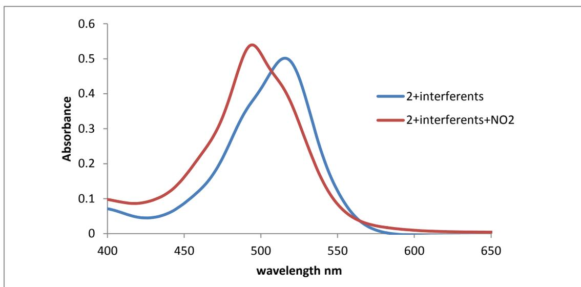
Figure S-9. UV spectra of probe **2**+interferents (CO<sub>2</sub>+NO+H<sub>2</sub>S+SO<sub>2</sub>) and probe **2** in the presence of interferents plus NO<sub>2</sub>.
