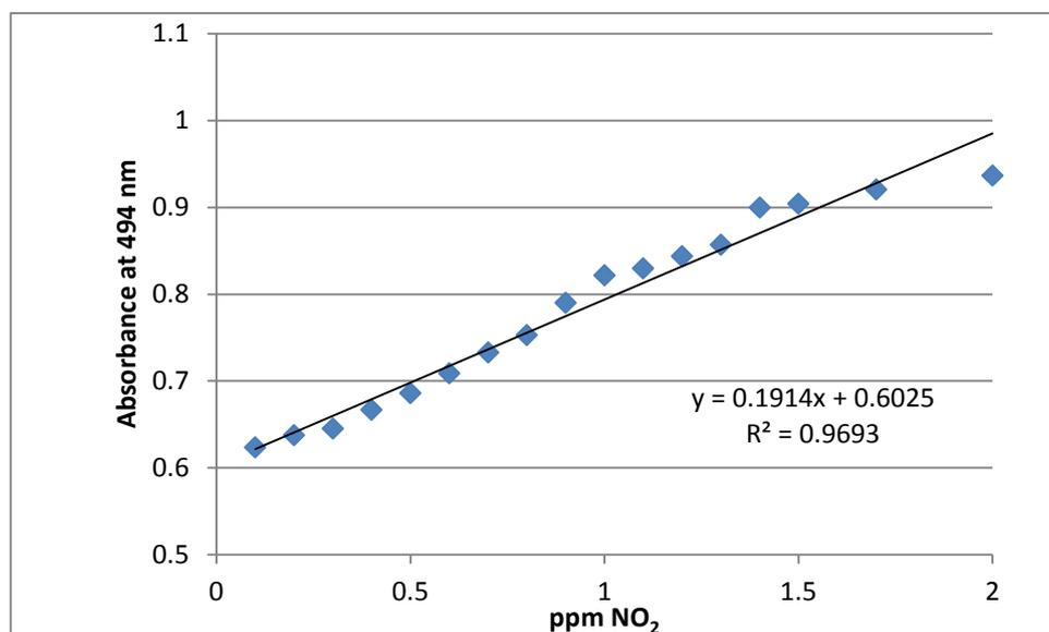
Figure S-7. Absorbance at 494 nm of **2**+NO<sub>2</sub> (1.0 x 10<sup>-5</sup>M in acetonitrile) *versus* increasing amounts of NO<sub>2</sub> at room temperature.
