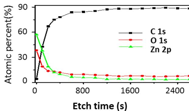
**Figure S2.** XPS etch profile for C 1s, O 1s, and Zn 2p orbitals in the ZnGO specimen.
