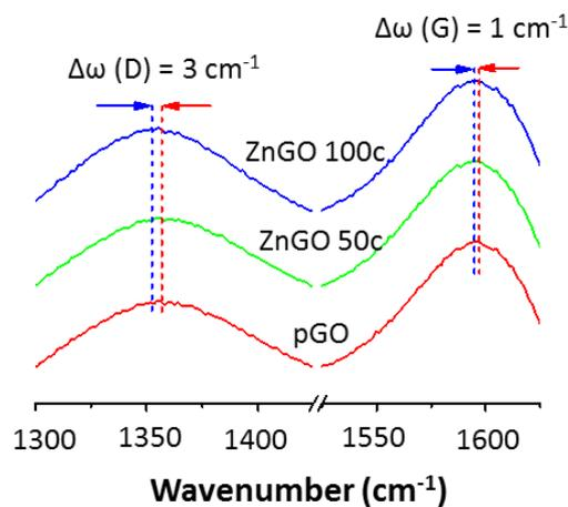
**Figure S4.** Raman spectra of diverse GO membranes upon different ALD cycles.
