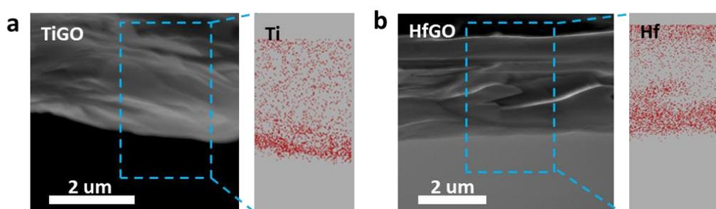
**Figure S1.** (a, b) Left side is the SEM images of Ti-impregnated GO (TiGO) and Hf-impregnated GO (HfGO); (a, b) Right side is its corresponding EDX mapping of Ti and Hf, respectively.
