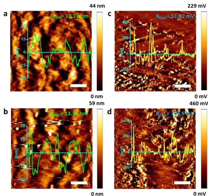
**Figure S3** (a-b) AFM topographic images and height profiles of pGO and ZnGO; (c-d) The corresponding AFM lateral force images and voltage profiles of pGO and ZnGO, respectively. Scale bar = 1  $\mu\text{m}$ .
