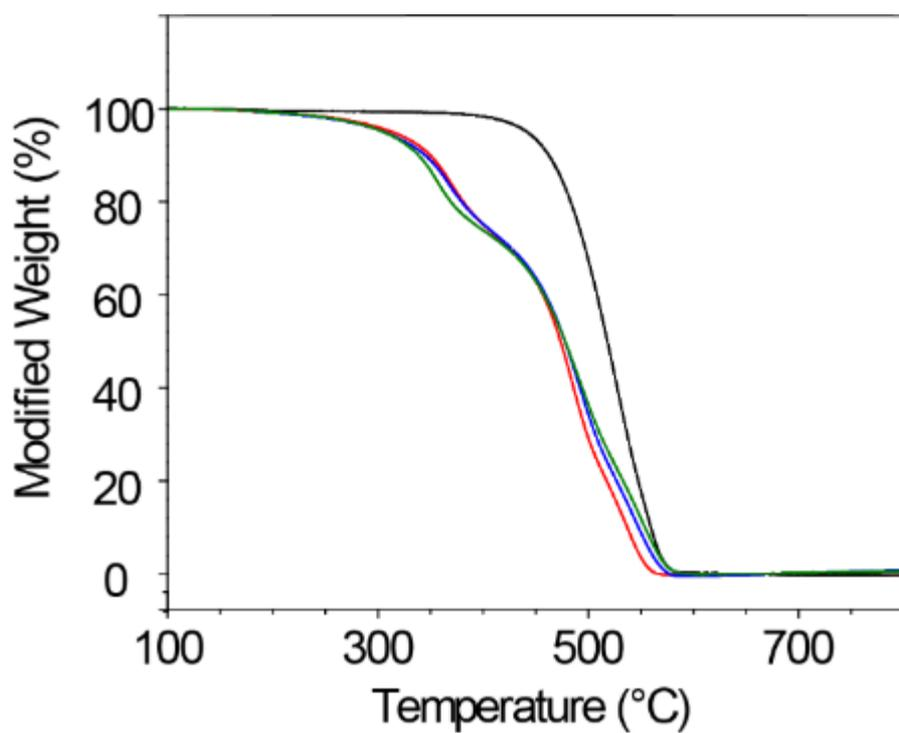
**Figure S8.** TGA analysis (air, 10°Cmin<sup>-1</sup>) of pristine (7,6)-enriched SWNTs (black) and the product formed by treatment with 1, 2 and 3 (blue)(red)(green) and the Grubbs second-generation catalyst in TCE at room temperature for 72 h.
