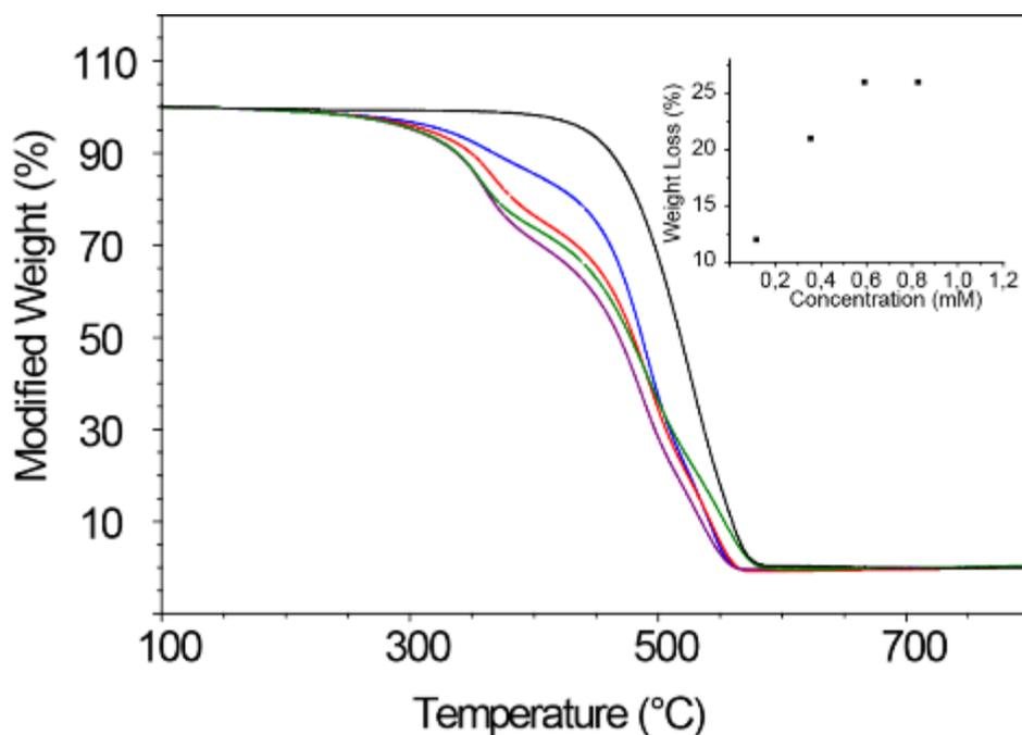
**Figure S6.** Variation in the degree of functionalization with the relative concentration of macrocycle **6** with respect to that of the SWNTs, as shown by TGA analysis (air,  $10 \text{ }^\circ\text{Cmin}^{-1}$ ): pristine (6,5)-enriched SWNTs (black), 0.12 mM (blue), 0.35 mM (red), 0.59 mM (green) and 0.83 mM (purple). Inset shows the relative weight loss versus the concentration.
