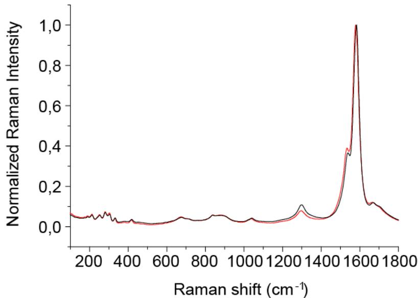
**Figure S2.** Raman spectra of (6,5)-enriched SWNTs (black) and the corresponding MINT(6,5) (red). The spectra is the average of three different measurements ( $\lambda_{exc} = 633$  nm)
