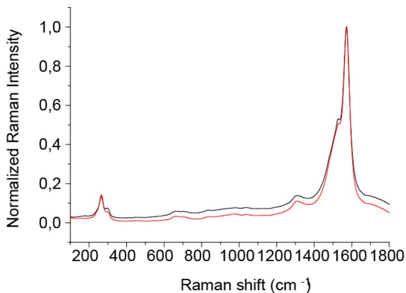
**Figure S3.** Raman spectra of (6,5)-enriched SWNTs (black) and the corresponding MINT(6,5) (red). The spectra is the average of three different measurements ( $\lambda_{exc} = 532 \text{ nm}$ )
