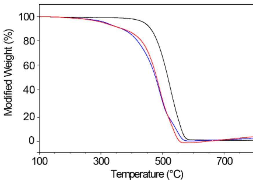
**Figure S7.** TGA analysis (air, 10 °C / min) of: 1 (black), linear receptor control experiment (red) and preformed macrocycle 6 control experiment (blue).
