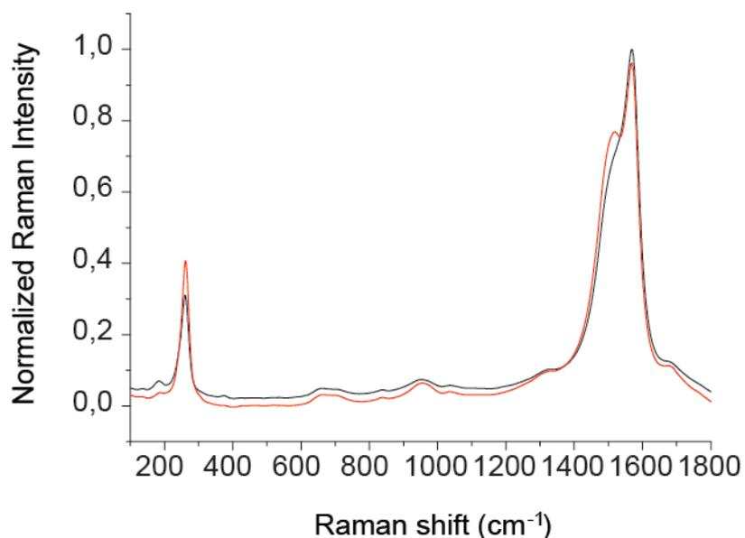
**Figure S5.** Raman spectra of (7,6)-enriched SWNTs (black) and the corresponding MINT(7,6) (red). The spectra is the average of three different measurements ( $\lambda_{exc} = 532 \text{ nm}$ ).
