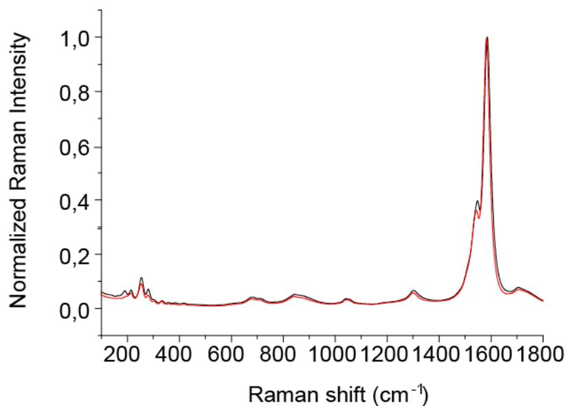
**Figure S4.** Raman spectra of (7,6)-enriched SWNTs (black) and the corresponding MINT(7,6) (red). The spectra is the average of three different measurements ( $\lambda_{exc} = 633 \text{ nm}$ )
