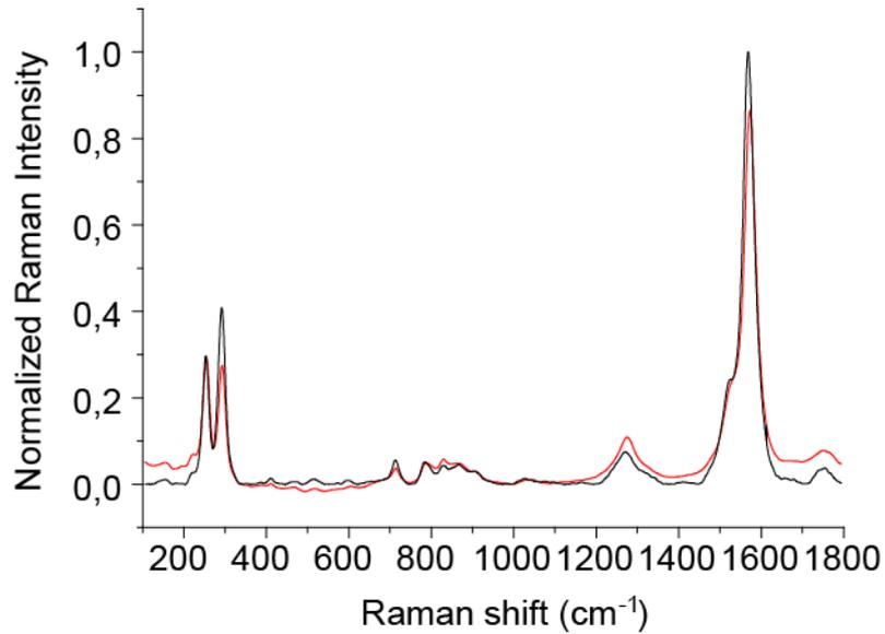
**Figure S1.** Raman spectra of (6,5)-enriched SWNTs (black) and the corresponding MINT(6,5) (red). The spectra is the average of three different measurements ( $\lambda_{exc} = 785$  nm)
