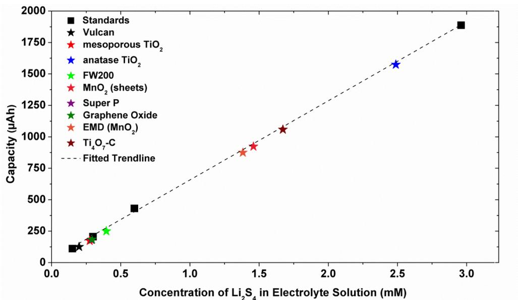
**Figure S1:** Calibration plot (squares) derived from the Coulombic capacity realized by oxidizing a known concentration of Li<sub>2</sub>S<sub>4</sub> in TEGDME to sulfur. Experimental points (stars) were mapped on the curve for a variety of different materials using the same method, providing a measure of their polysulfide adsorptivity.
