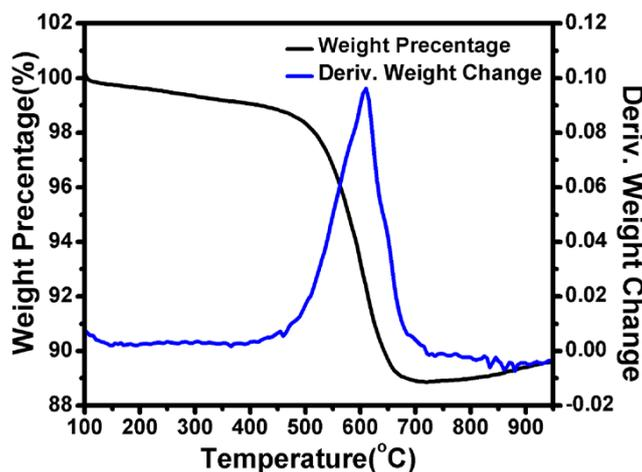
Fig.S1. TGA of precursor of  $\text{Na}_{2.65}\text{Ti}_{3.35}\text{Fe}_{0.65}\text{O}_9$
