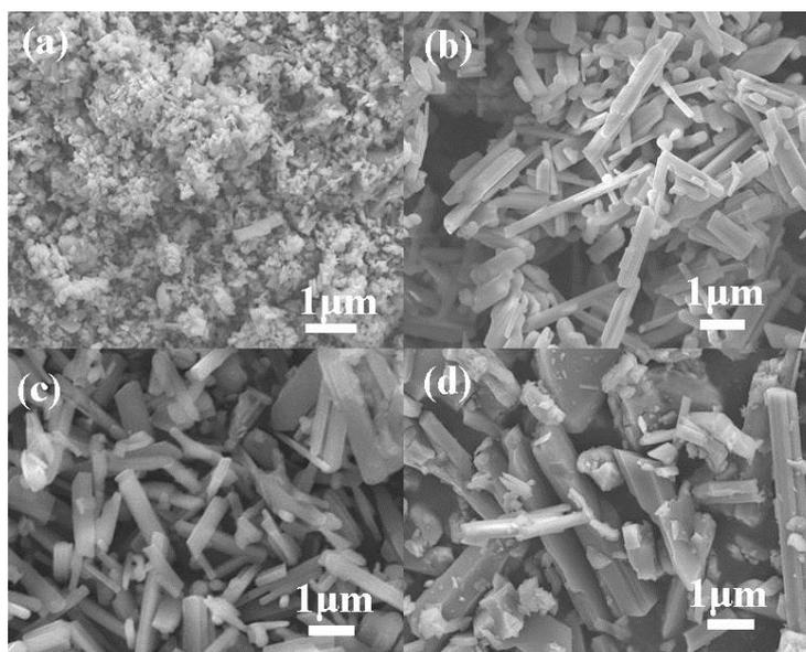
Fig. S3. SEM of the samples obtained at different temperature: (a) 750 °C, (b) 800 °C, (c) 850 °C and (d) 900 °C for 15h.
