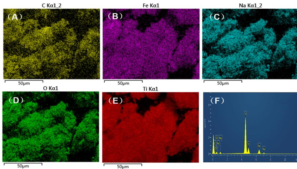
Fig.S4. EDS-element distribution mapping images of  $\text{Na}_{2.65}\text{Ti}_{3.35}\text{Fe}_{0.65}\text{O}_9/\text{C}$ .
