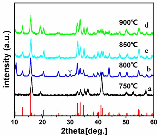
Fig.S2. XRD patterns of samples obtained at different temperature
