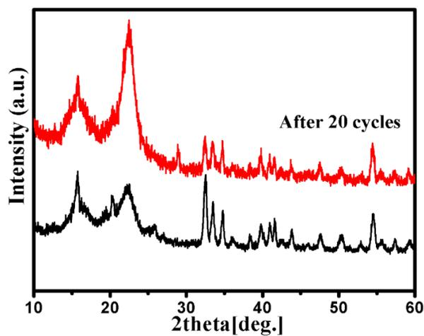
Fig.S5. Structural stability of  $\text{Na}_{2.65}\text{Ti}_{3.35}\text{Fe}_{0.65}\text{O}_9$  upon cycling
