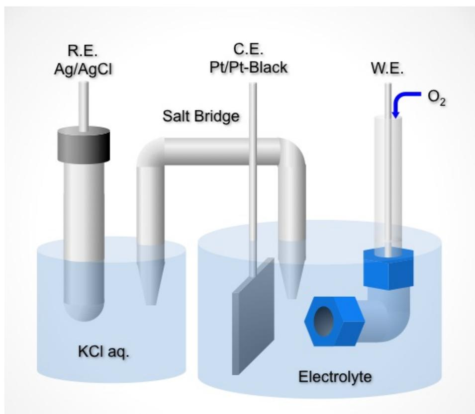
**Supplementary Fig. S1** Schematic representative of the three-electrode cell in the present work. The whole set up of the three-electrode cell was placed in a oxygen filled chamber. Since the Ag/AgCl reference electrode is not stable in alkaline solution, the cell was separated with a salt bridge filled with a gel of a KCl aqueous solution.
