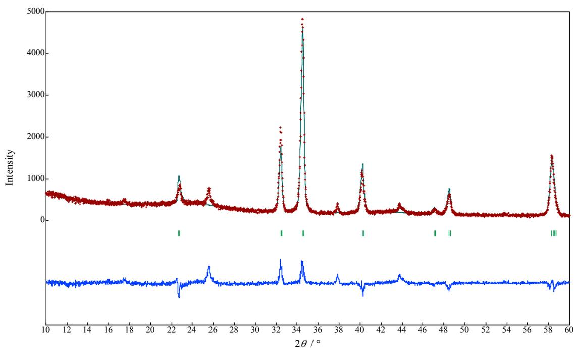
**Supplementary Fig. S2** A refined XRD pattern of discharged electrode. Fitting result of the measured diffraction pattern (brown) and the simulated pattern (green) was good. The diffraction peak at 25 ° is assigned to graphite. And the peaks at 38 ° and 44 ° were corresponding to the air-free aluminum sample holder.
