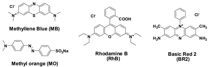
Fig. S8 The structures of dyes, MB, MO, RhB, and BR2.
