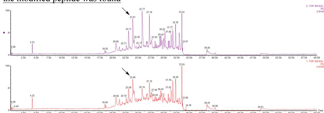
**B) MS spectrum of peptide: 27–VIESGPHCANTEIIVK–42** obtained after tryptic digestion of the purified product and containing the modification at histidine 33 (B = [Ru(CO)<sub>2</sub>]<sup>2+</sup>). *m/z* value of the triply charged peptide = 622.93
