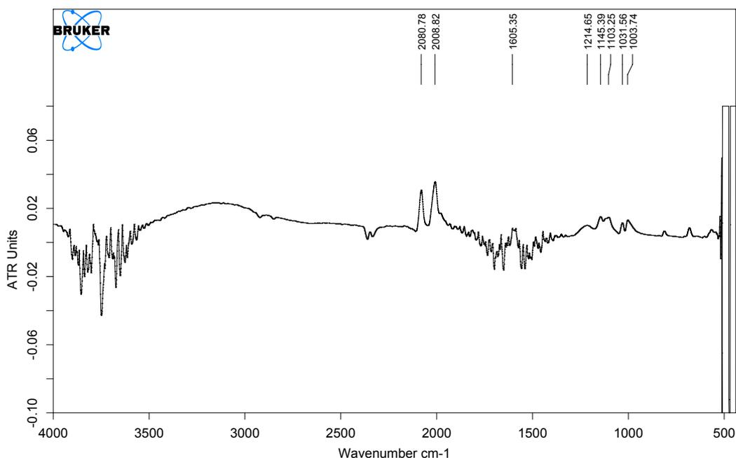
**Fig. S2** FTIR (ATR) spectrum of *cis*-[Ru(CO)<sub>2</sub>(H<sub>2</sub>O)<sub>4</sub>](OTs)<sub>2</sub>.
