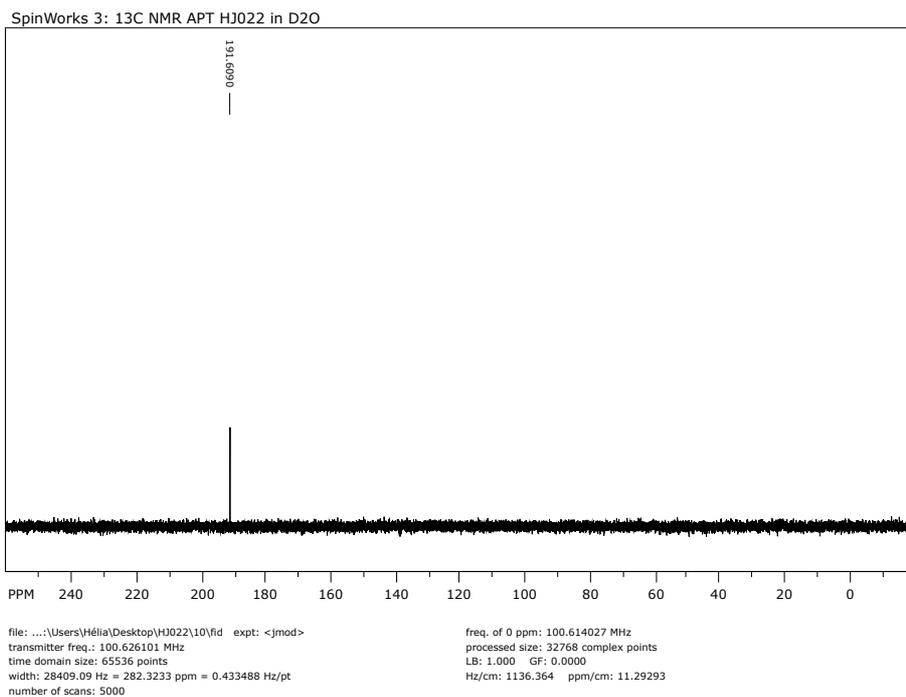
**Fig. S3**  $^{13}\text{C}$  NMR spectrum (D<sub>2</sub>O;  $\delta$  ppm) of *cis*-[Ru(CO)<sub>2</sub>(H<sub>2</sub>O)<sub>4</sub>](OTs)<sub>2</sub>.
