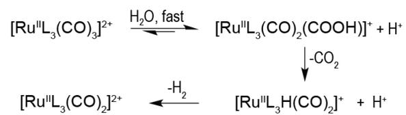
**Fig. S1** Proposed water-gas shift reaction for the generation of the  $[\text{Ru}(\text{CO})_2]^{2+}$  fragment from CORM-3.
