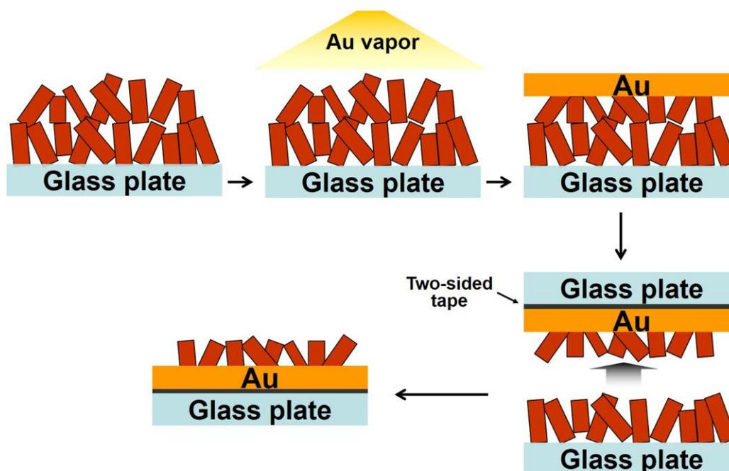
**Figure S2.** Fabrication of LTC/Au electrodes by PT method.
