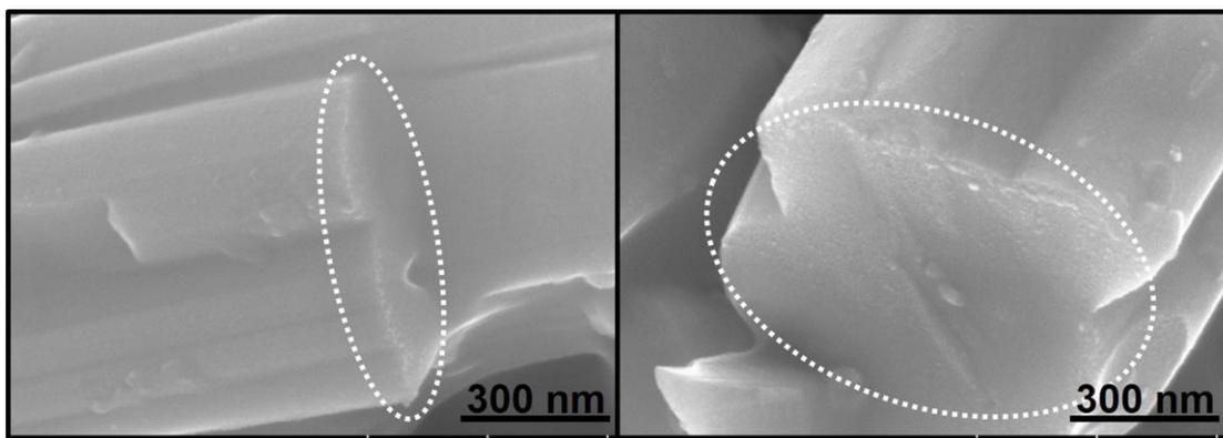
**Figure S5.** SEM images of Pt/Sc-LTC/Au electrodes. The Pt was deposited in a solution containing  $\text{Na}_2\text{SO}_4$  (0.1 M) and  $\text{H}_2\text{PtCl}_6$  ( $10 \times 10^{-6}$  M).
