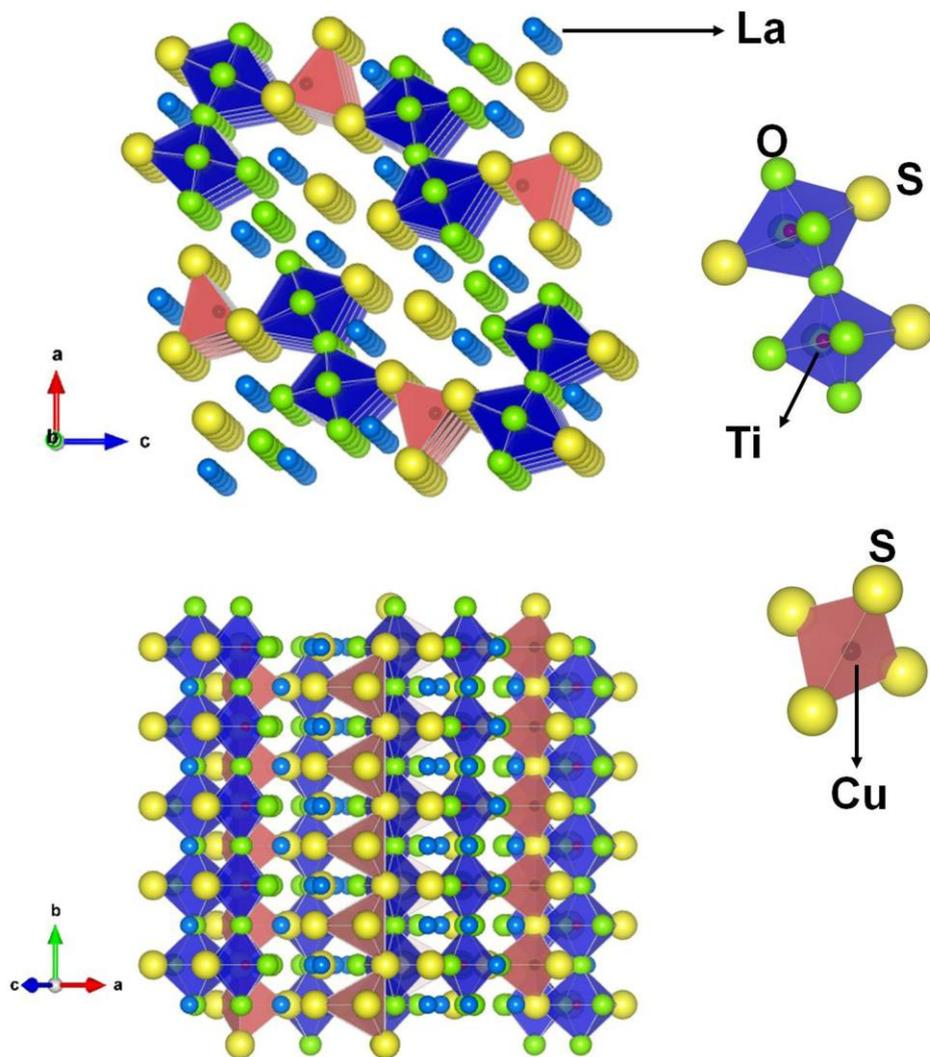
**Figure S7.** Crystal structure of  $\text{La}_5\text{Ti}_2\text{CuS}_5\text{O}_7$  viewed along  $b$  and  $c$  axes (depicted using Vesta<sup>4</sup>).
