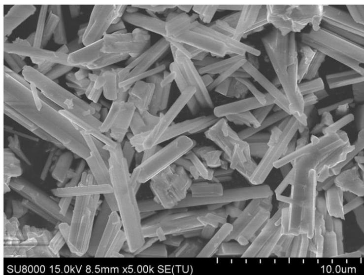
**Figure S1.** SEM image of Sc-LTC powder.
