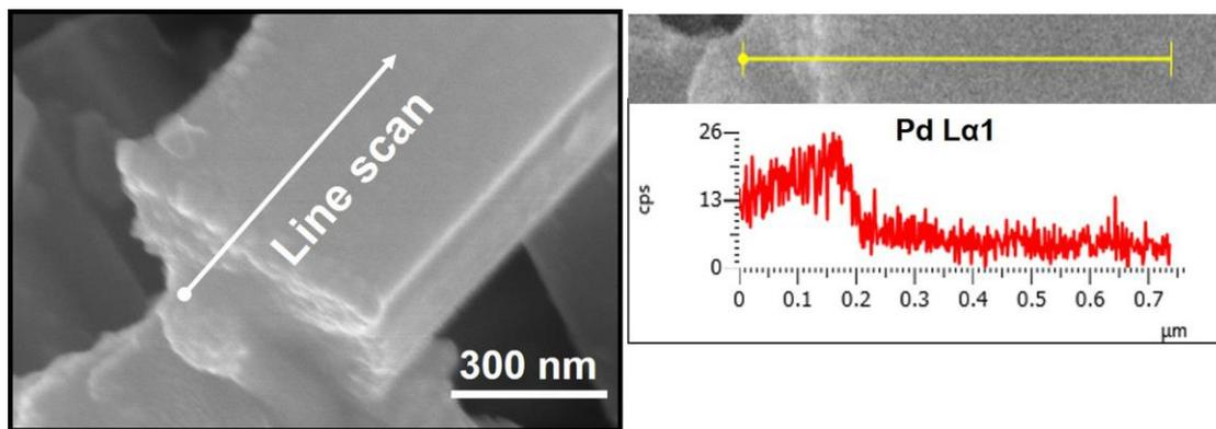
**Figure S6.** SEM and EDX analysis of Pd/Sc-LTC/Au electrodes. The Pd was deposited in a solution containing  $\text{Na}_2\text{SO}_4$  (0.1 M),  $\text{K}_2\text{C}_2\text{O}_4$  (0.1 M), and  $(\text{NH}_4)_2\text{PdCl}_4$  ( $15 \times 10^{-6}$  M).
