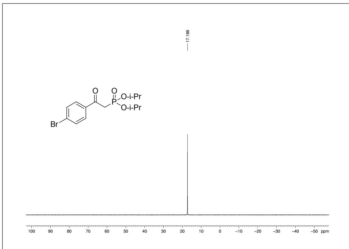
**Fig. 55**  $^{31}\text{P}$  NMR spectrum of compound **3n**
