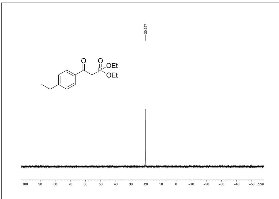
**Fig. 35**  $^{31}\text{P}$  NMR spectrum of compound 3i
