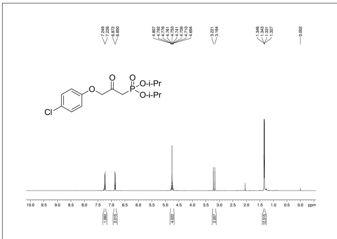
**Fig.89**  $^1\text{H}$  NMR spectrum of compound 3w
