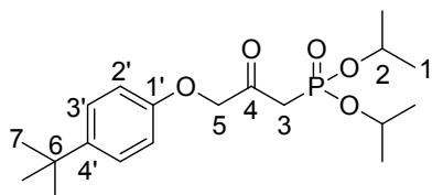
Yellow oil,  $^1\text{H}$  NMR ( $\text{CDCl}_3$ , 400 MHz)  $\delta$ : 7.30 (d, 2H, 3'-H,  $J$ = 8.8 Hz), 6.85 (d, 2H, 2'-H,  $J$ = 8.8 Hz), 4.82-4.74 (m, 2H, 2-H), 4.72 (s, 2H, 5-H), 3.22 (d, 2H, 3-H,  $J$ = 22.8 Hz), 1.34 (d, 12H, 1-H,  $J$ = 6.0 Hz), 1.30 (s, 9H, 7-H);  $^{13}\text{C}$  NMR ( $\text{CDCl}_3$ , 100 MHz);  $\delta$ : 198.7 (d, C-4,  $J_{\text{P-C}}$ = 6.5 Hz),
