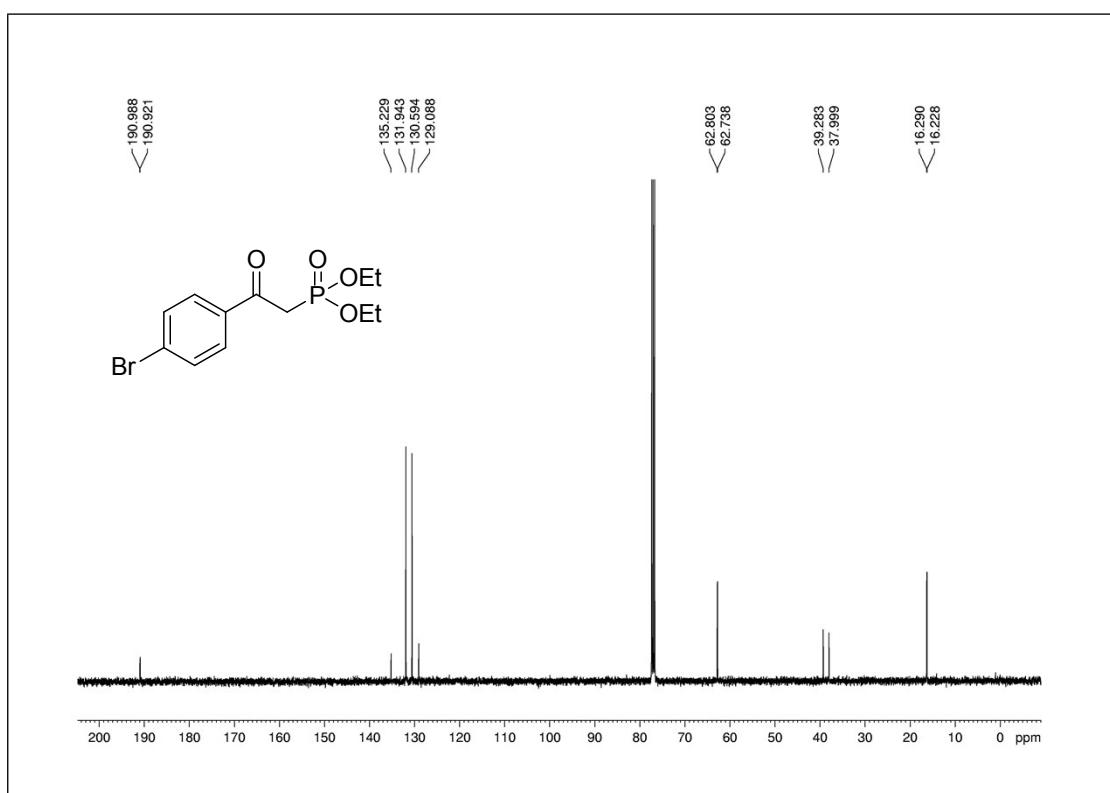
**Fig. 50**  $^{13}\text{C}$  NMR spectrum of compound **3m**
