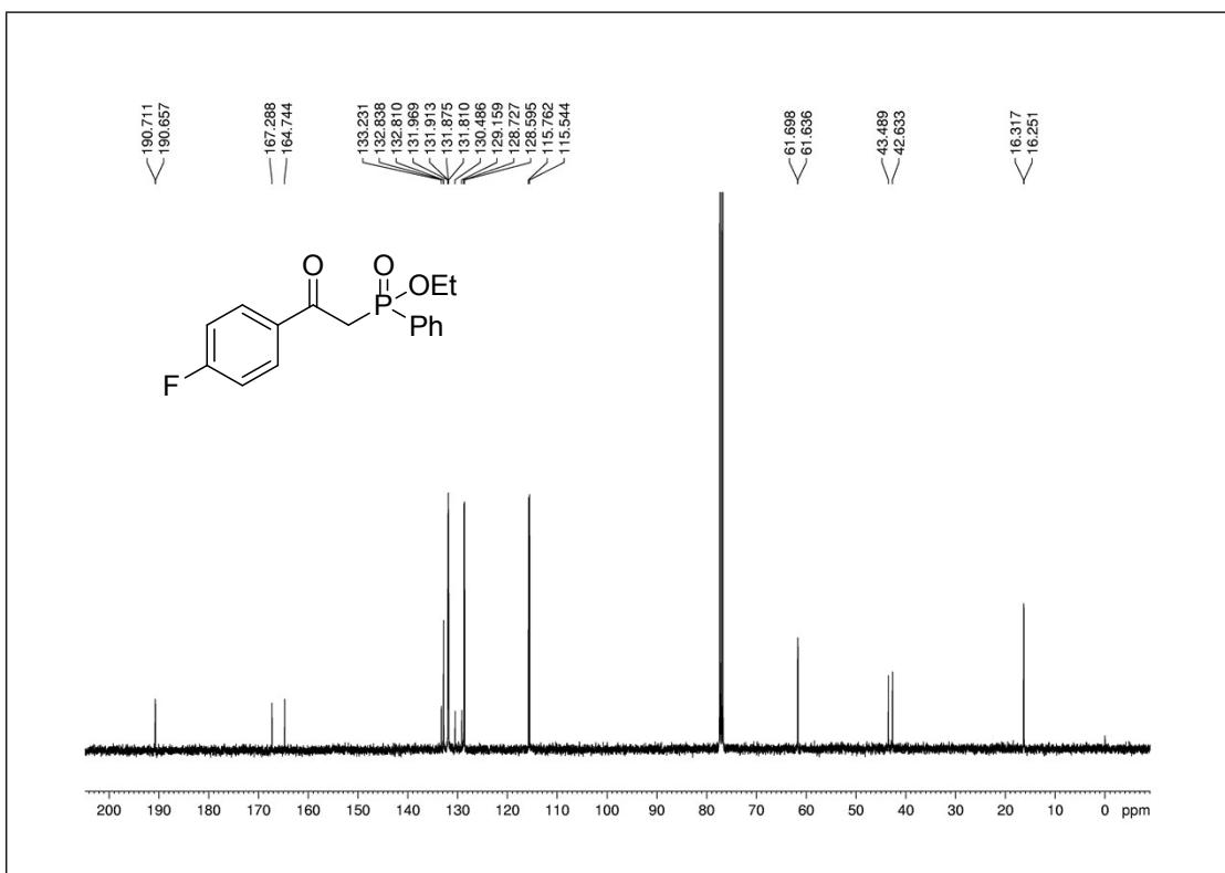
**Fig. 66**  $^{13}\text{C}$  NMR spectrum of compound 3q
