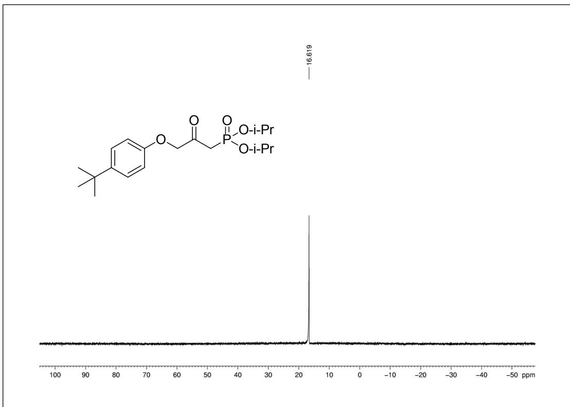
**Fig. 87**  $^{31}\text{P}$  NMR spectrum of compound **3v**
