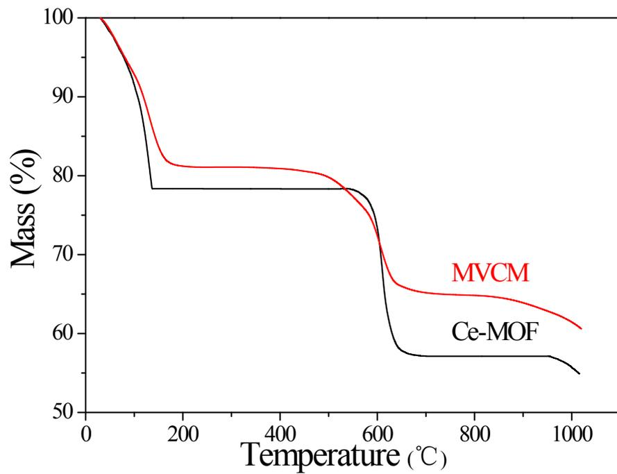
Fig. S4 TGA curves of MVCM and Ce-MOF.
