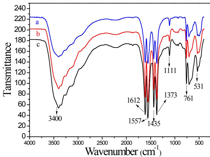
Fig. S3 FT-IR spectrum of MVC (a) after, (b) before catalytic reaction and (c) Ce-MOF.
