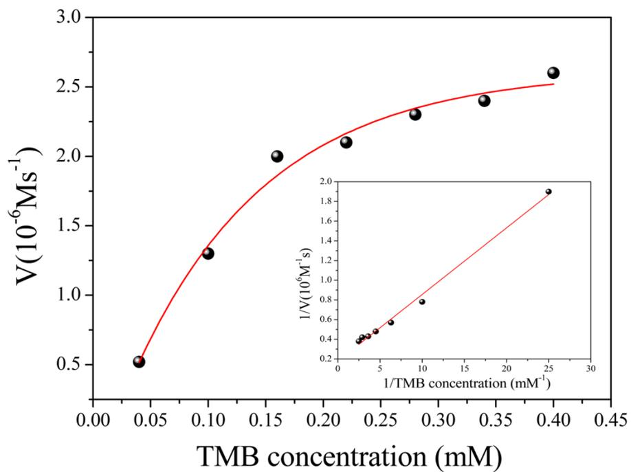
Fig. S10 Steady-state kinetic assays of the MVCM. Insets: Lineweaver–Burk plots of the double reciprocal of the Michaelis–Menten equation. TMB was used as substrate.
