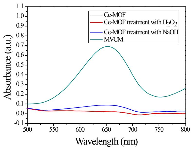
Fig. S6 Catalytic activity of different oxidase mimetic.
