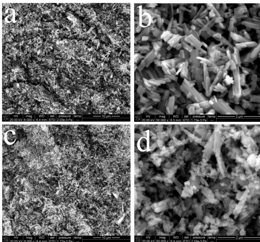
Fig. S2 SEM images of MVCM (a, b) and Ce-MOF (c, d)
