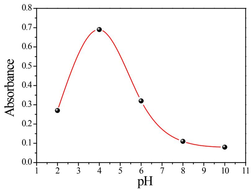
Fig. S9 The catalytic activity of MVCM at different pH values of solution.
