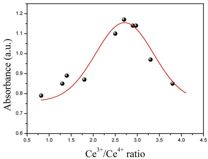
Fig. S8 The catalytic activities of MVCM at different Ce<sup>3+</sup>/Ce<sup>4+</sup> ratios.
