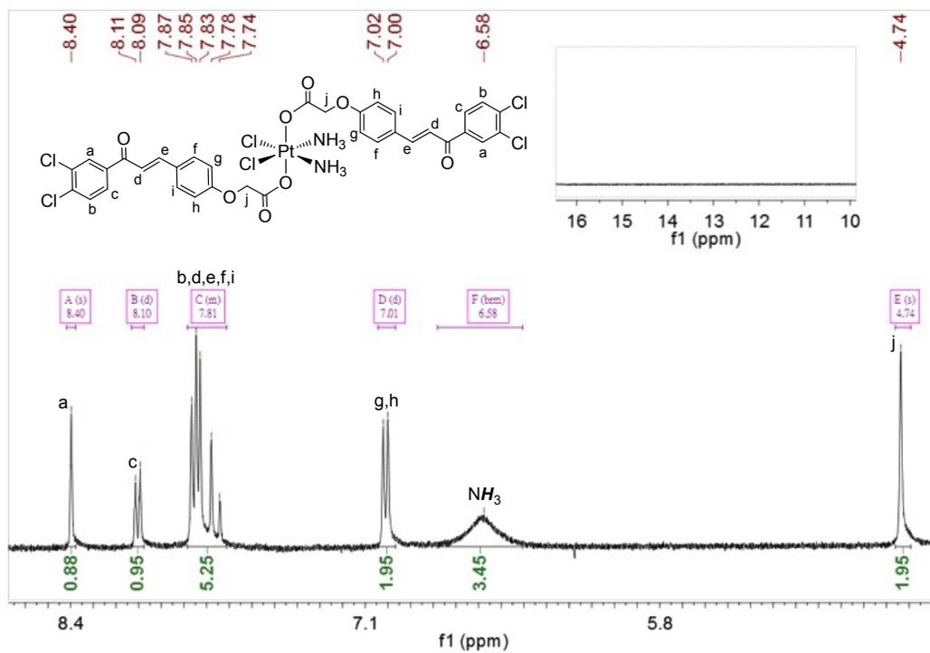
Figure S2  $^1\text{H}$  NMR spectrum of chalcoplatin (4) in  $\text{DMSO-}d_6$ .
