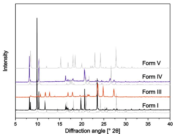
**Figure S6** Experimental PXRD patterns of three crystal forms of PCB and the calculated patterns from the crystal structures (grey scale).
