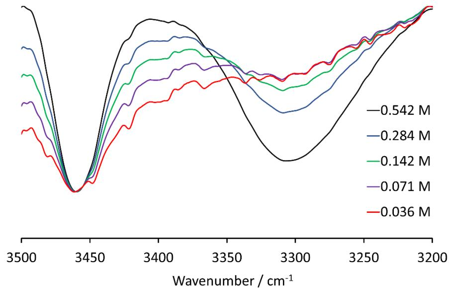
**Figure S4** FTIR spectra of the titration of OCB in chloroform solution. The spectra have been normalised at the maximum intensity band at *ca.* 3460 cm<sup>-1</sup>, which is assigned as the monomer band. The broader peak at *ca.* 3300 cm<sup>-1</sup> is assigned to the dimer.
