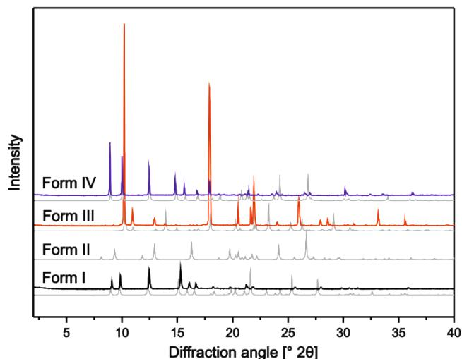
**Figure S3** Experimental PXRD patterns of three crystal forms of OCB and the calculated patterns from the crystal structures of all four crystal forms (grey scale).
