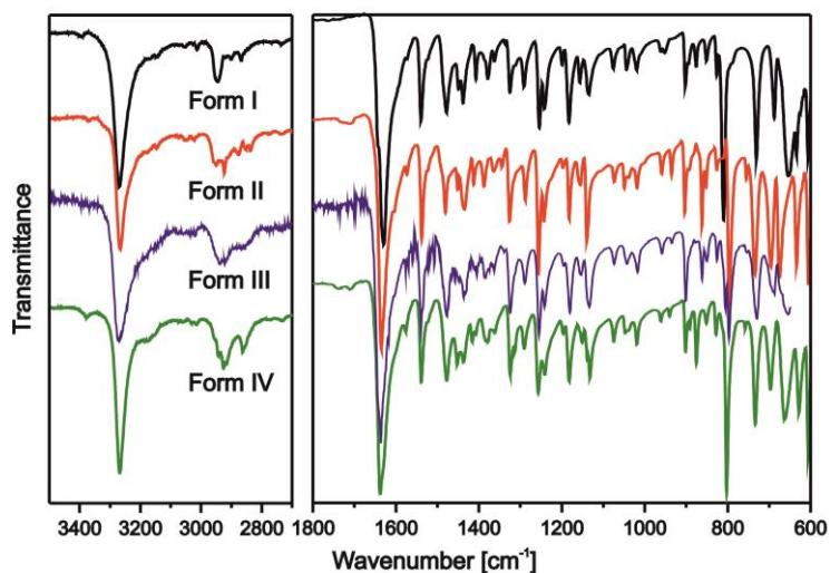
**Figure S5** FTIR spectra of the four crystal forms of PCB.
