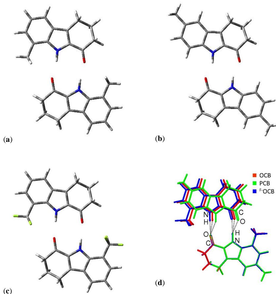
**Figure S7** DFT optimised structures of the dimers of (a) OCB, (b) PCB and (c) <sup>F</sup>OCB at the B3LYP/6-311+G(d) level of theory with GD3BJ dispersion correction. (d) Overlap of the lower molecules of the dimers to illustrate the difference in offset.
