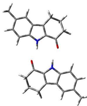
**Figure S1** Dimer motif found in the carbazolones with lateral offset of the centro-symmetric dimer. The hydrogen bond acceptor group is shifted towards the indolyl moiety, while the synthon stays overall planar.
