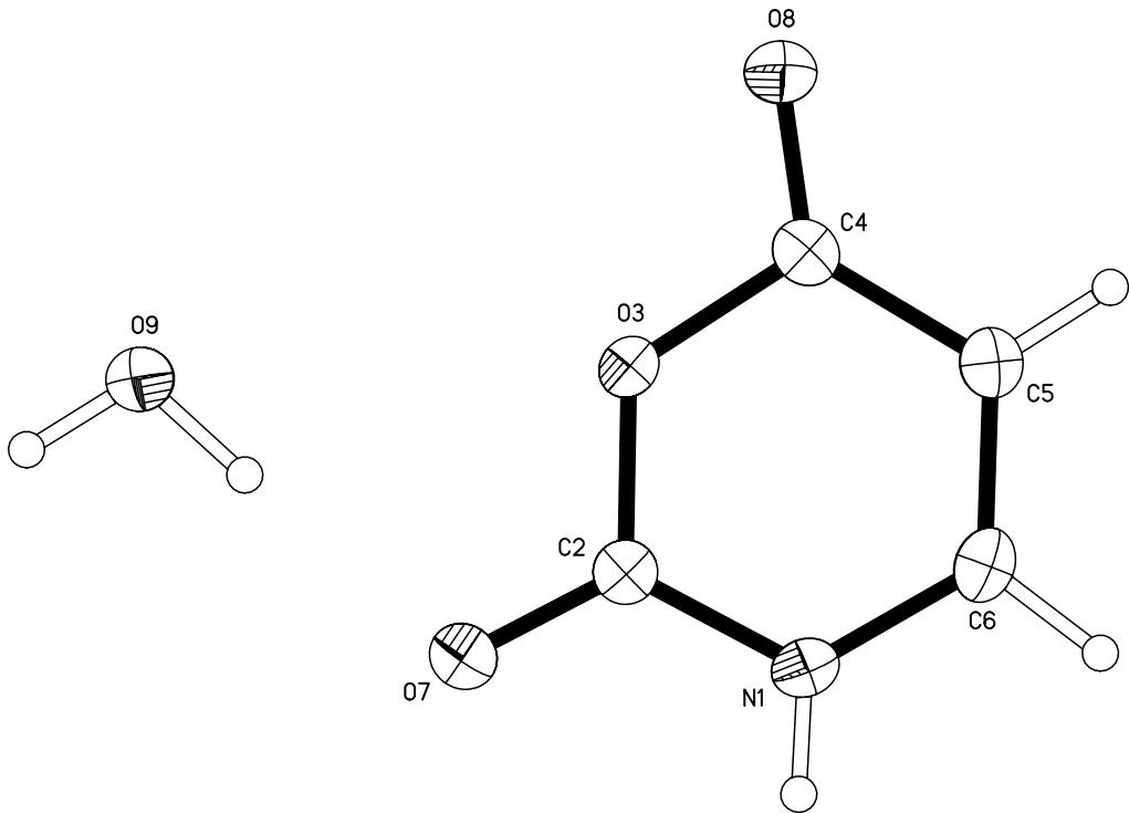
A view of a molecule of 3-oxauracil and a molecule of water from the crystal structure showing the numbering scheme employed. Anisotropic atomic displacement ellipsoids for the non-hydrogen atoms are shown at the 50% probability level. Hydrogen atoms are displayed with an arbitrarily small radius.
