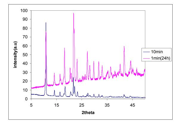
S1 Comparison of XRPD patterns from samples of material 1 prepared by 1 and 10 minutes grinding. The 1 minute sample had been left to stand for 24h before obtaining the XRPD pattern.
