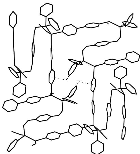
**Fig. S3** Showing C-H... $\pi$  weak interactions between phenyl rings attached on phosphorus atoms and uninvolved-in- $\pi$ -stacking pyridyl rings in the Z-shape subunit, Ring-centroids distance: 4.454 $\text{\AA}$ , dihedral angle: 25.7°, and H... $\pi$ <sub>centroid</sub>: 3.057 $\text{\AA}$ .
