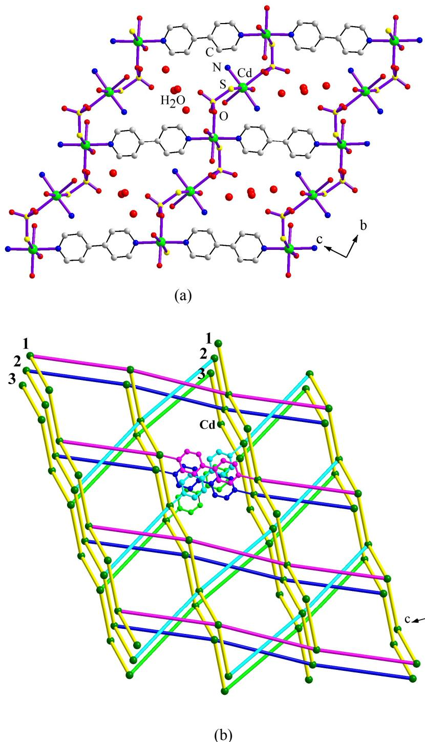
Fig. S9: (a) Two-dimensional layer view of cadmium-thiosulfate with *bpy*, containing lattice water of compound I. (b) Three-dimensional interpenetrating structure of compound I. Purple, blue, cyan and green lines show the different layer of *bpy*. Yellow line corresponds to the thiosulfate chain.
