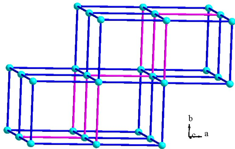
Fig. S15: (b) Schematic diagram of **pcu** net. Purple bonds represent the bonds that are absent in **III**.
