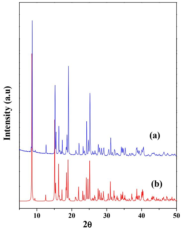
Fig. S1: Powder XRD ( $\text{CuK}\alpha$ ) pattern of **I**, (a) experimental and (b) simulated
