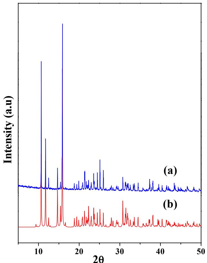
Fig. S2: Powder XRD ( $\text{CuK}\alpha$ ) pattern of **II**, (a) experimental and (b) simulated
