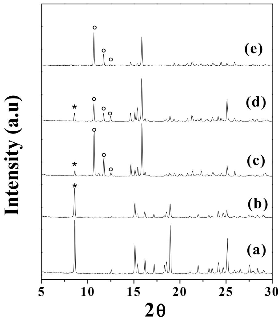
Fig. S17: Transformation of **I** to **II** by reaction of **I** and *bpy* (1: 0.50) at 45 °C at different times (a) pure **I**, (b) after 4 hrs, (c) after 8 hrs, (d) after 12 hrs and (e) after 20 hrs (pure **II**) The symbol \* shows the peak of **I** and the symbol O represents **II**.
