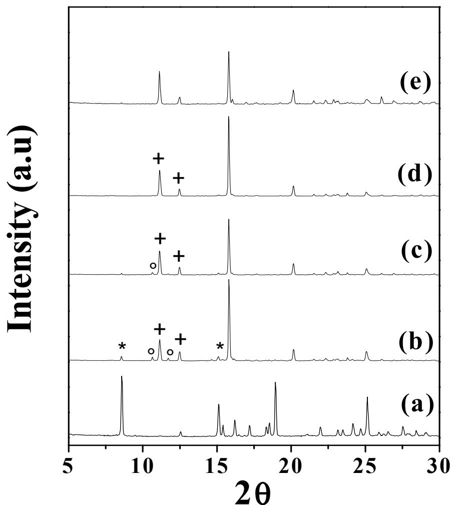
Fig. S18: Transformation of **I** to **III** by the reaction of **I** and *bpy* (1: 0.25) at  $60^{\circ}\text{C}$  in different times (a) pure **I**, (b) after 4 hrs, (c) after 8 hrs, (d) after 12 hrs and (e) after 20 hrs (pure **III**). The symbol \* represent the peaks of **I**, the symbol o represents the peaks of **II** and the symbol + represents the peaks of **III**.
