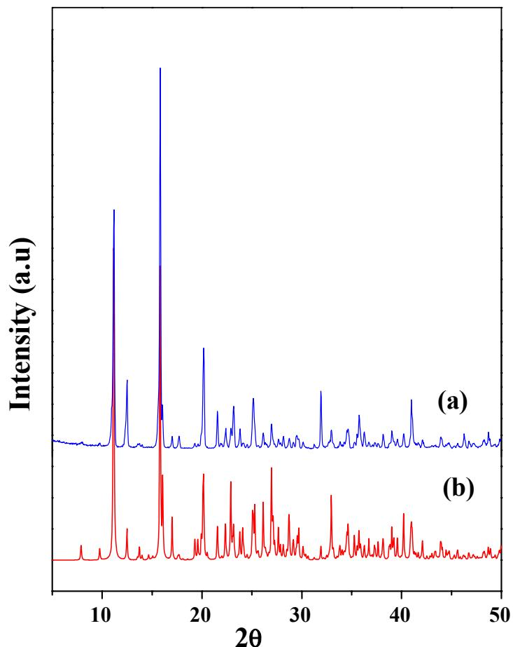
Fig. S3: Powder XRD ( $\text{CuK}\alpha$ ) pattern of **III**, (a) experimental and (b) simulated
