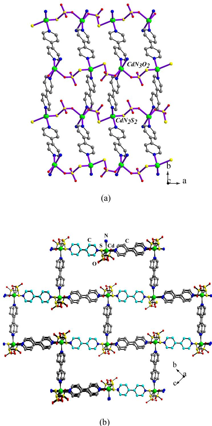
Fig. S12: (a) Two-dimensional layer view of compound **III** with metal-thiosulfate and *bpy*. One coordination of trigonal bipyramidal cadmium with *bpy* is missing here which forms the three-dimensional structure. (b) The three-dimensional architecture of compound **III**.
