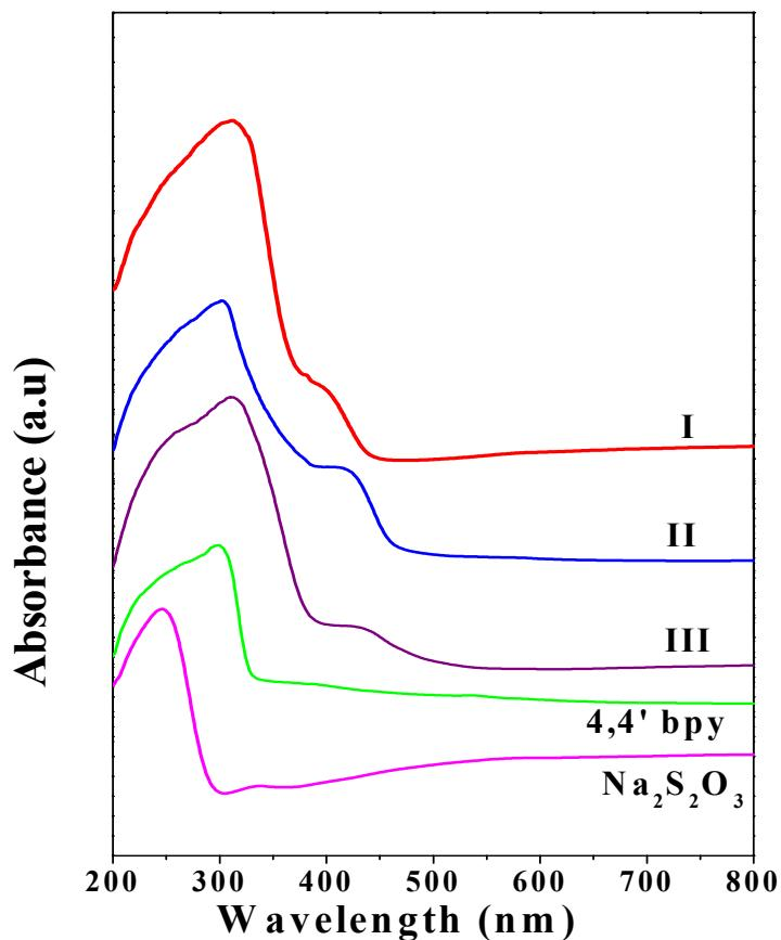
Fig. S6: Solid state absorbance spectra (UV-visible) of compound I-III, 4,4'-bipyridine and Na<sub>2</sub>S<sub>2</sub>O<sub>3</sub>.
