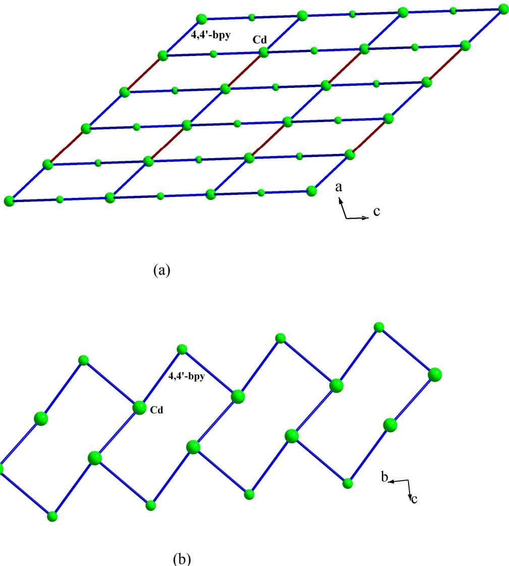
Fig. S10: (a) Two-dimensional layer of Cd and bpy in Compound **II**. (b) One-dimensional edge-sharing rectangular box in compound **III**. Linear lines are *bpy* unit and green spheres are Cd.
