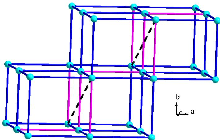
Fig. S14: (b) Schematic diagram of **pcu** net. Purple bonds show the bonds that are absent in **II** and black dotted lines are extra bonds in **II**.
